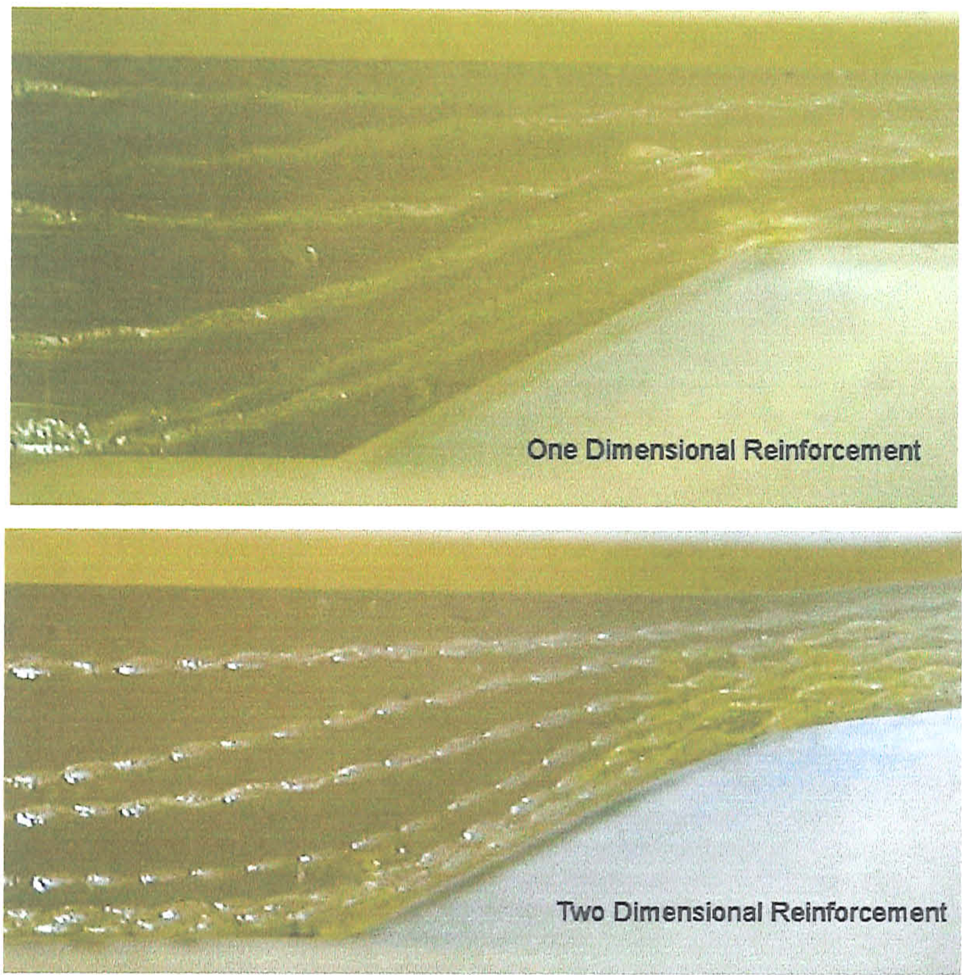
Fig 8.3.2.1-2 The fibre alignments of the wedge-shaped test specimens in Chapter 5.
