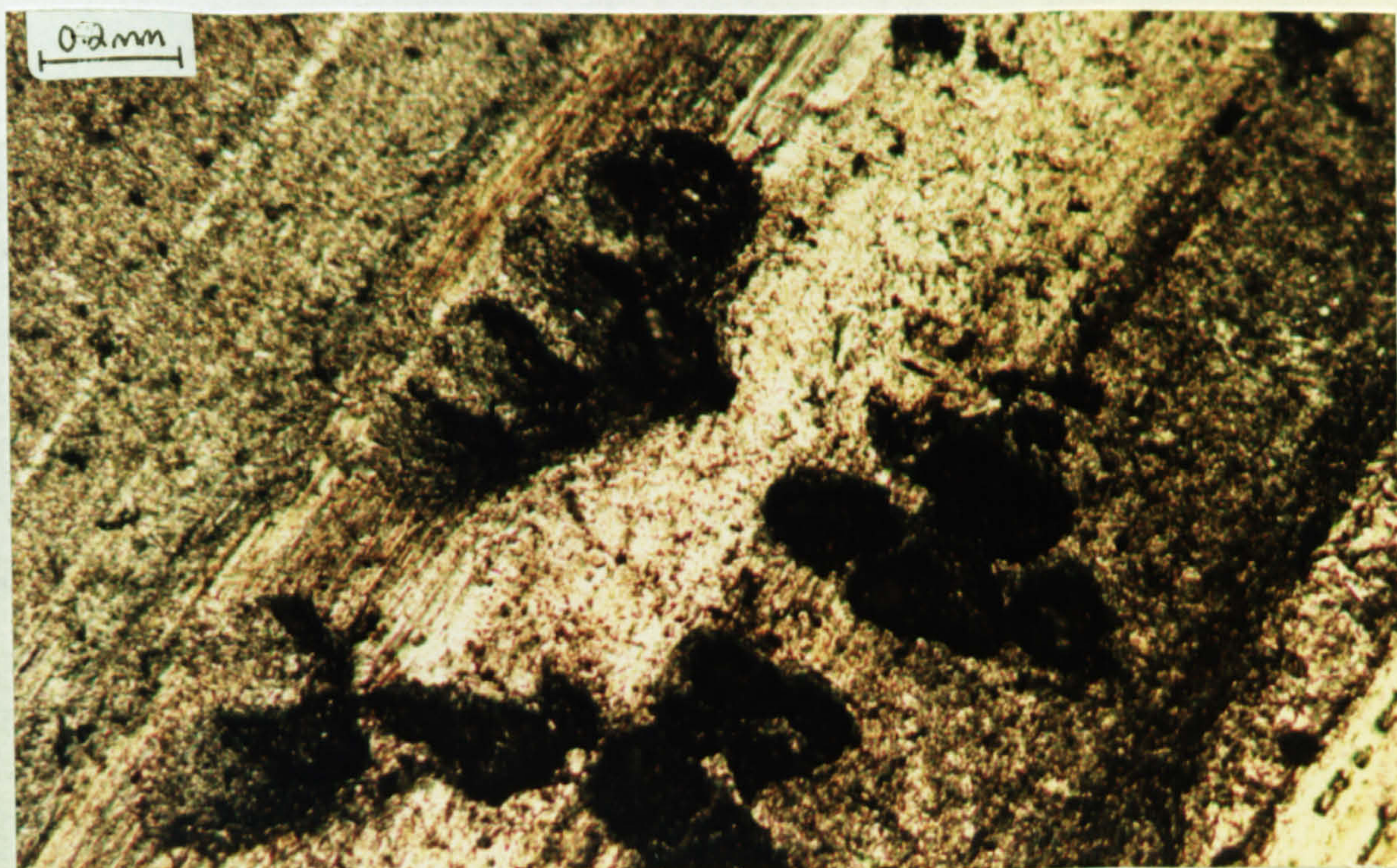
Fig. 3.1(a) Pitting on the outer surface of a Stellite 6 wear ring after exposure to seawater at 90°C and approximately four times the concentration of normal seawater and (b) closer view of pitting on the outer surface of the Stellite 6 wear ring
