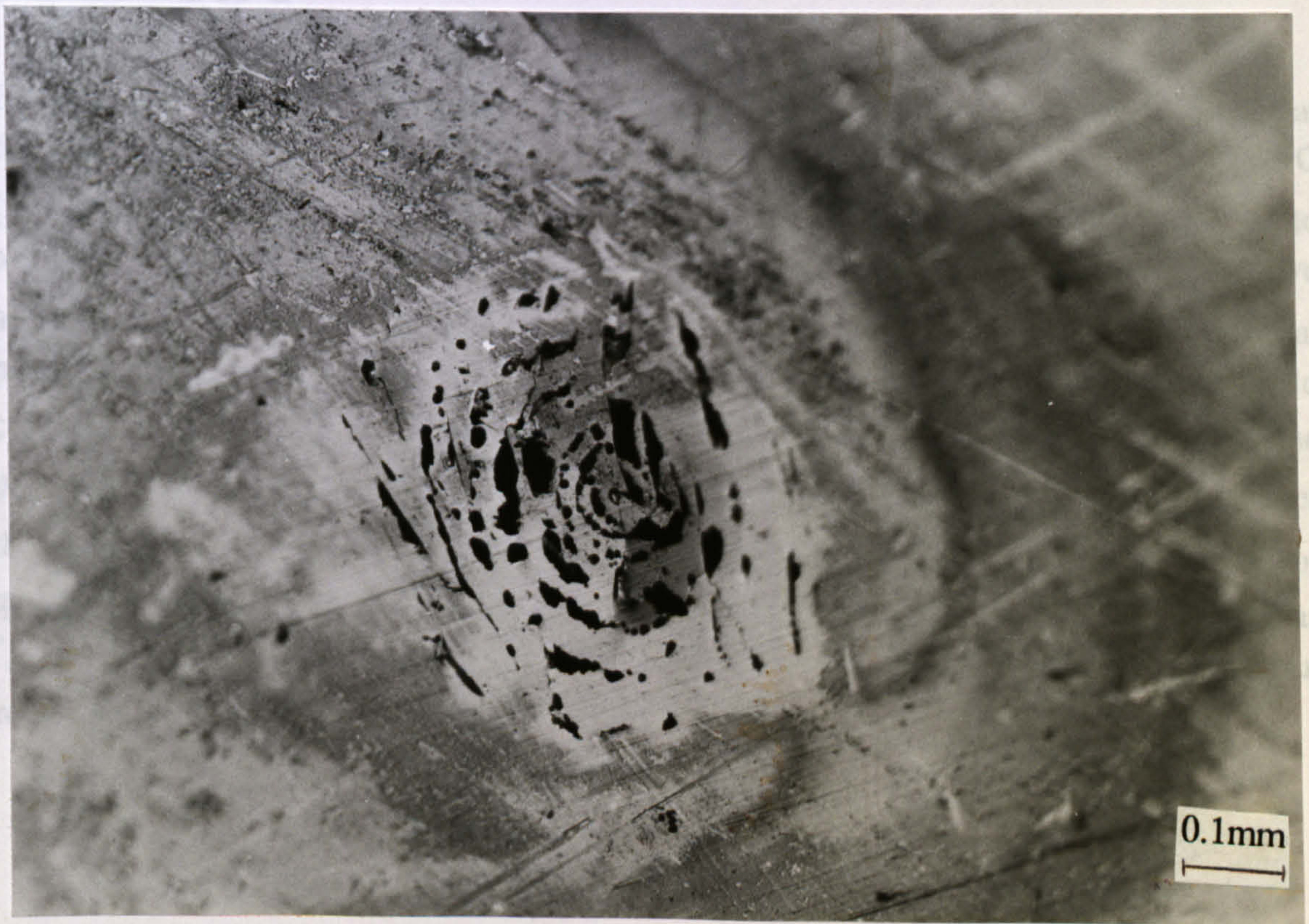
Fig. 3.14. Pitting attack on UNS S32760 after anodic polarisation at 90°C
