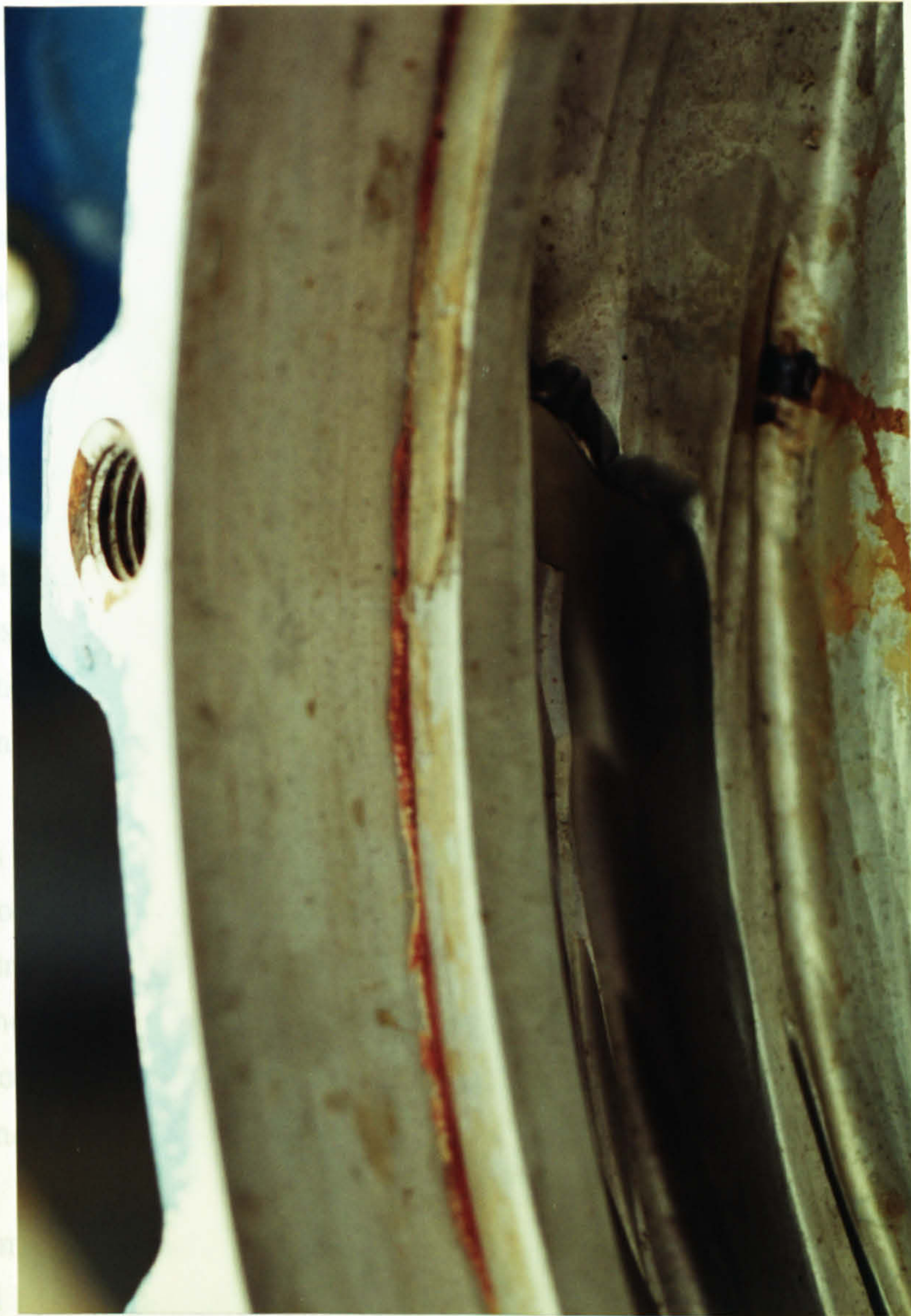
(b) Fig. 5.6a and b. Erosion on the UNS S31603 pump casing after 240-300 hours in periodic service
