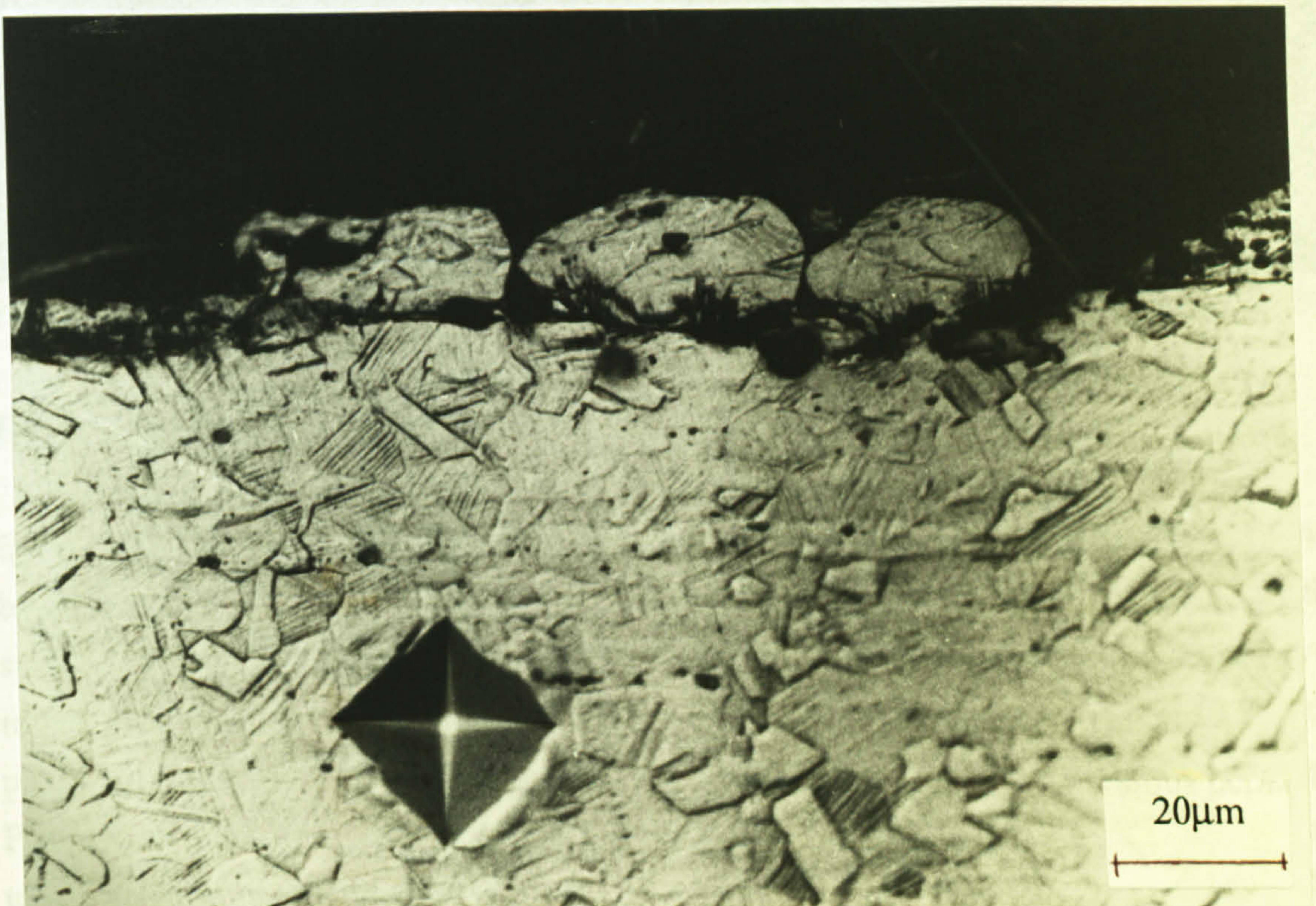
Fig. 5.50. Fragments of material detaching from the surface of an eroded sample of UNS S31603
