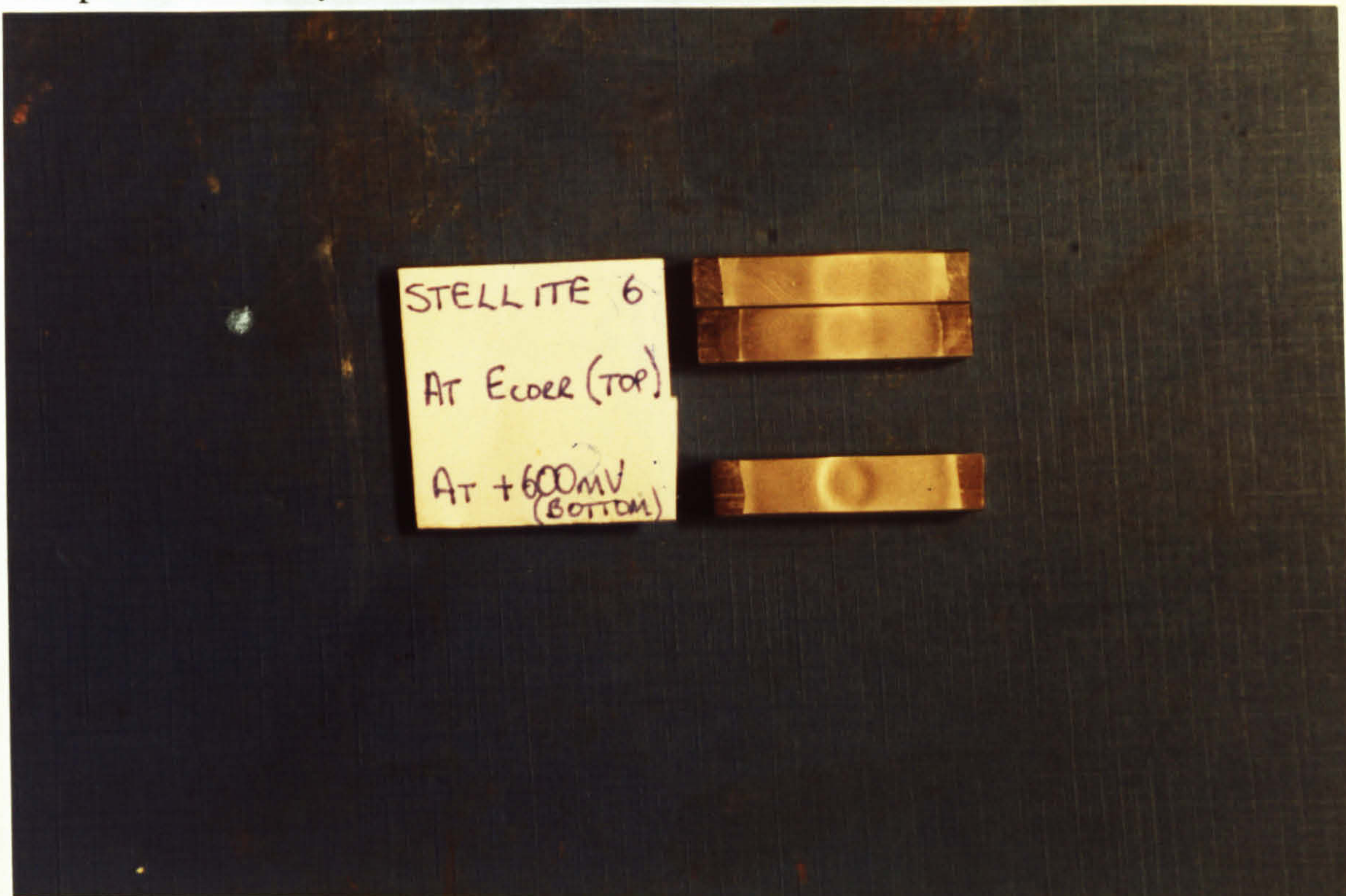
Fig. 5.51. Deeper wear scar on specimen under potentiostatic control at 600mV (SCE)
