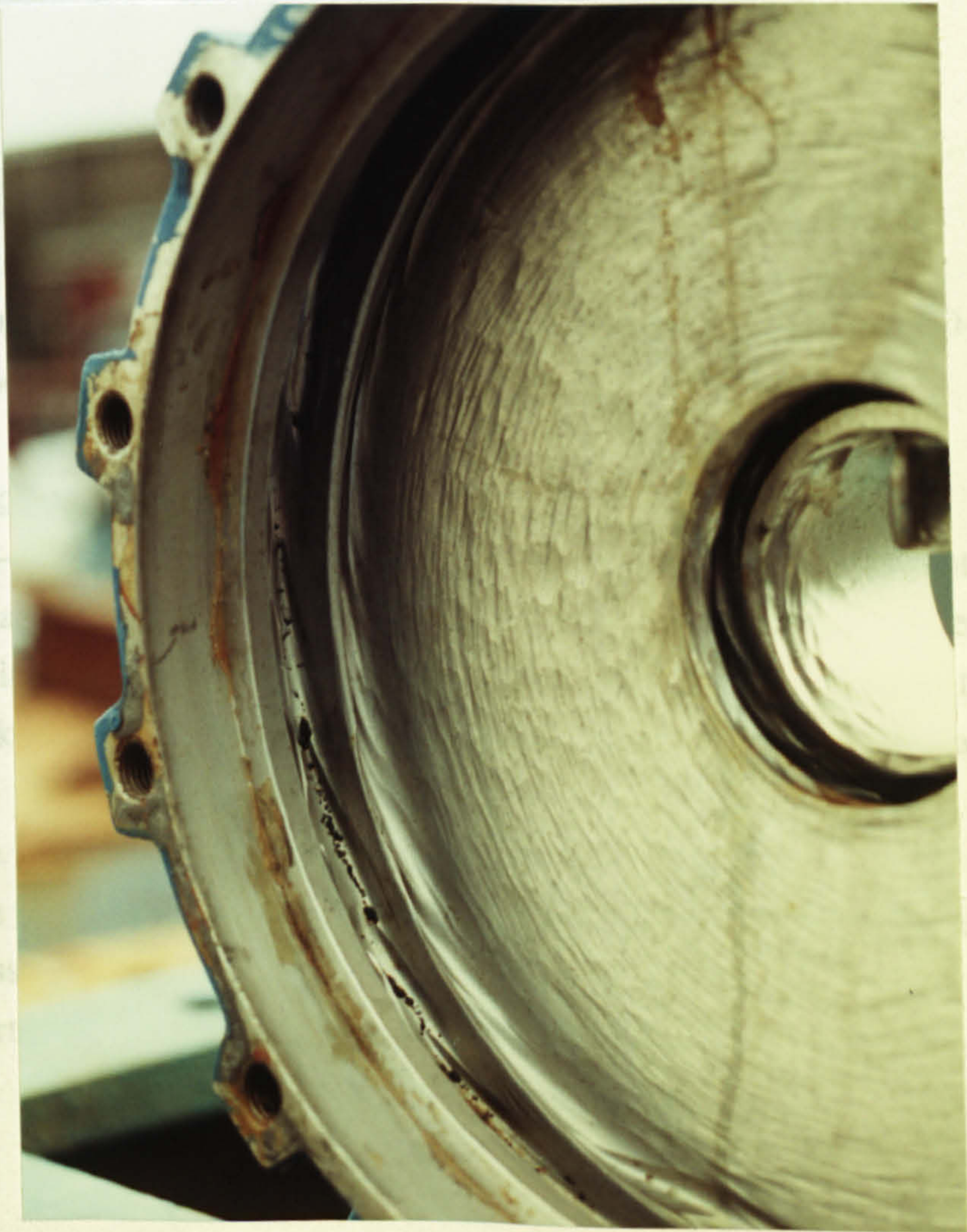
Fig. 5.5. Deterioration of a cast iron valve from the test rig after 240-300 hours service
