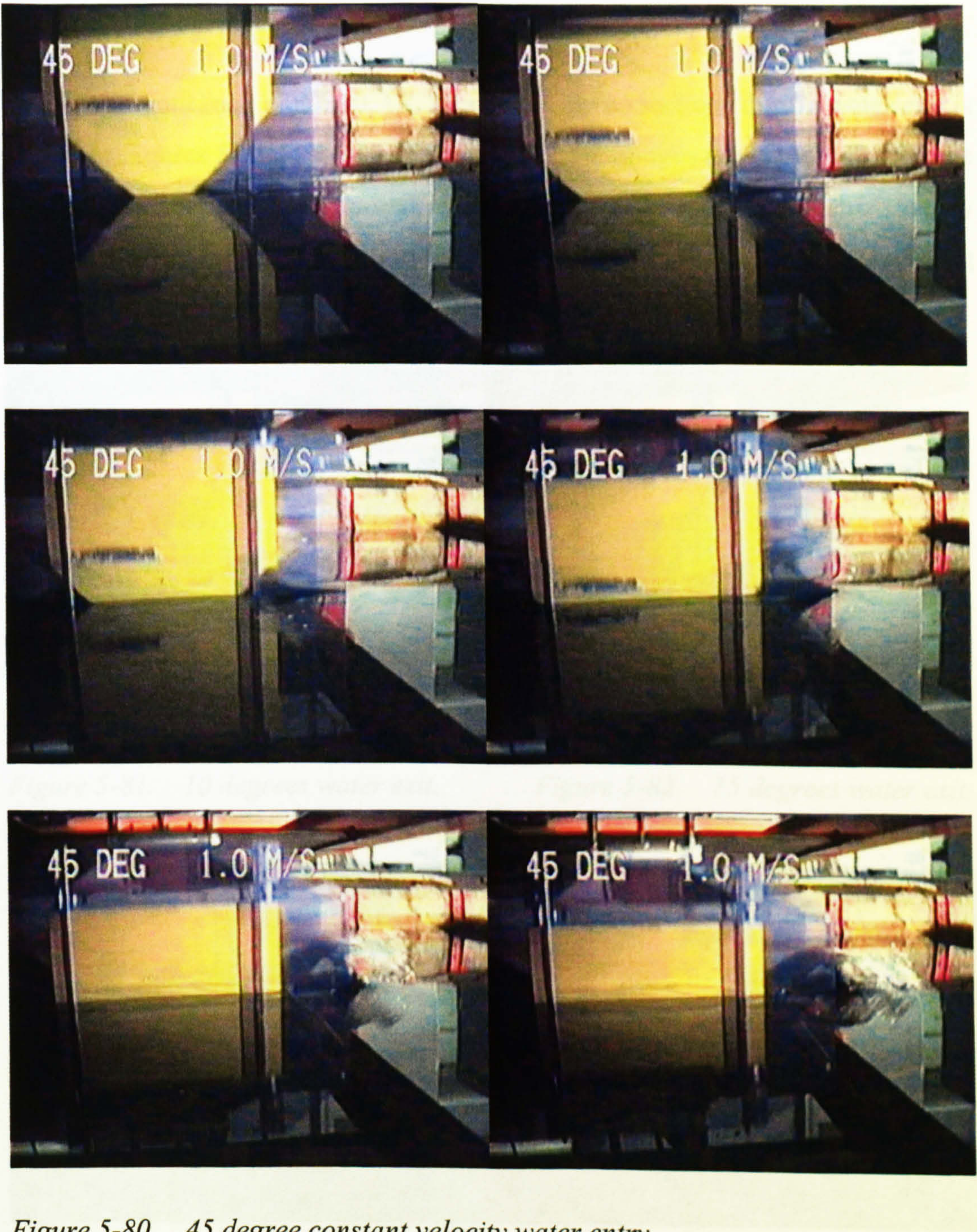
Figure 5-80. 45 degree constant velocity water entry.
