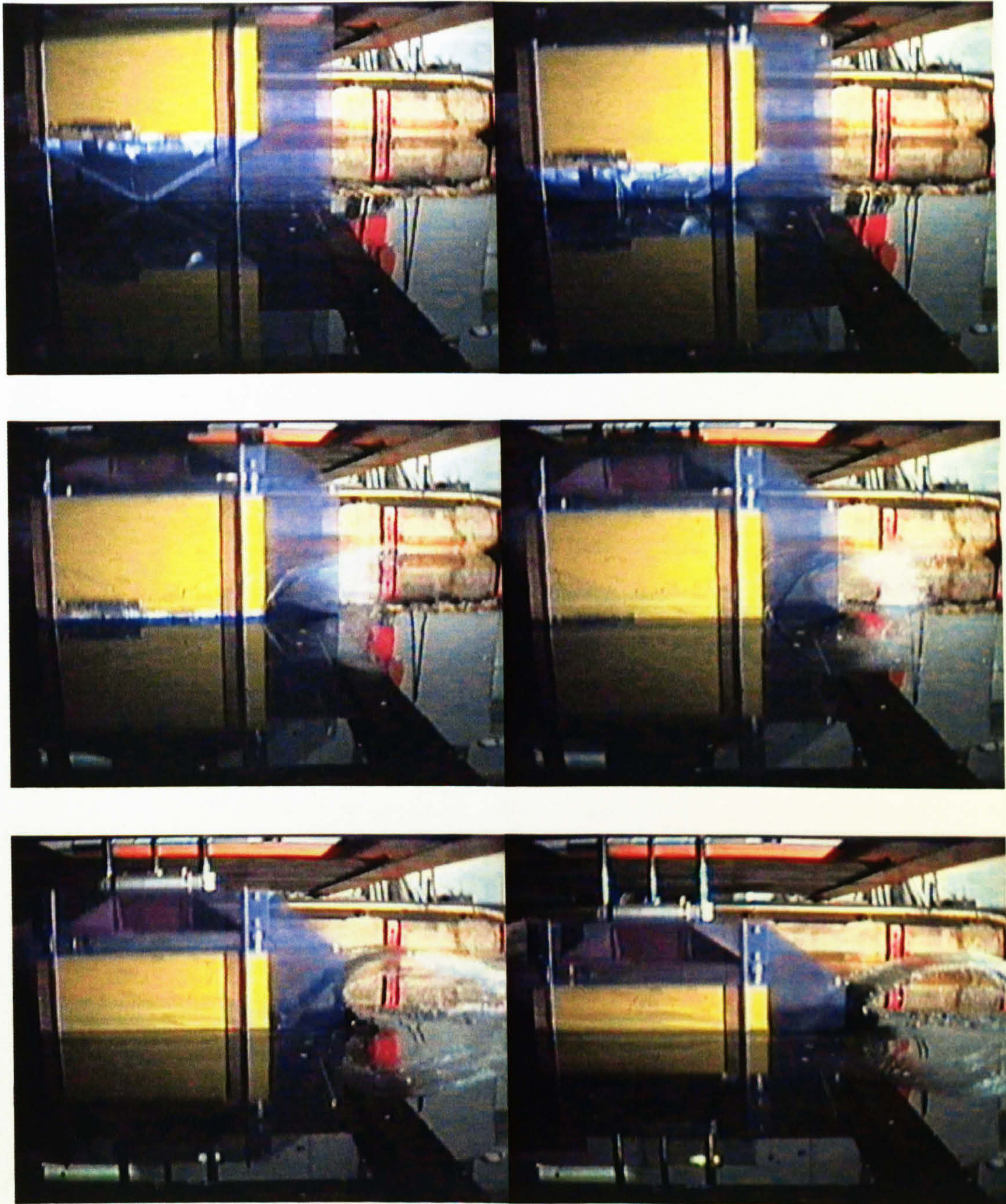
Figure 5-79. 30 degree constant velocity water entry.
