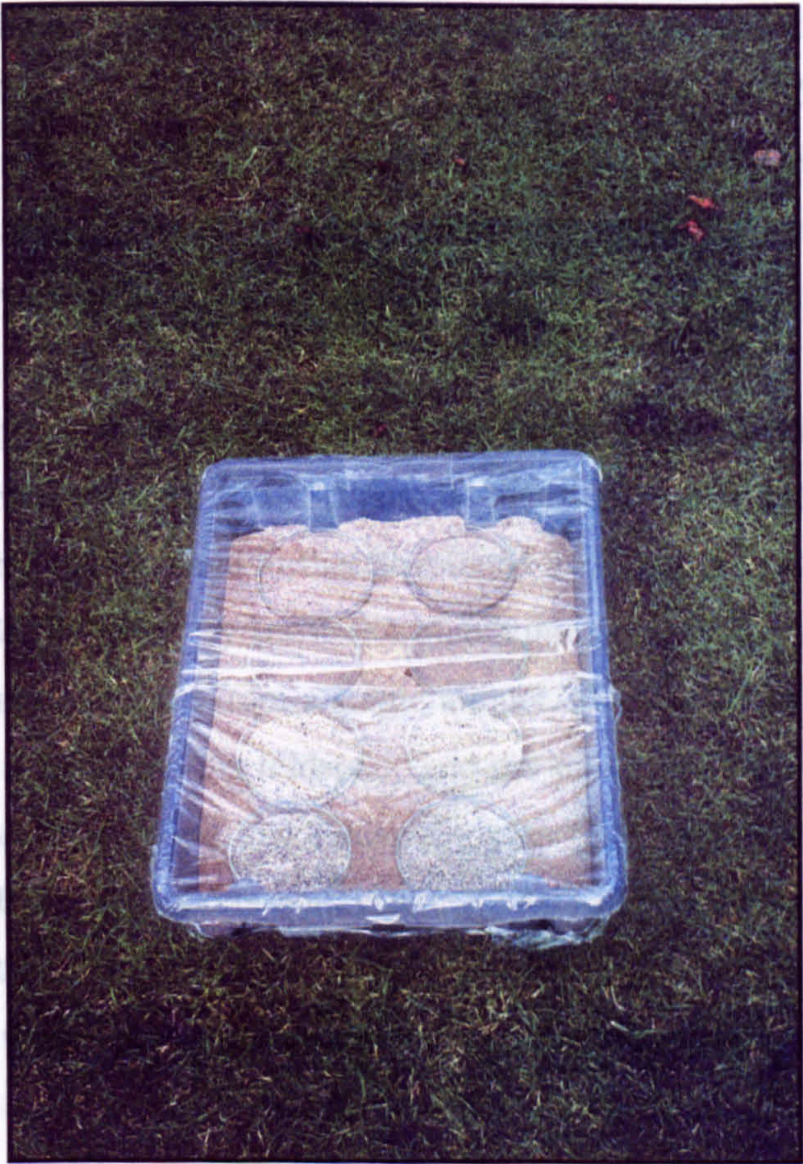
Figure 3.27 – Field bleaching experiment. Two glass petri dishes per sample in a perspex container filled with sand and covered with cling-film to prevent contamination of the samples.
