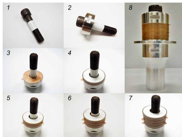
Figure 5.2 Exciter section assembly steps.
