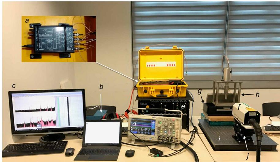
Figure 6.3 HRC equipment: (a) 4-channel DAQ; (b) power amplifier; (c) PC with MATLAB and DAQ software; (d) 4-channel oscilloscope with signal generator; (e) laser signal processor; (f) sensor head; (g) translation stage; (h) resonator fixture; (i) breadboard; (j) lab-jack.
