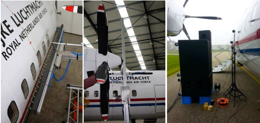
(b) Microphone array mounted on transversing mechanism for the reciprocal (c) Transfer function measurements using a transmission loss measurements method. direct technique.
