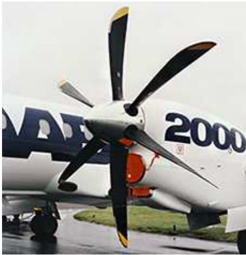
(b) Dowty Propellers R381 propeller system for the Saab 2000.
