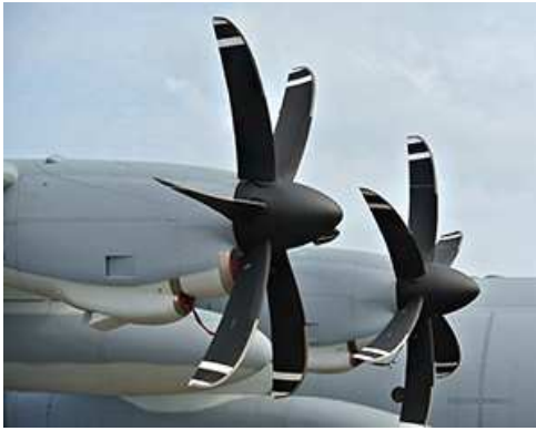
(a) Dowty Propellers R391 propeller system for Lockheed Martin's C-130J Super Hercules. The same design is used on the Alenia Aeronautica C-27J.
