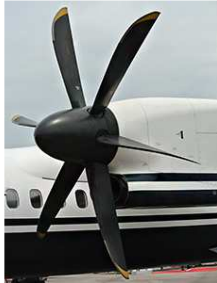
(c) Dowty Propellers R408 propeller system of the Bombardier Q400 Dash 8. The same design is used on the Antonov AN-132D and the AVIC's MA700.
