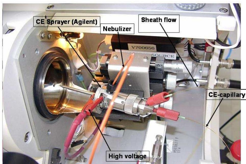
Figure 2-5. Interface of capillary and mass spectrometer
