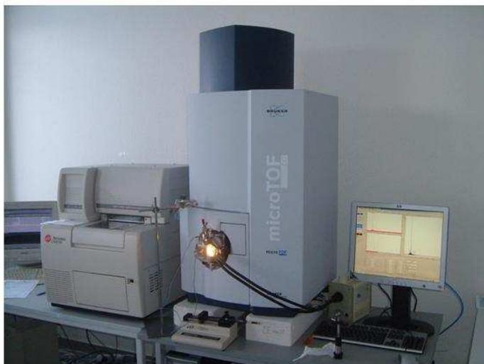
**Figure 2-4. Capillary electrophoresis (left), microTOF mass spectrometer (middle) and computer for data acquisition (right).**
