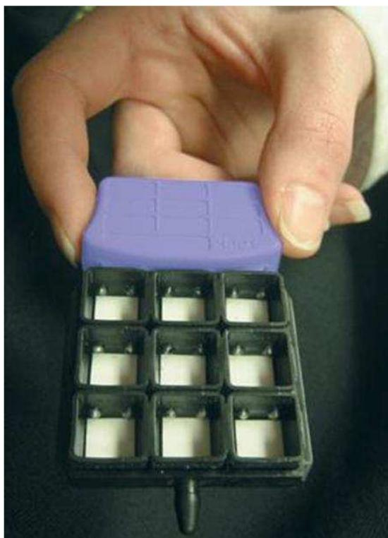
**Figure 2-2. Biochip carrier with 9 reaction wells.**
