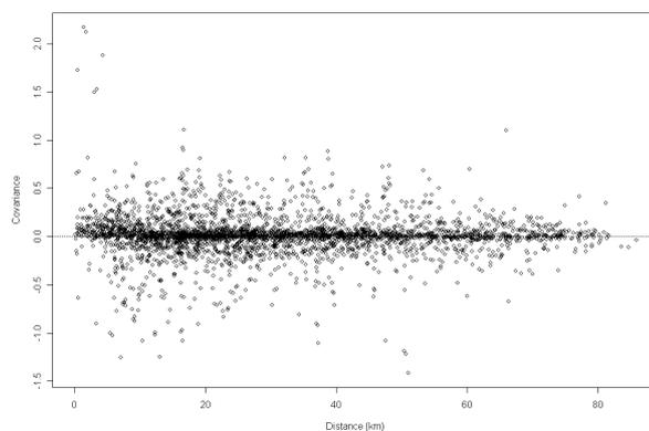
**Figure 2.7.** Covariogram cloud based on Euclidean distance
