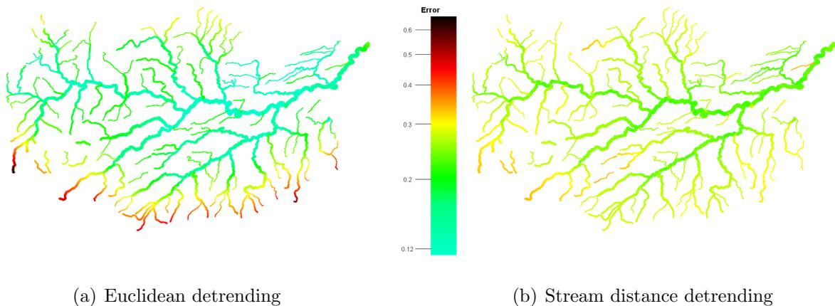
**Figure 4.10.** Comparison of kriging error in 1998 for different detrending methods
