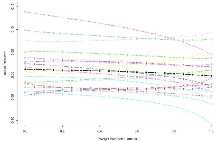
**Figure 3.2.** Assessing Bias in the Euclidean distance detrended results by looking at difference between actual value and predicted value
