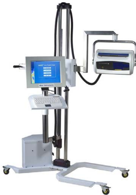
Figure 4-1 - Moor Laser Doppler Scanner LD12-IR & its use intraoperatively.
