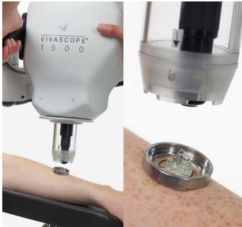
Figure 2-2 - Vivascope 1500 attaching to skin surface to be examined. Steel ring attaches to skin with adhesive.
