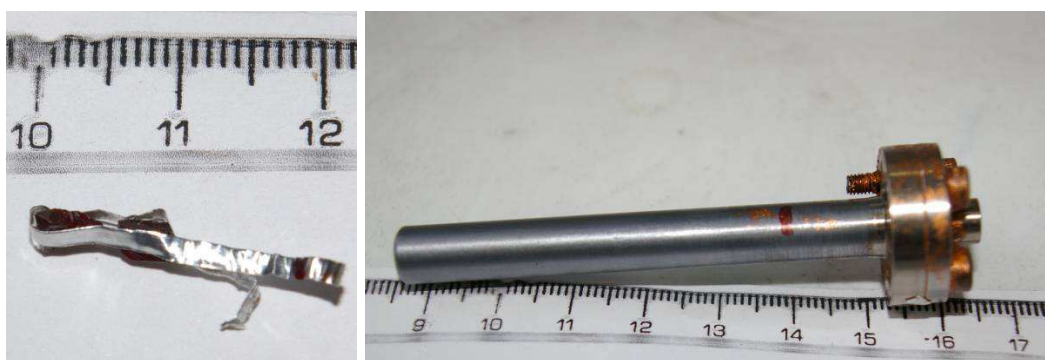
Figure 7-2. The two crystals mounted for the multiple crystal sample (left) and the vanadium can (right) used in the neutron diffraction experiment on SXD. Each interval on the ruler represents 1 mm.
