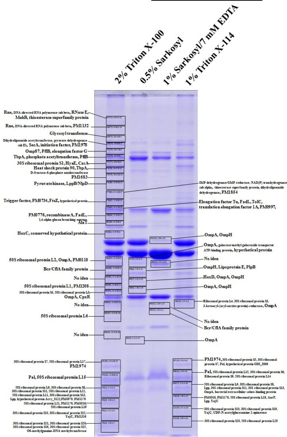
**Figure 3-6.** 1D-SDS-polyacrylamide gel showing excised bands from the OMP profiles of the bovine isolate PM632 prepared by 2% Triton X-100, 0.5% Sarkosyl, 1% Sarkosyl/7 mM EDTA and 1% Triton X-114. The identified proteins corresponding to the cut bands are labelled.
