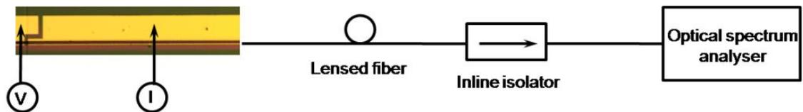
Figure 5.6: Schematic of experimental setup for optical spectra measurements.
