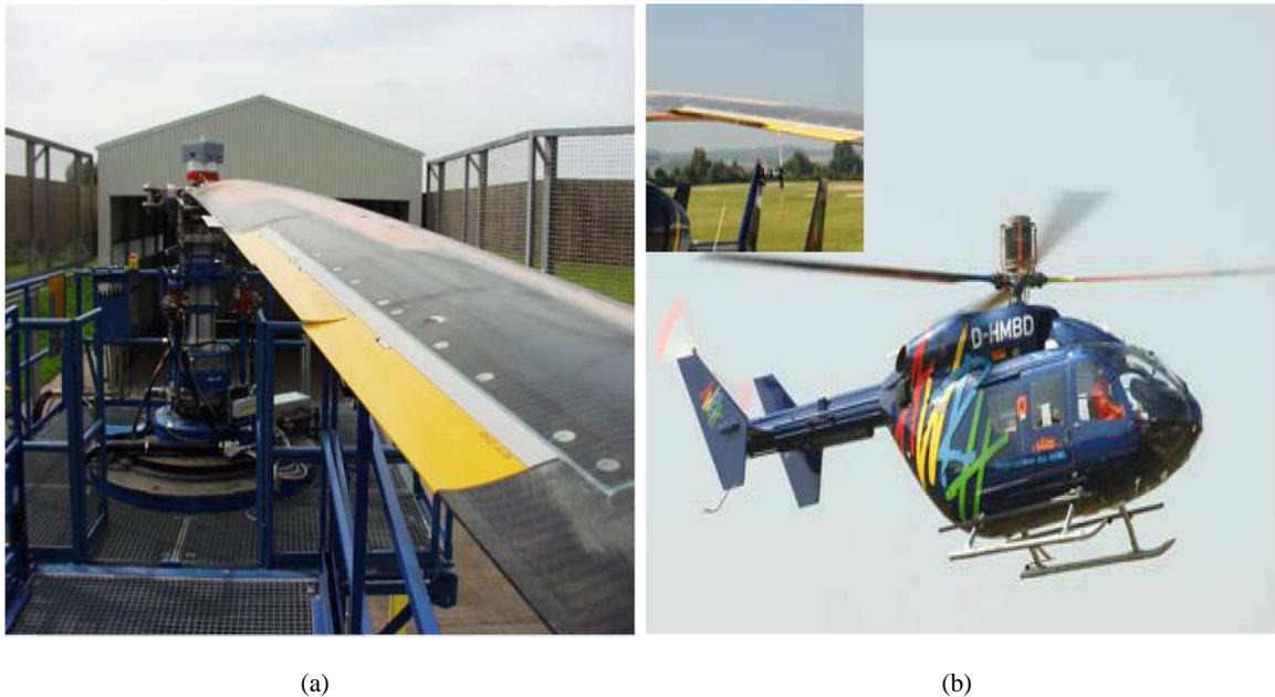
Figure 1.10: Flight tests of AFC for vibration reduction. (a) Whirl tower equipped with AFC blade. (b) BK117 in-flight with AFC blades. Taken from Ref. [18].
