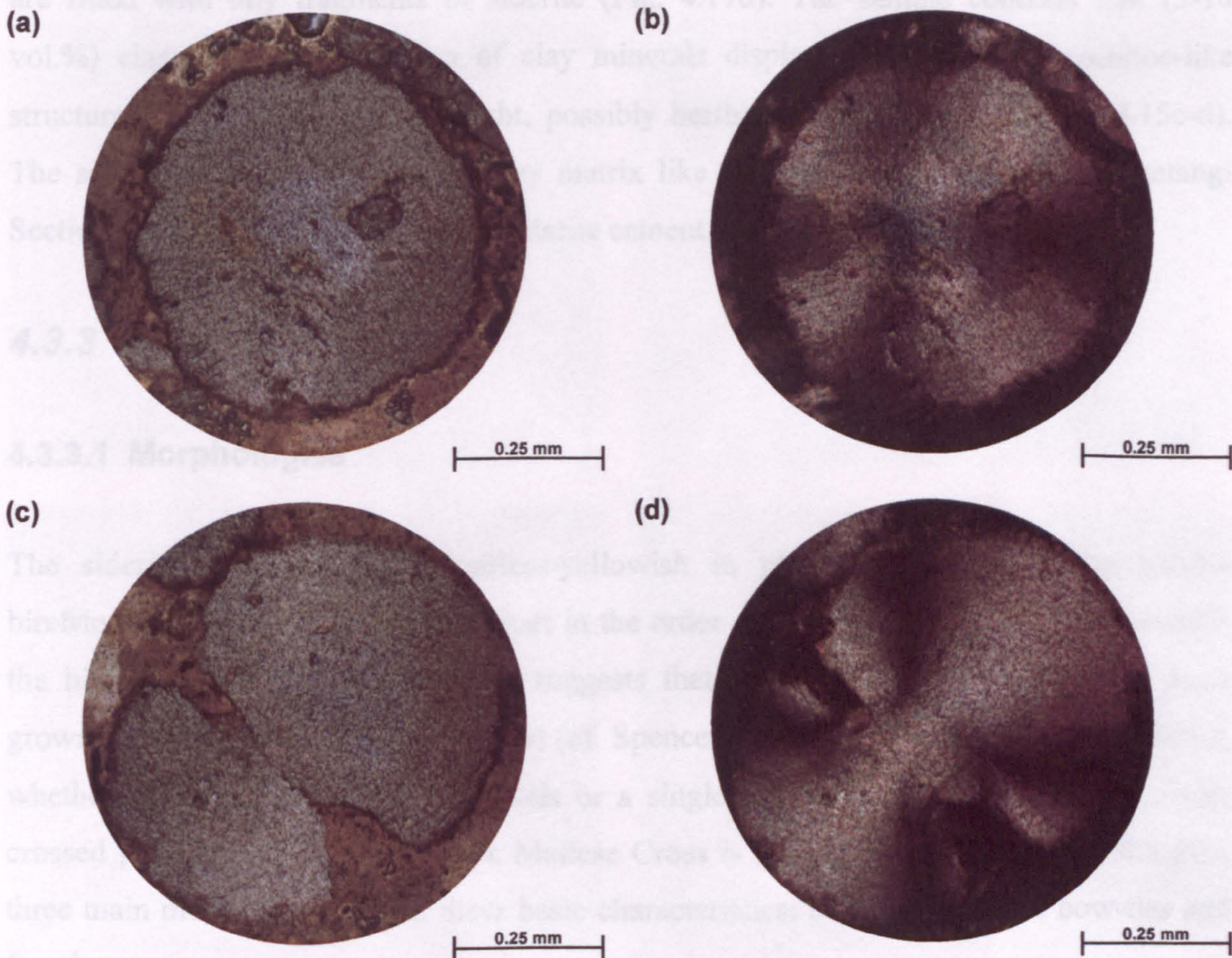
Fig. 4.16. Photomicrographs of siderite spherules from sample SUF.8.2, ironstone, Rokhagi Section, ca. 3.5 km SE of Hvalba, Suðuroy, Faeroe Islands. (a) Perfect siderite spherule showing no internal segmentation. (b) Same view as in (a) under cross-polarised light. Notice the Maltese Cross extinction pattern. (c) Bow-tie shaped siderite spherule, which has grown unevenly. (d) Same view as in (c) under cross-polarised light. Notice the Maltese Cross extinction pattern.
