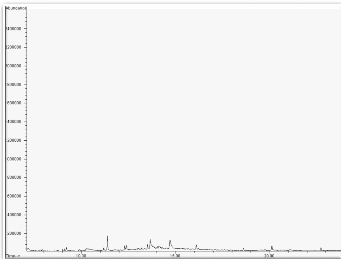
Figure 6-21: An example of a SIM Chromatogram for an endogenous interferences study using a blank urine specimen without the addition of ISD
