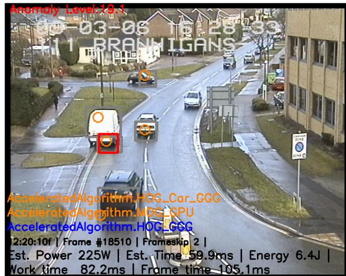
Figure 6.12: An anomaly detection is logged. The red box indicates a van parked in a forbidden location.
