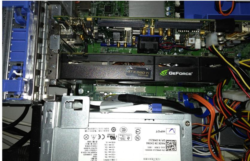
Figure 4.1: ML605 FPGA card (upper) and GPU card (lower) in development system.
