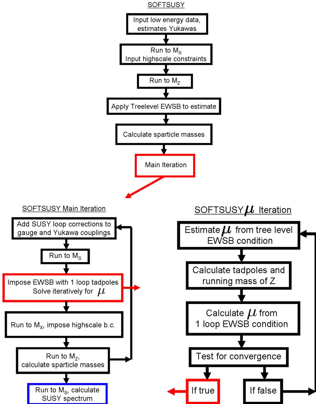
Figure 4.1: Flow chart showing how SOFTSUSY finds sparticle spectra consistent with high scale boundary conditions (e.g. those of the CMSSM), correct EWSB and low energy data from experiments.
