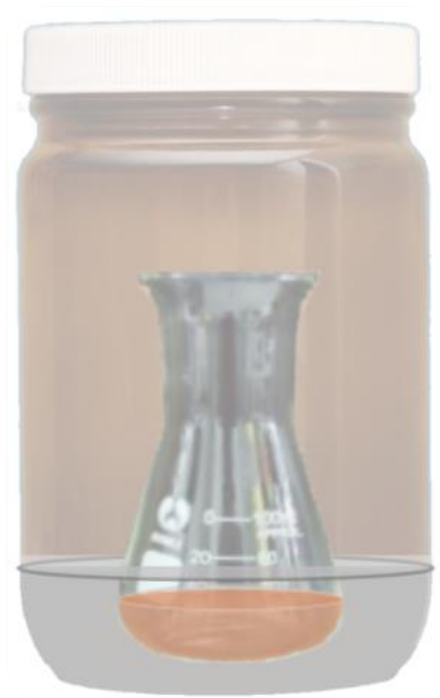
Figure 119: Representation of the crystallisation set-up: compound solution contained in a 50 mL conical flask inserted into a 500 mL tub with Et 2 O. The mother liquor is shown in orange, whilst the grey area represents the Et 2 O.
