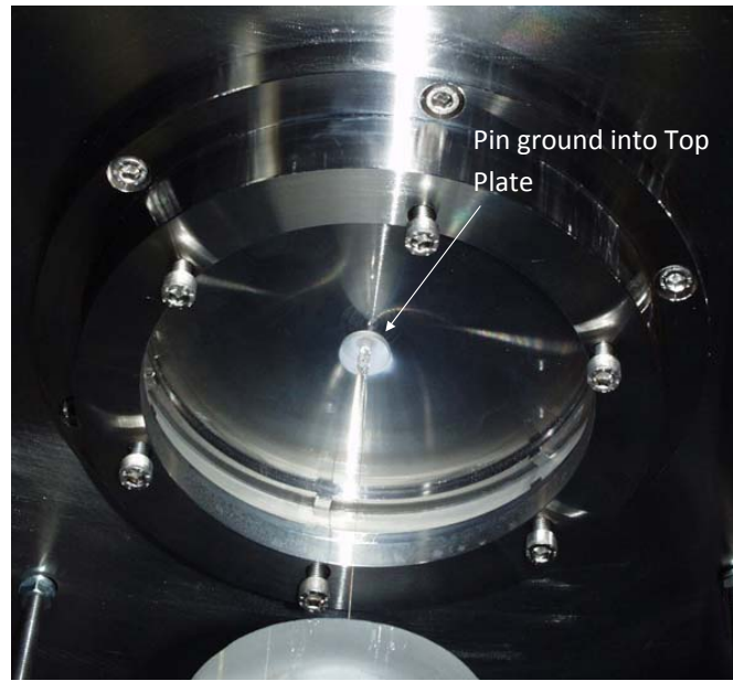
Figure 4.6: Isolation mass, upper fibre and top clamp plate system.
