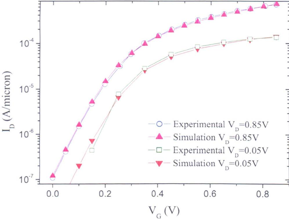
Figure 6.8: Calibrated  $I_D$ - $V_G$  characteristics of the 35 nm physical gate length n-type Si MOSFET; experimental data from Inaba *et al.* [181]
