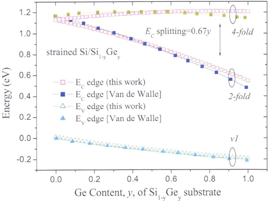
Figure 3.9: Calculated conduction band splitting and the valence band edge of strained Si on relaxed Si<sub>1-y</sub>Ge<sub>y</sub> as a function of Ge composition  $y$  (assuming the valence band edge of Si as the reference zero of the energy level), compared with the work by Walle *et al.* [120] and Rieger *et al.* [121]
