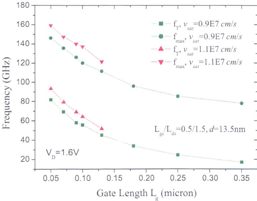
Figure 4.15: Intrinsic RF characteristics versus the gate length at  $V_D=1.6 \text{ V}$  (the gate-to-channel distance=13.5 nm)
