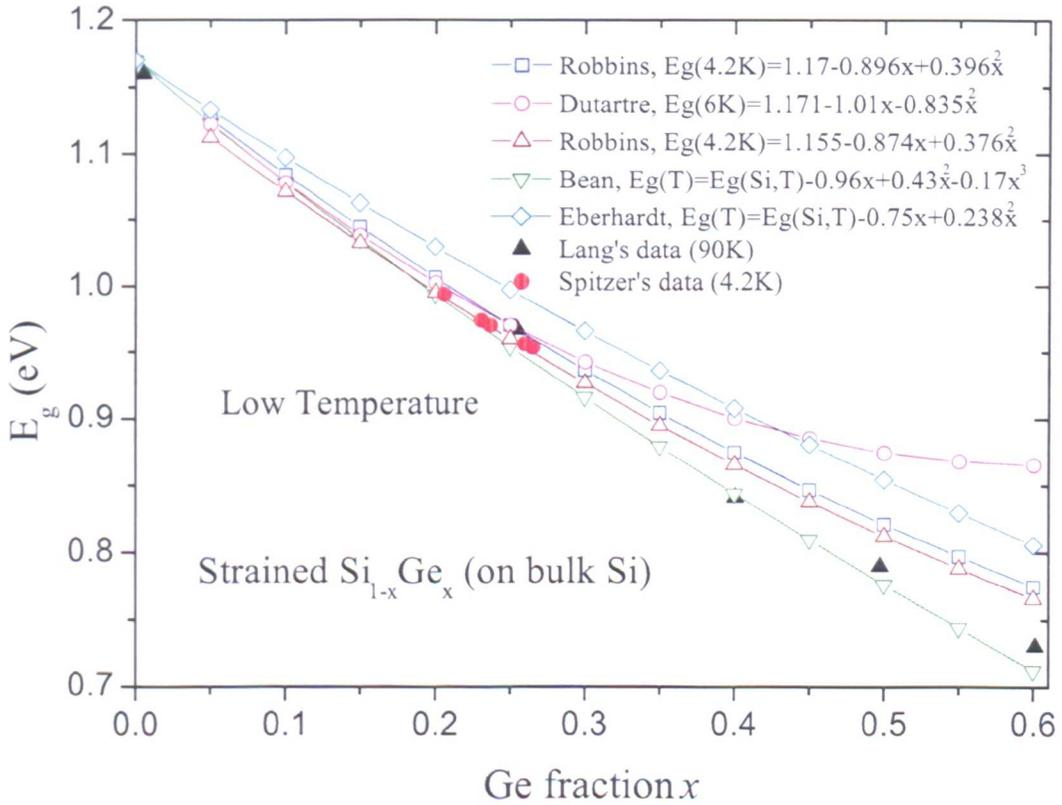
Figure 3.4: Bandgap of strained  $\text{Si}_{1-x}\text{Ge}_x$  on Si (001) substrate
