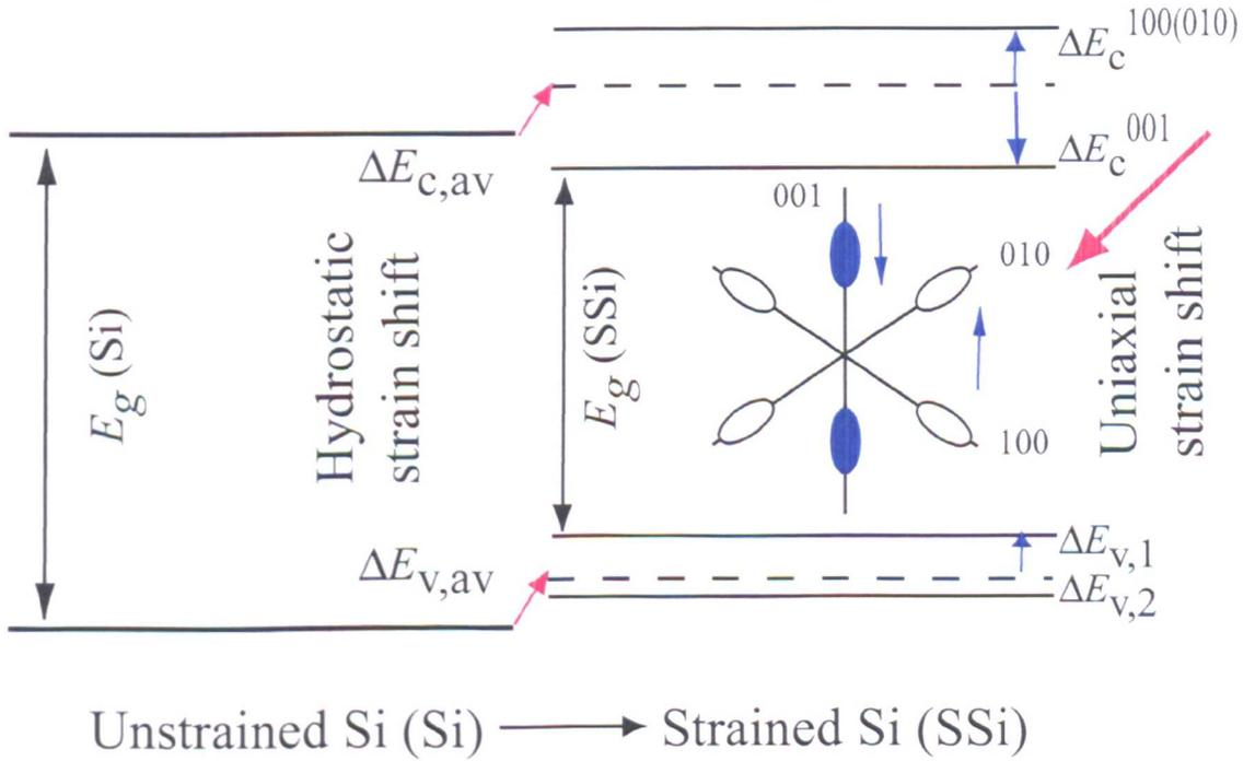
Figure 3.5: The strain effects to the band structure of silicon
