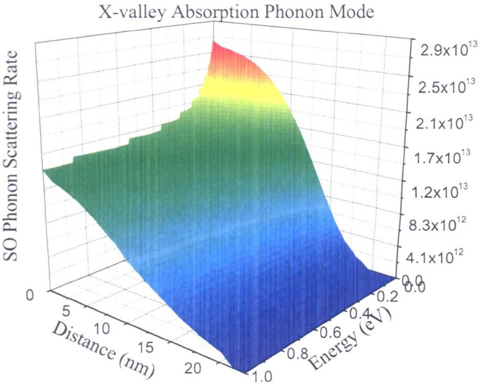
Figure 6.2: Scattering rate of soft optical phonon scattering in a Si/HfO<sub>2</sub> system (absorption mode of phonon mode 1 ( $\omega_{SO1}$ ) in  $X$ -valley)
