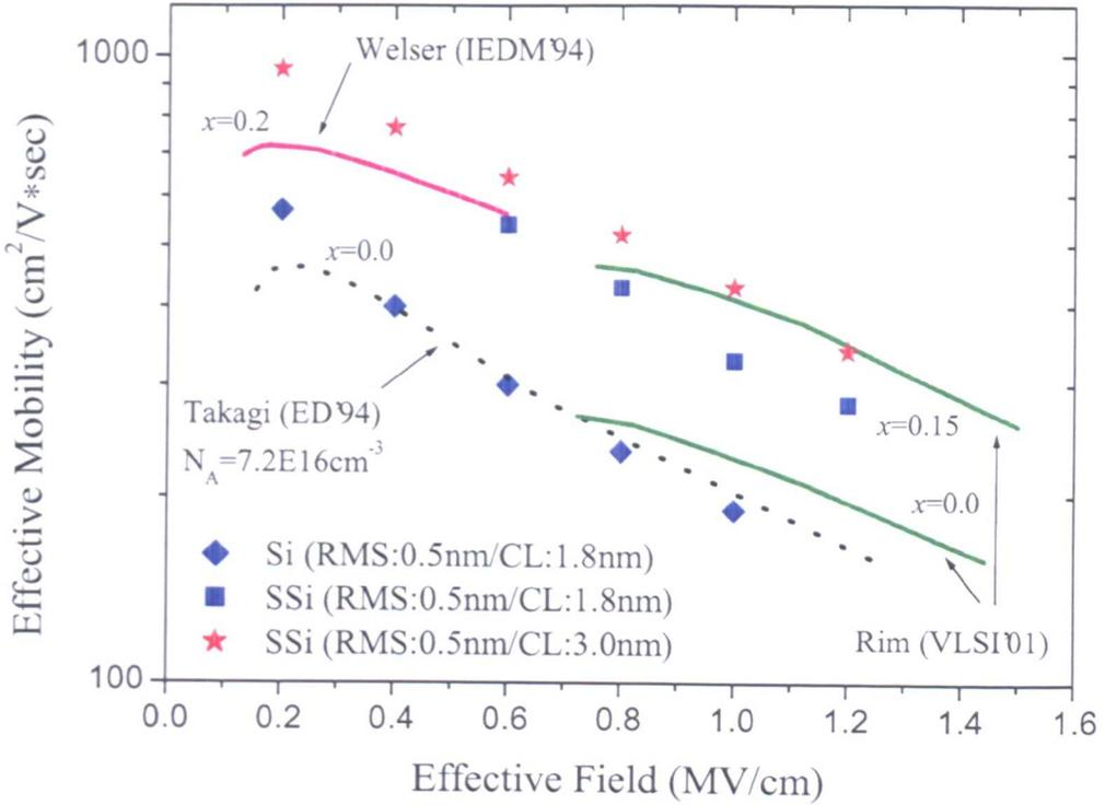
Figure 6.5: Field dependence of the effective electron mobility of strained Si, compared with data from Rim *et al.* [31] and Welser *et al.* [67]
