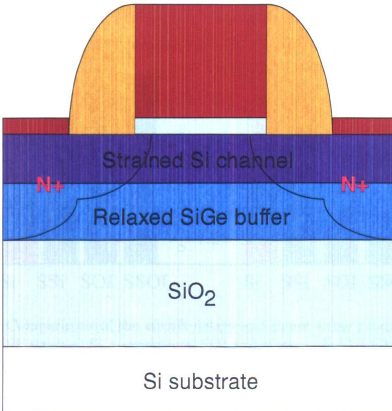
Figure 5.18: Illustration of simulated strained Si on SiGe on insulator device structure
