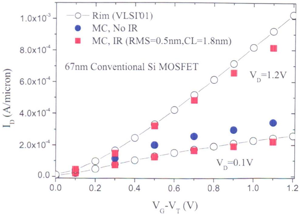
Figure 6.4: Monte Carlo simulated  $I_D$ - $V_G$  characteristics of the 67 nm Si MOSFET with and without IR scattering, compared with data from Rim *et al.* [31]
