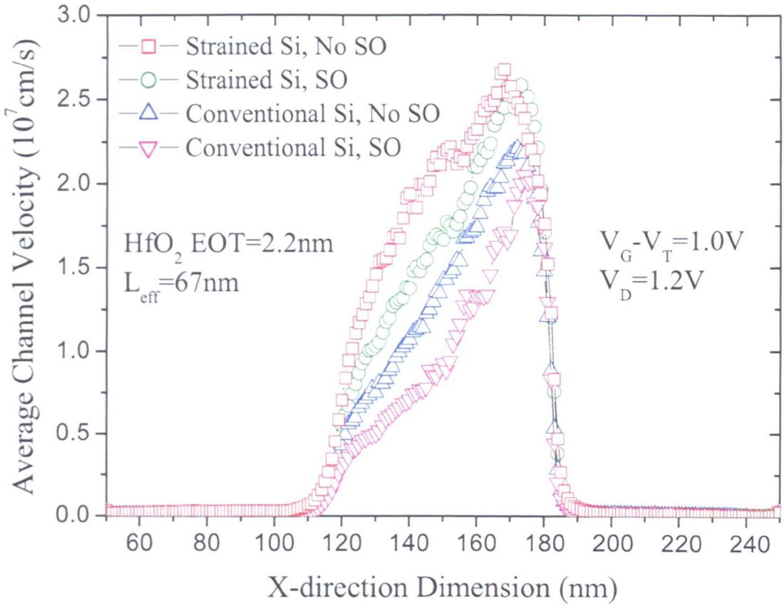
Figure 6.14: Average channel velocities obtained from MC simulations with and without SO phonon scattering in the 67 nm conventional and strained Si MOSFETs
