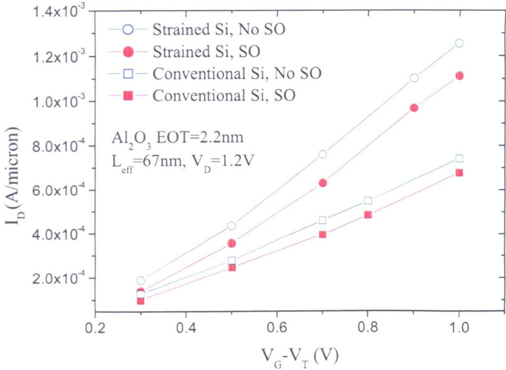
Figure 6.15: Performance comparisons of Monte Carlo simulations with and without soft optical phonon scattering in 67 nm n-type conventional and strained Si MOSFETs with Al<sub>2</sub>O<sub>3</sub> gate dielectrics at  $V_D=1.2\text{V}$
