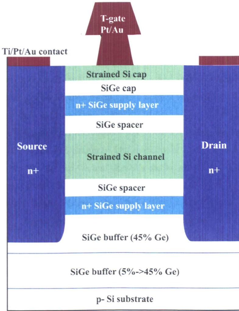
Figure 4.4: Illustration of simulated strained Si/SiGe MODFET
