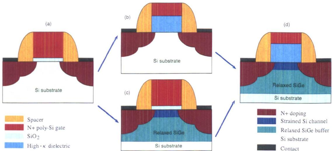
Figure 6.11: Schematics of the simulated devices: (a) conventional Si MOSFET with  $\text{SiO}_2$ ; (b) conventional Si MOSFET with high- $\kappa$  dielectrics; (c) strained Si MOSFET with  $\text{SiO}_2$ ; (d) strained Si MOSFET with high- $\kappa$  dielectrics
