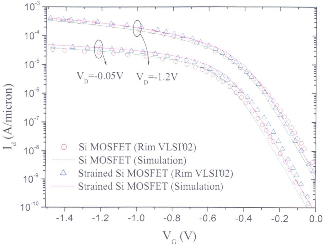
Figure 5.7: Calibrated  $I_D$ - $V_G$  characteristics of the 90 nm gate length Si and strained Si p-MOSFETs
