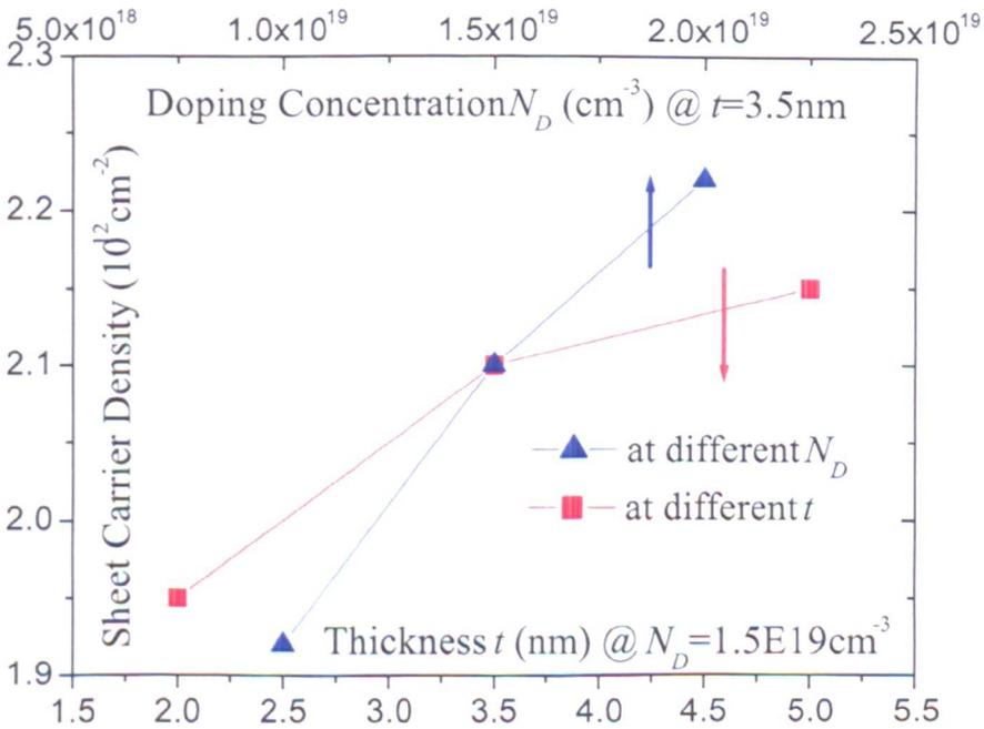
Figure 4.17: Effects of the front supply layer thickness and the doping concentration on the modulation efficiency and the sheet carrier density in the channel (the sheet carrier densities plotted in the second figure are extracted at the  $ME = 0.8$  within the first figure)
