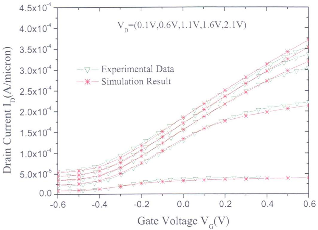
Figure 4.7: Calibrated  $I_D$ - $V_G$  characteristics of the  $0.25 \mu\text{m}$  MODFET
