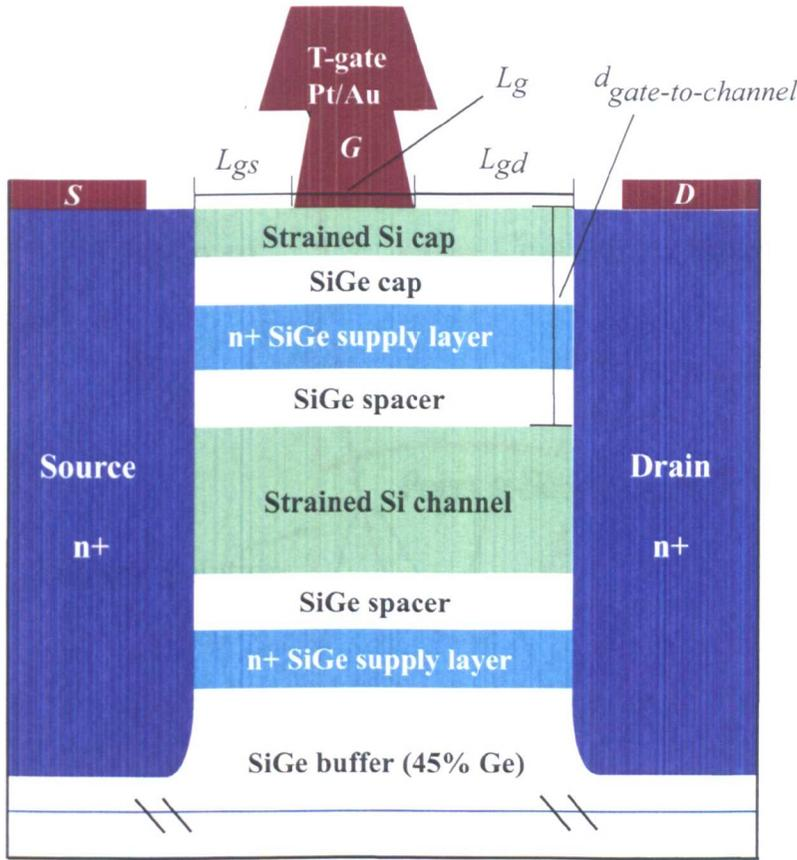
Figure 4.5: Schematic of strained Si/SiGe MODFET
