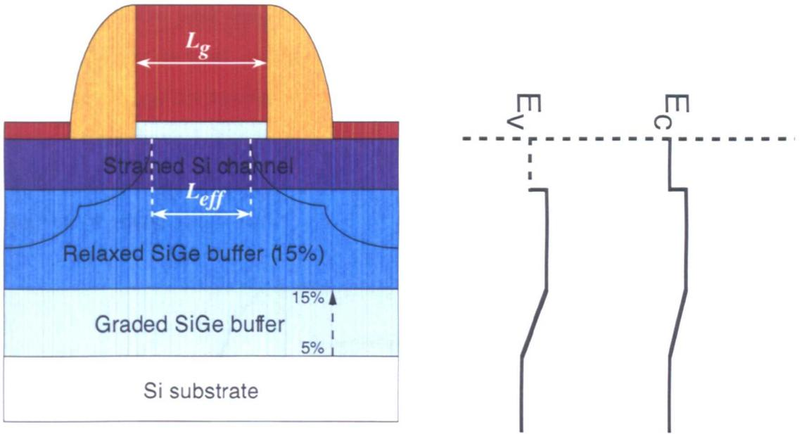
Figure 5.2: Schematic of strained Si MOSFET and band diagram along the middle of the device
