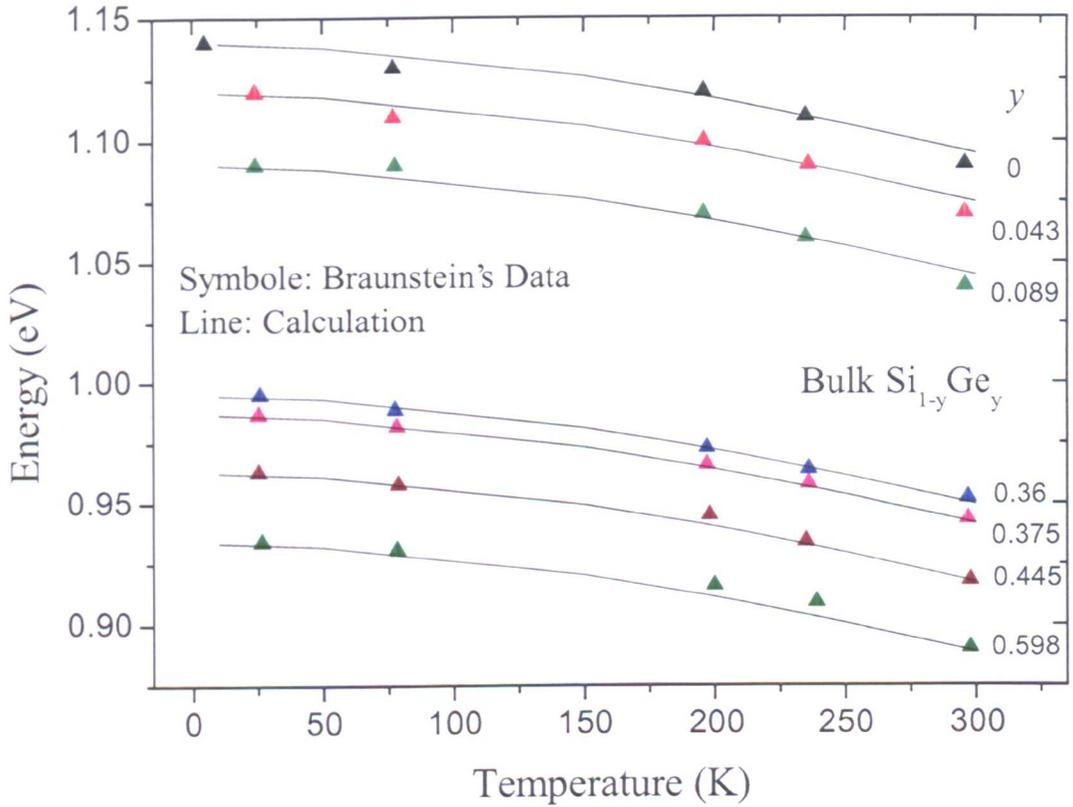
Figure 3.3: Temperature dependence of the bandgap for  $\text{Si}_{1-y}\text{Ge}_y$  bulk alloys
