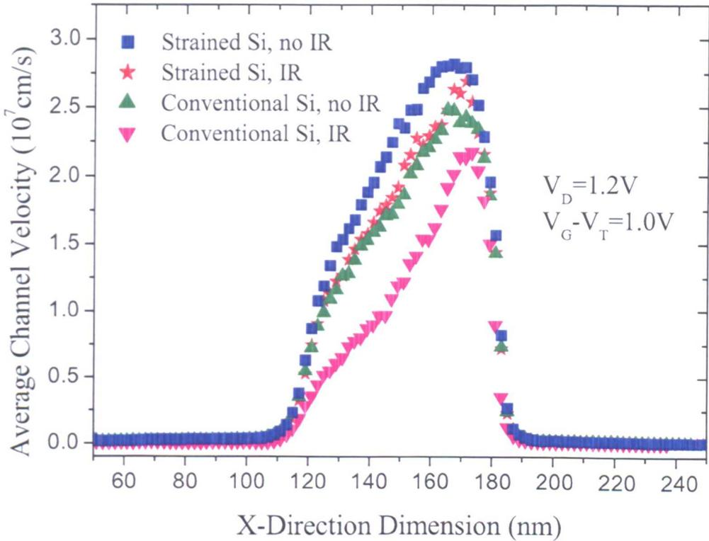
Figure 6.7: Monte Carlo simulated average channel velocities of the 67 nm n-type conventional Si and strained Si MOSFETs with and without interface roughness scattering
