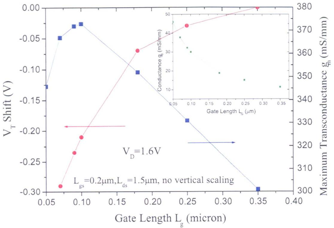
Figure 4.11: Threshold voltage shift and transconductance characteristics versus the gate length; the inset is the output conductance characteristics
