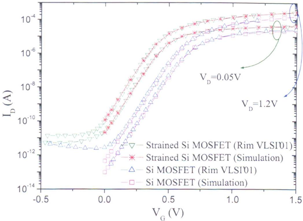
Figure 5.4: Calibrated  $I_D$ - $V_G$  characteristics of the 80 nm gate length Si and strained Si n-MOSFETs
