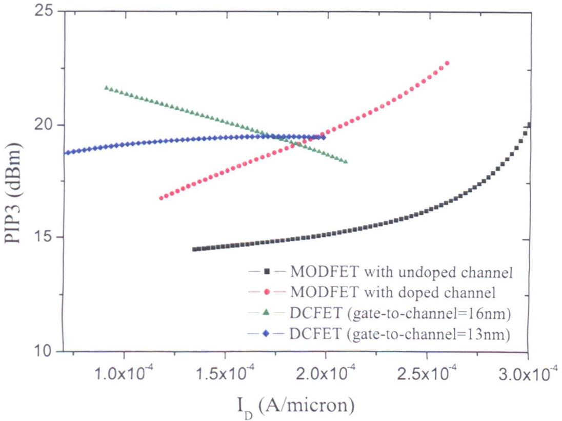
Figure 4.24: The comparison of PIP3 between structure A (undoped channel MODFET), structure B (doped channel MODFET) and structure C (DCFET)
