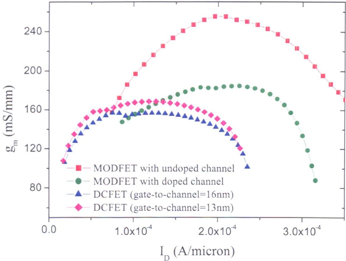
Figure 4.23: The comparison of device transconductance characteristics between structure A (undoped channel MODFET), structure B (doped channel MODFET) and structure C (DCFET)
