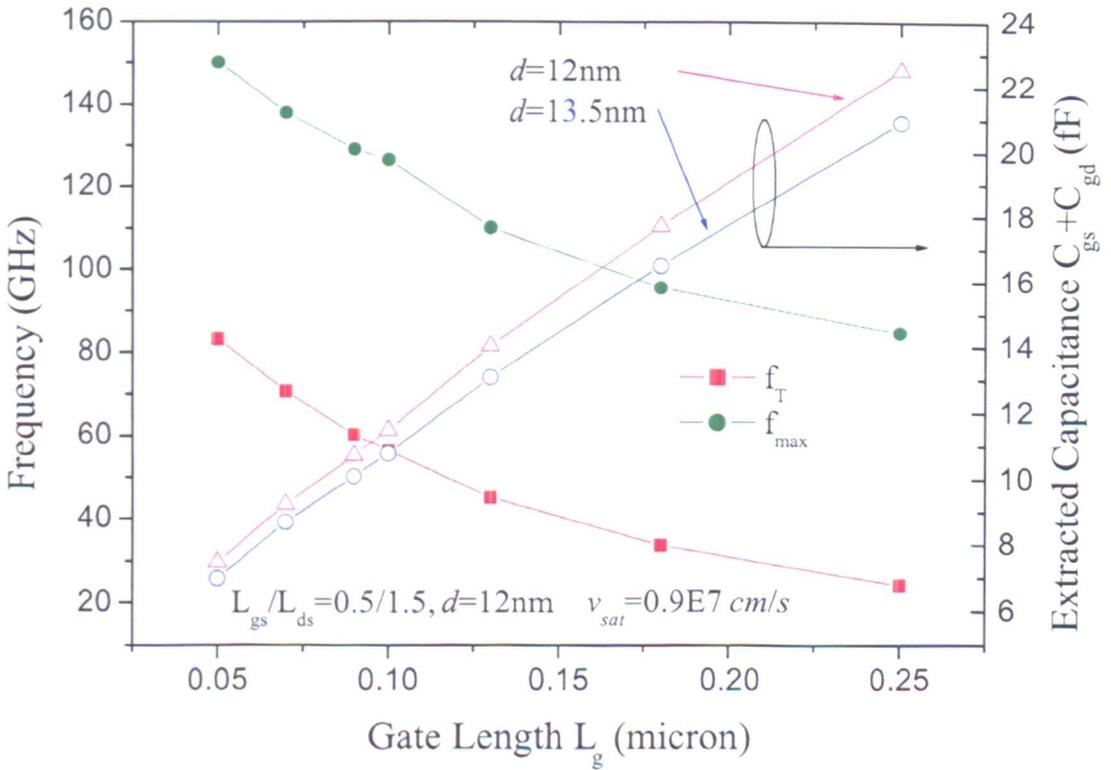
Figure 4.18: Extracted intrinsic RF characteristics and capacitance ( $C_{gs} + C_{gd}$ ) versus the gate length at  $V_D=1.6$  V, the gate-to-channel distance=12 nm
