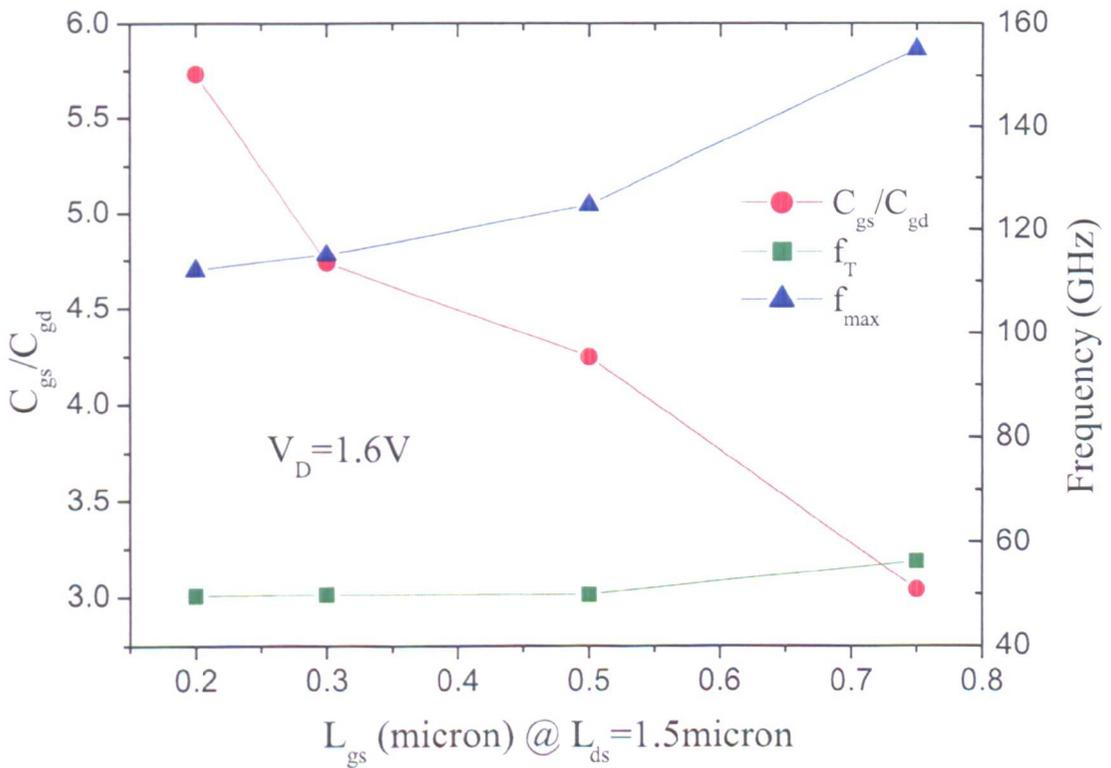
Figure 4.13: Effects of different  $L_{gs}/L_{ds}$  ratio (different  $L_{gs}$  with a fixed  $L_{ds}$ ) on the device characteristics ( $L_g = 0.1 \mu\text{m}$ ; all values are extracted from the MEDICI transient simulation without  $R_g$ ,  $R_d$  and  $R_s$ )
