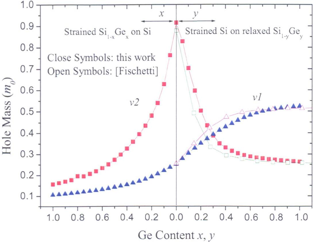
Figure 3.10: Calculated hole effective mass in band  $v1$  and  $v2$  from full-band  $k\bullet p$  calculations, compared with data from Fischetti *et al.* [142]
