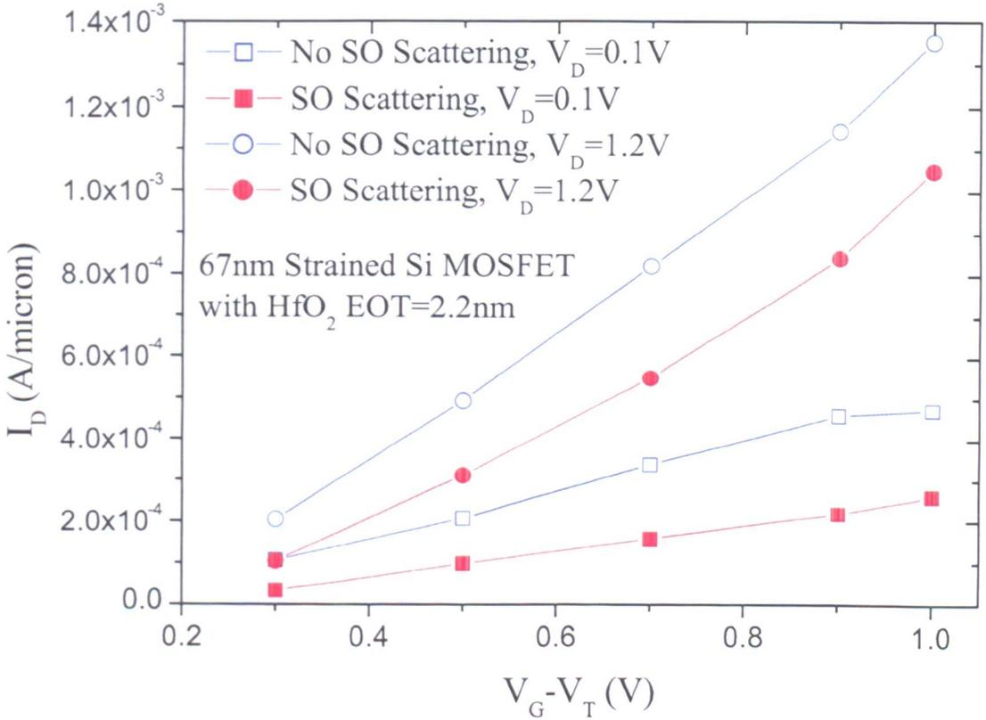
Figure 6.13: Monte Carlo simulated  $I_D$ - $V_G$  characteristics with and without SO phonon scattering of the 67 nm strained Si MOSFET with HfO<sub>2</sub> gate dielectrics.
