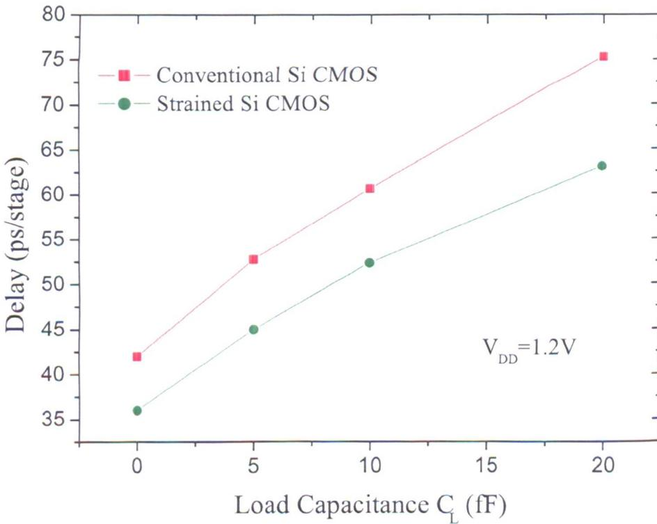
Figure 5.16: Circuit delays versus the load capacitance for the 67 nm Si and strained Si CMOS 3-stage ring oscillators
