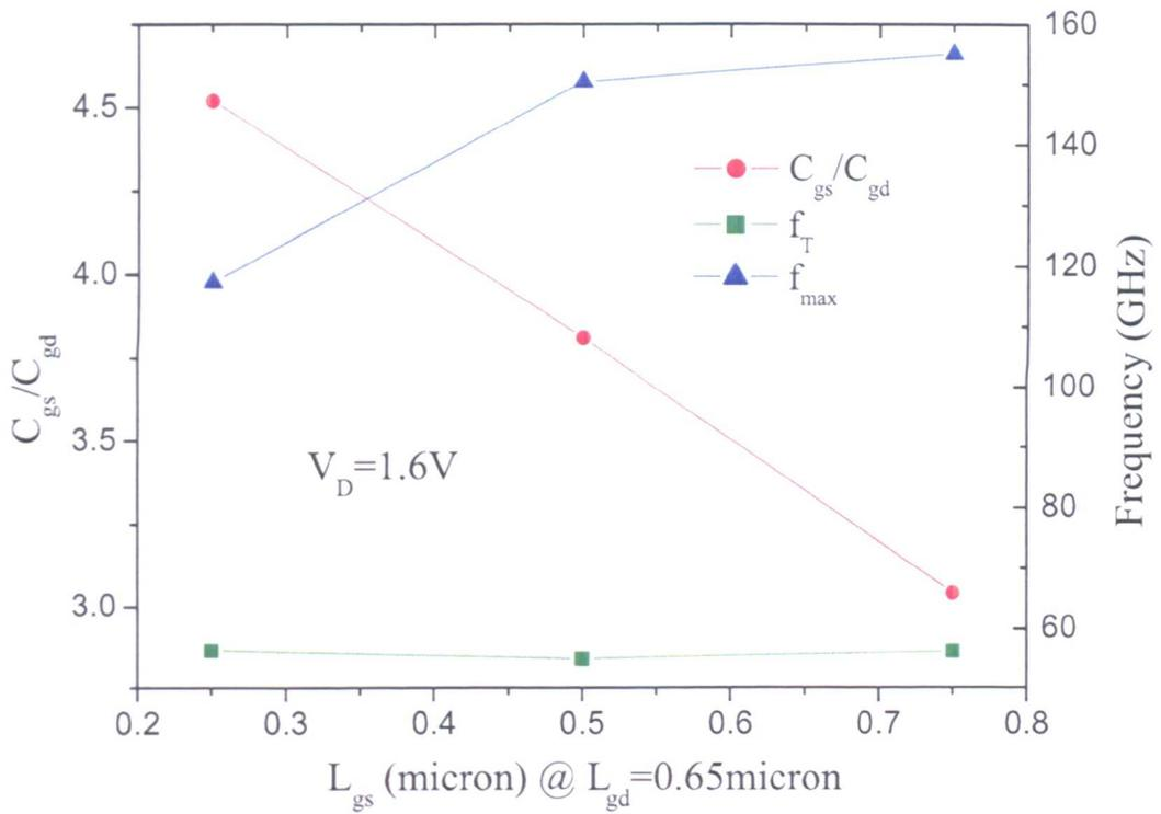
Figure 4.14: Effects of different  $L_{gs}/L_{ds}$  ratio (different  $L_{gs}$  with a fixed  $L_{gd}$ ) on the device characteristics ( $L_g=0.1 \mu\text{m}$ ; all values are extracted from the MEDICI transient simulation without  $R_g, R_d$  and  $R_s$ )
