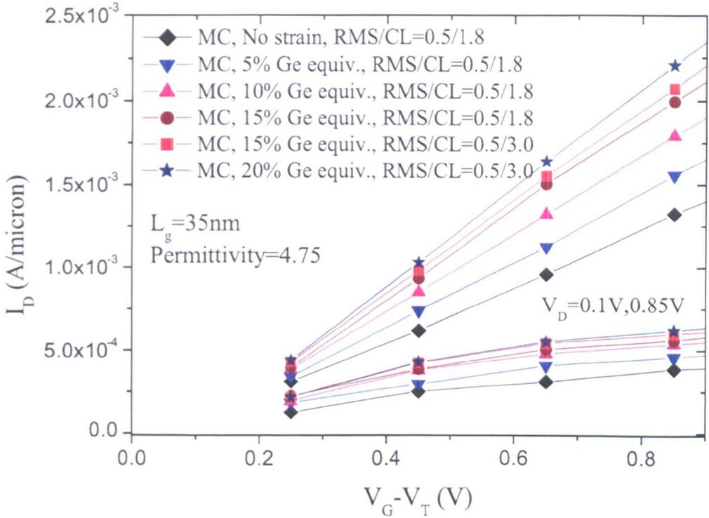
Figure 6.10: Monte Carlo simulated  $I_D$ - $V_G$  characteristics of 35 nm gate length n-type Si MOSFETs with different strain within the channel
