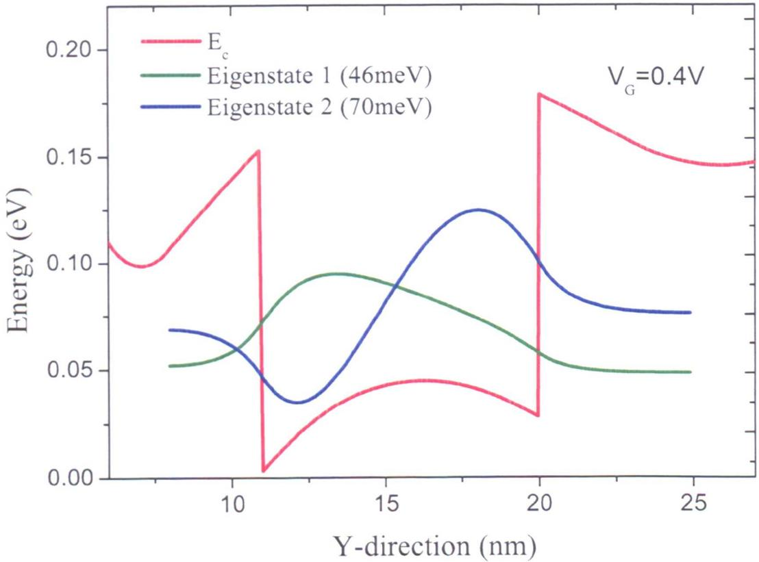
Figure 4.16: The conduction band diagram and the wave functions in a 9 nm thick strained Si channel
