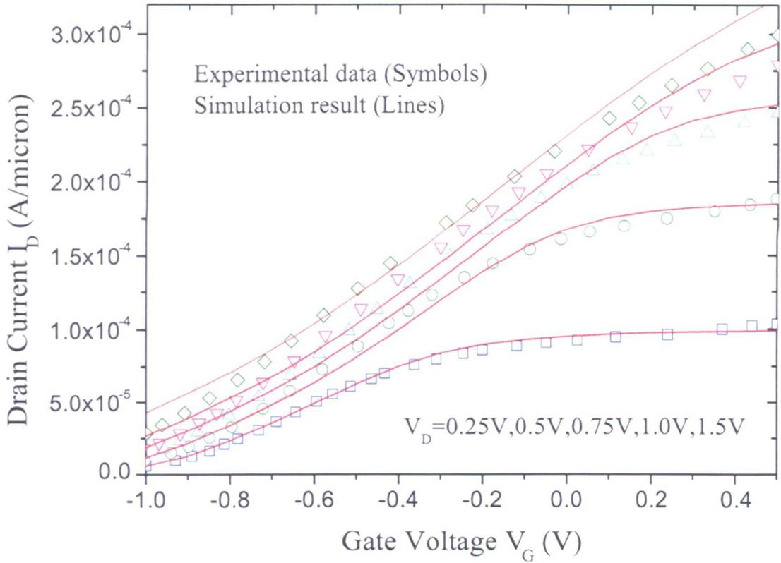
Figure 4.10: Calibrated  $I_D$ - $V_G$  characteristics of the 70 nm MODFET
