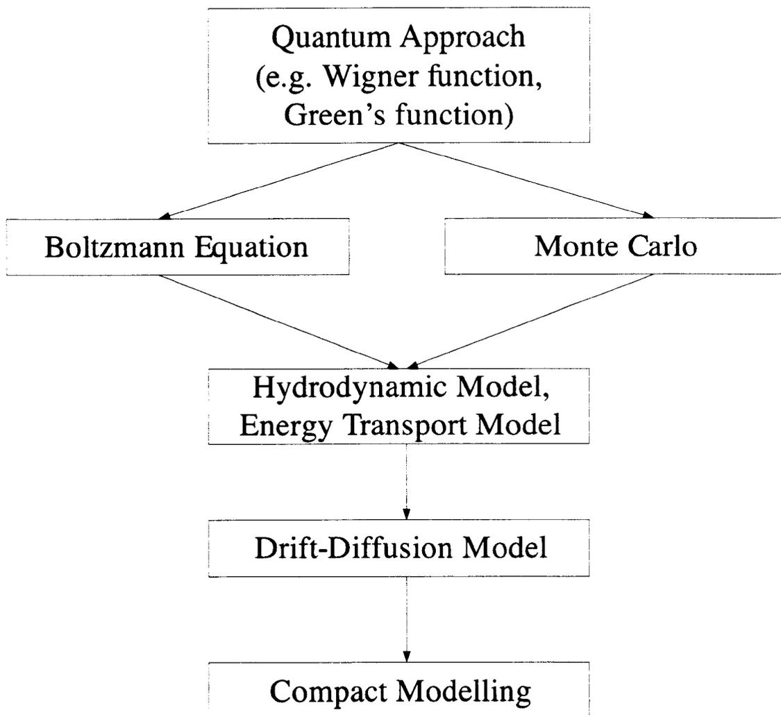
Figure 3.1: Hierarchy of semiconductor simulation models [123]
