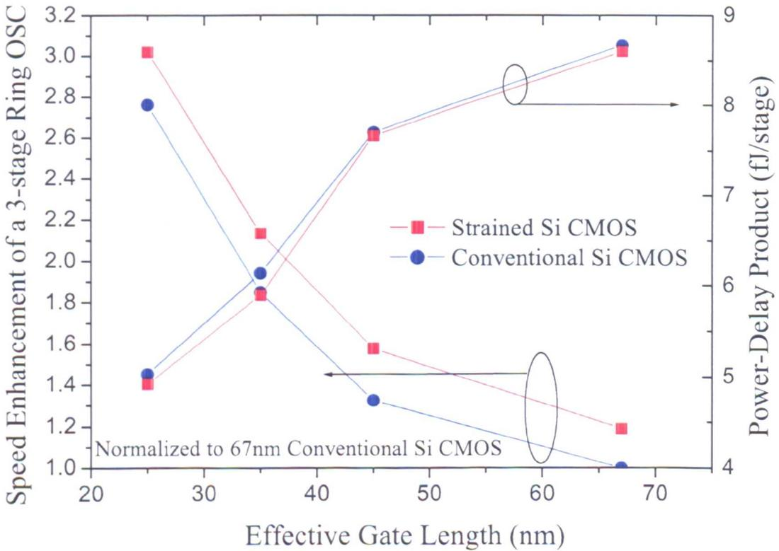
Figure 5.17: Speed enhancement and power-delay products against the effective gate length for Si and strained Si CMOS unloaded 3-stage ring oscillators
