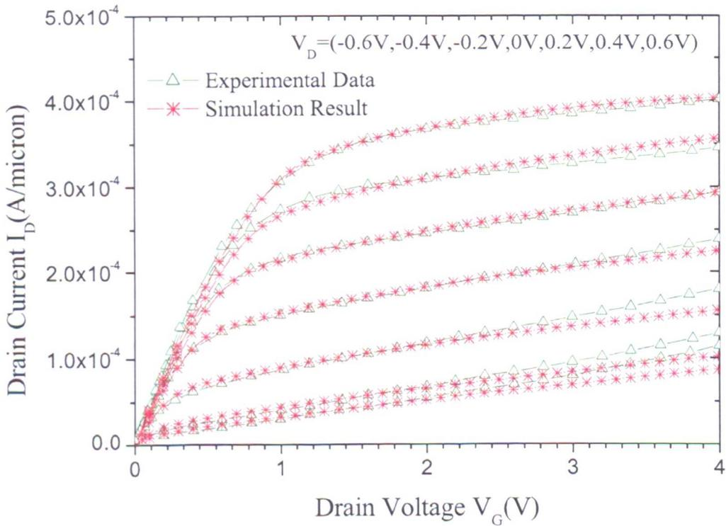
Figure 4.8: Calibrated  $I_D$ - $V_D$  characteristics of the  $0.25 \mu\text{m}$  MODFET
