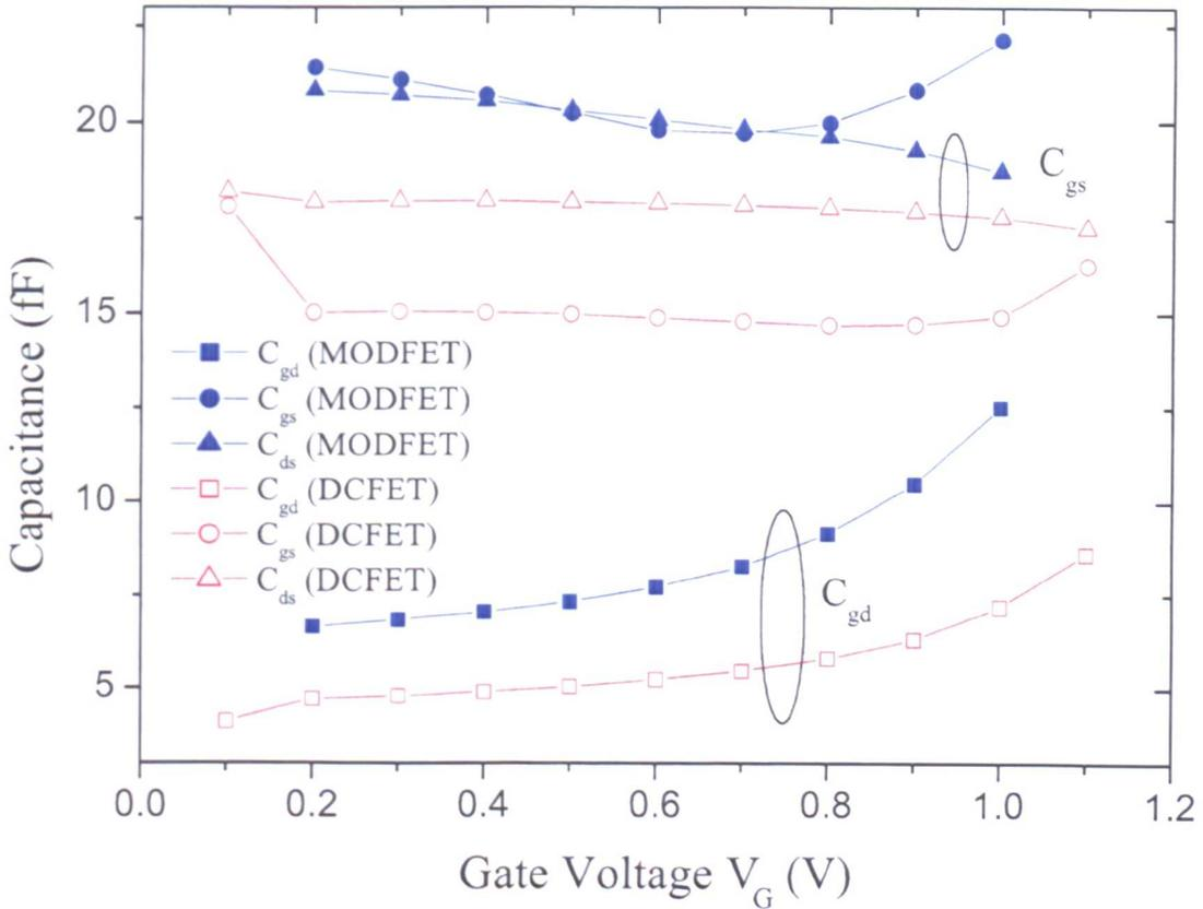
Figure 4.25: The comparison of intrinsic capacitances between structure A (undoped channel MODFET) and structure C (DCFET) at  $V_D=1.5$  V
