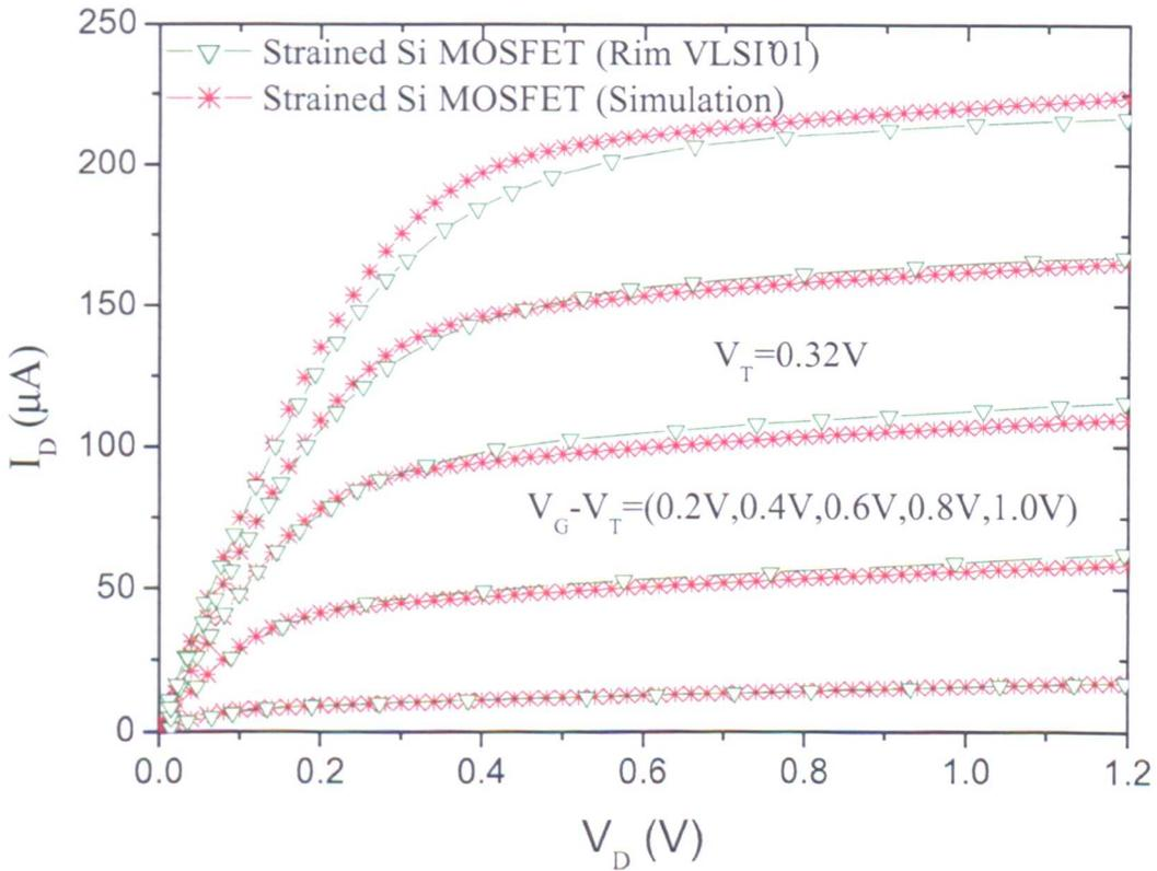
Figure 5.6: Calibrated  $I_D - V_D$  characteristics of the 80 nm gate length strained Si n-MOSFET
