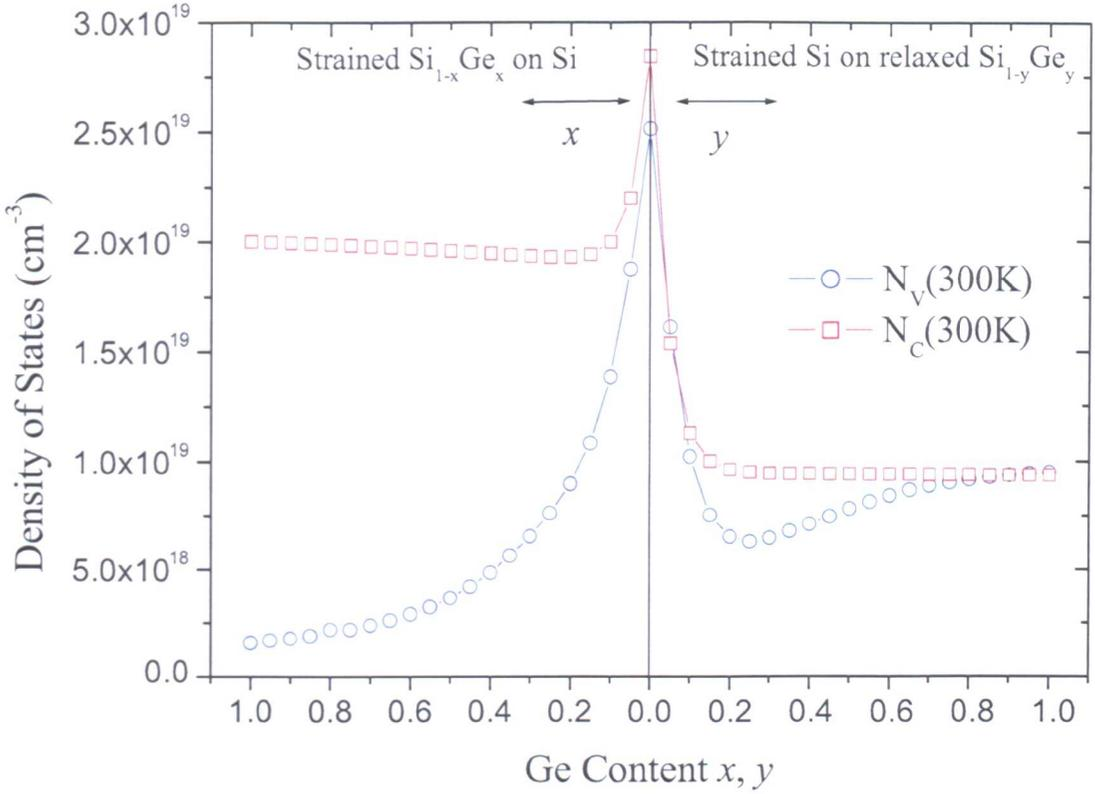
Figure 3.11: Calculated electron and hole density of states of tensile strained Si and compressive strained SiGe at 300K
