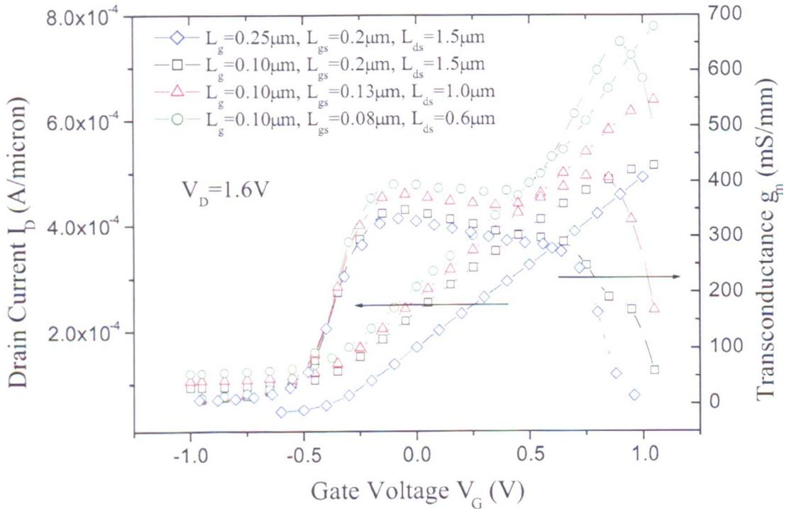
Figure 4.12: Drain current and transconductance characteristics with different lateral scaling strategies
