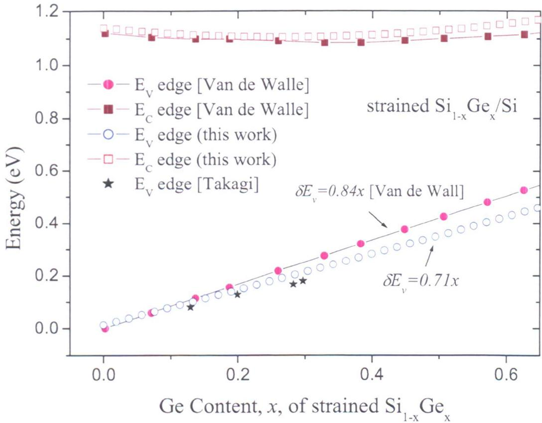
Figure 3.8: Calculated valence and conduction band offsets between strained Si<sub>1-x</sub>Ge<sub>x</sub> and unstrained Si (assuming the valence band edge of Si as the reference zero of the energy level), compared with the data taken from Walle *et al.* [120] and Takagi *et al.* [132]
