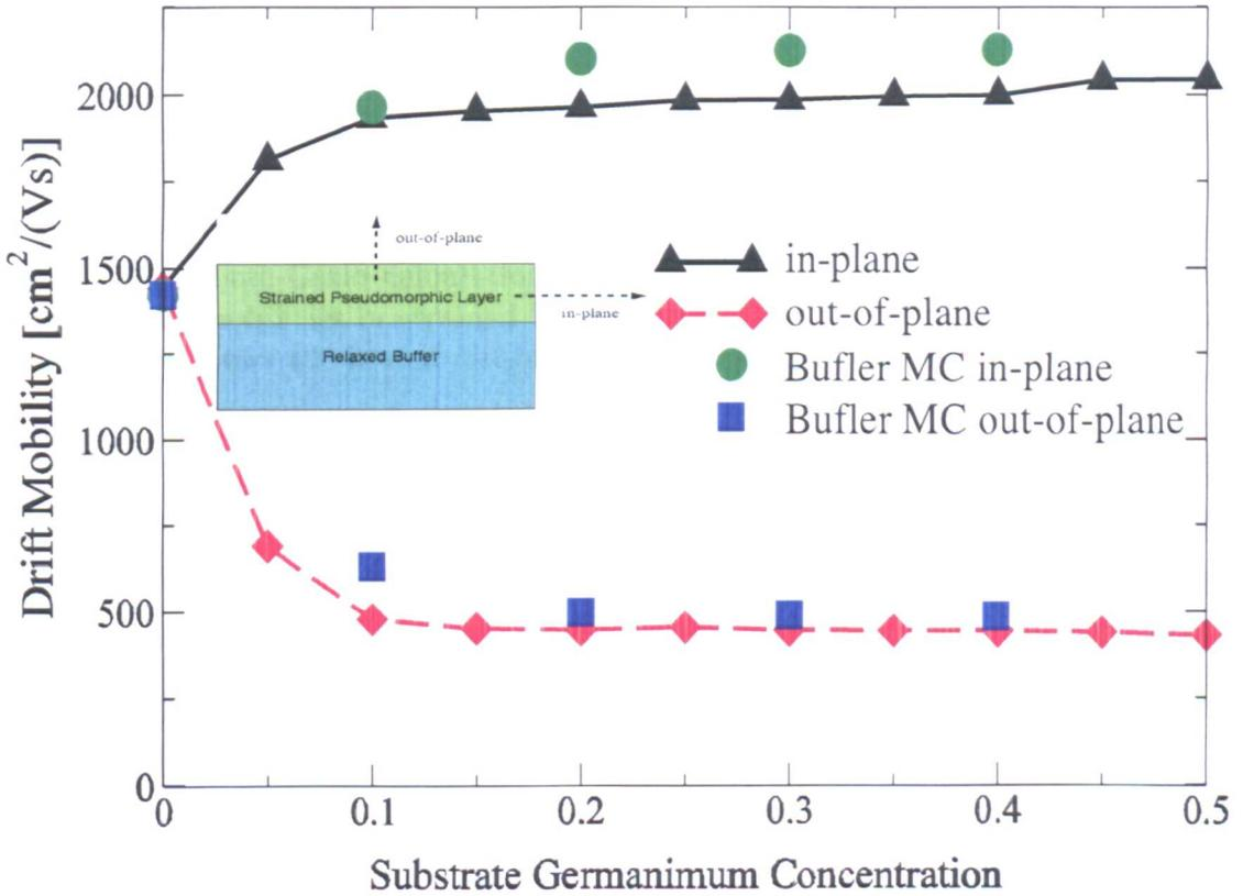
Figure 2.3: Monte-Carlo calculation of low-lateral-field ( $0.25\text{kV/cm}$ ) in- and out-of-plane electron mobilities in strained Si as a function of Ge content within the SiGe buffer. The electron mobilities from Bufler *et al.* [44] are shown for comparison.
