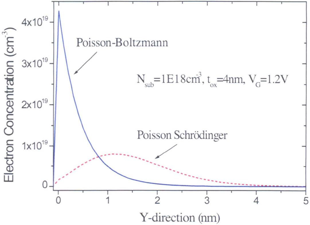
Figure 5.1: Electron distributions solved by 1D Greg-Snyder solver [28] based on the solutions of Poisson-Boltzmann and Poisson-Schrödinger equations
