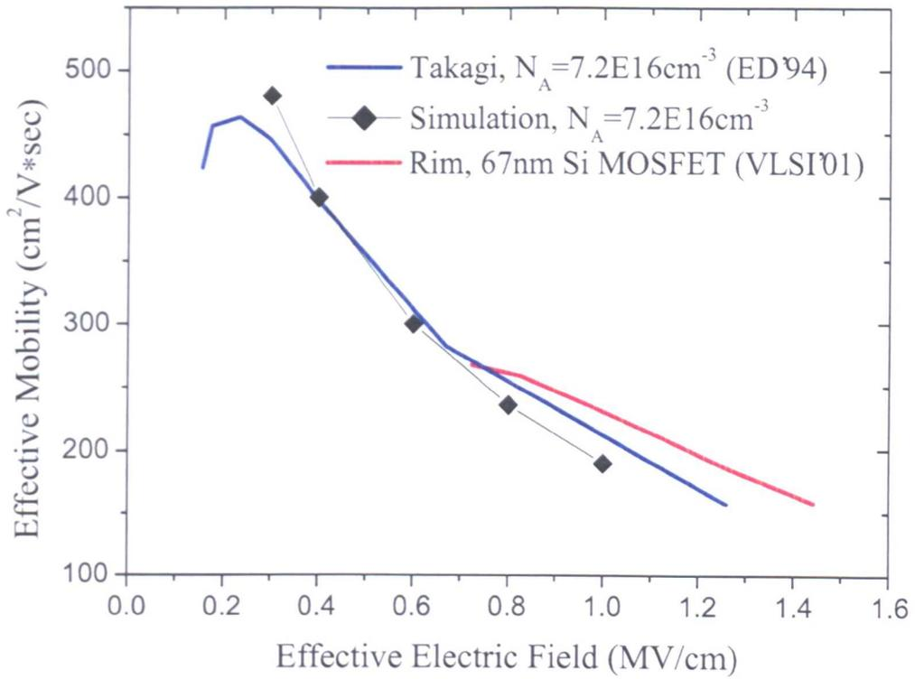
Figure 6.3: Field dependence of the effective electron mobility of bulk Si, compared with data from Takagi *et al.* [171] and Rim *et al.* [31]
