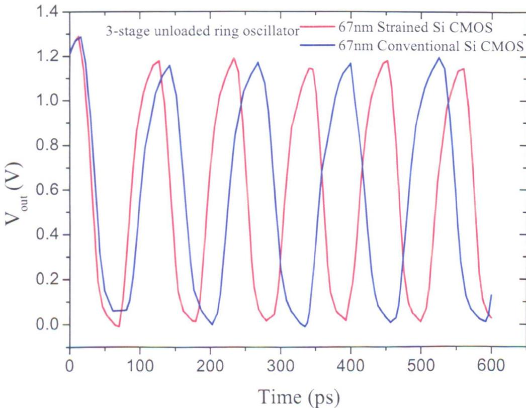
Figure 5.14: Output circuit characteristics for the 67 nm effective gate length Si and strained Si CMOS unloaded 3-stage ring oscillators
