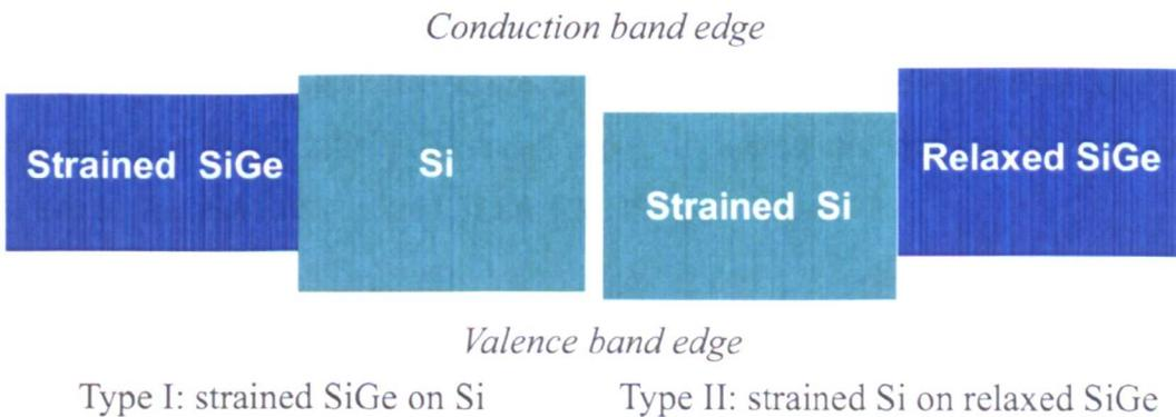
Figure 2.1: The band structures of strained SiGe on unstrained Si and strained Si on relaxed SiGe
