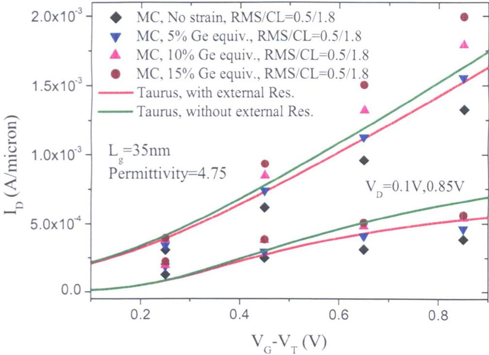
Figure 6.9: Monte Carlo calibrated  $I_D$ - $V_G$  characteristics of 35 nm gate length n-type Si MOSFETs, compared to the data from calibrated Taurus simulator
