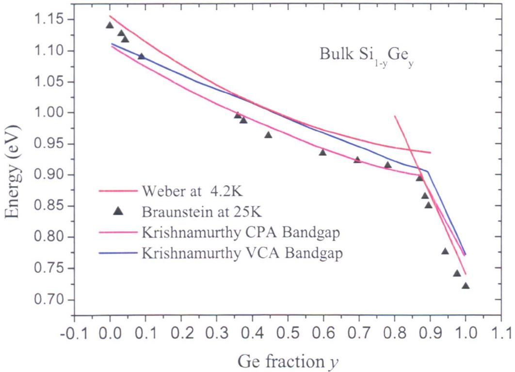
Figure 3.2: Bandgap of bulk  $\text{Si}_{1-y}\text{Ge}_y$  alloy
