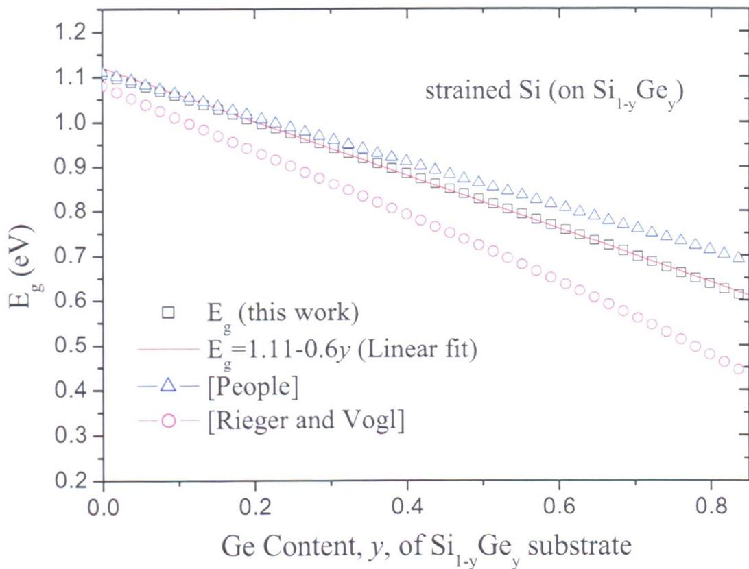
Figure 3.7: Calculated bandgap of strained Si on relaxed  $\text{Si}_{1-y}\text{Ge}_y$  as a function of Ge content  $y$ , compared with the calculations taken from People [14] and Rieger *et al* [121]
