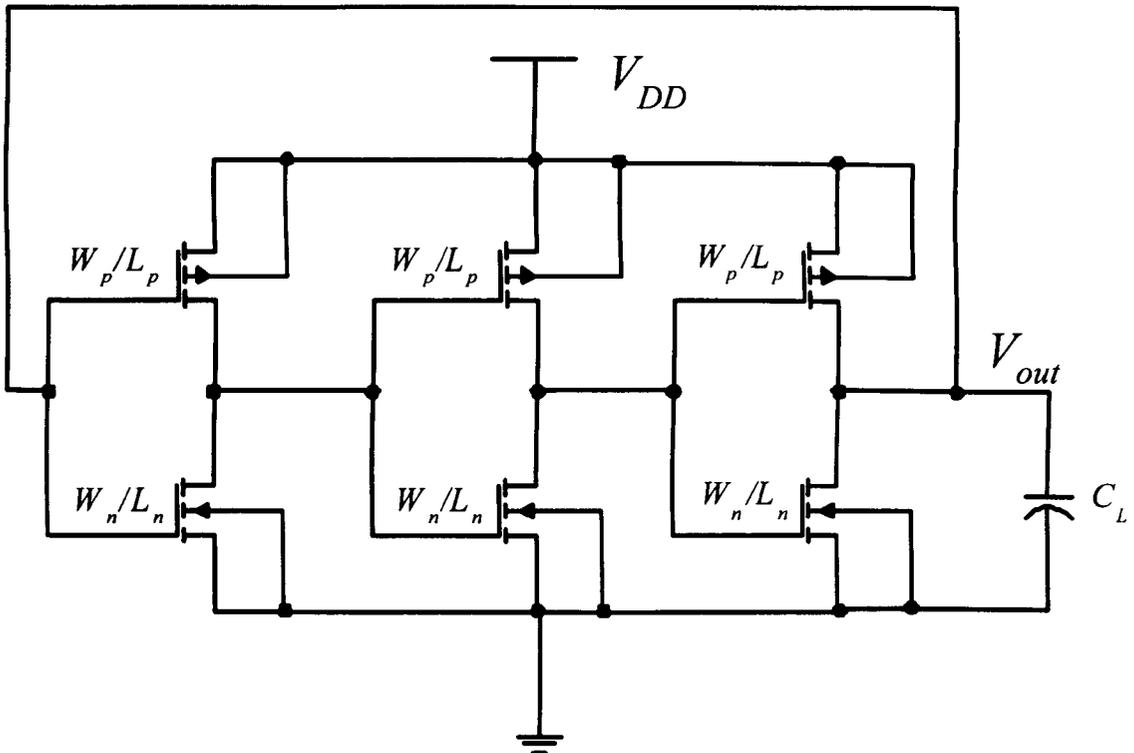
Figure 5.13: Schematic of CMOS 3-stage ring oscillator ( $W_n/W_p=1\mu\text{m}/2\mu\text{m}$ )
