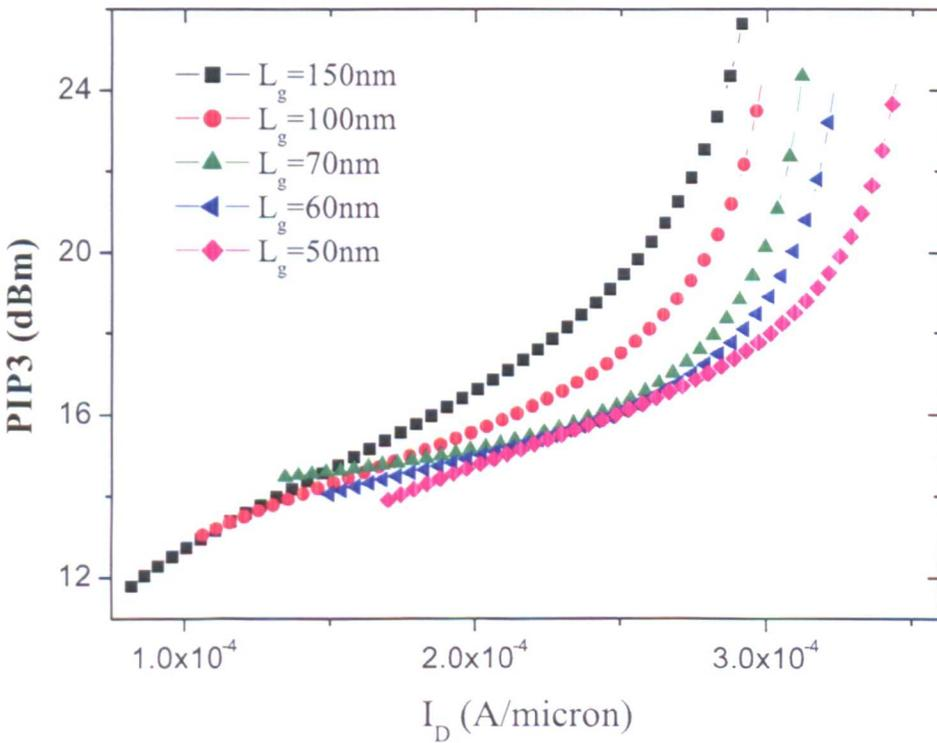
Figure 4.21: The device PIP3 characteristics with different gate length  $L_g$
