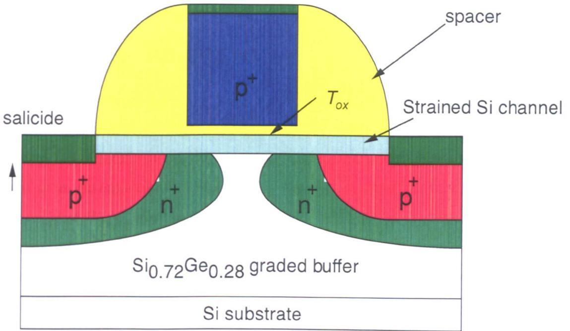
Figure 5.12: Schematic of the simulated p-type well-tempered strained Si MOSFET
