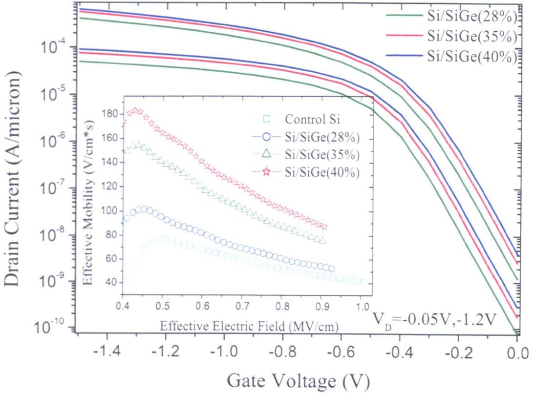
Figure 5.10: Simulated  $I_D$ - $V_G$  characteristics of 90 nm strained Si MOSFETs with different Ge contents in the buffer; the inset is the extracted effective mobility from the simulations
