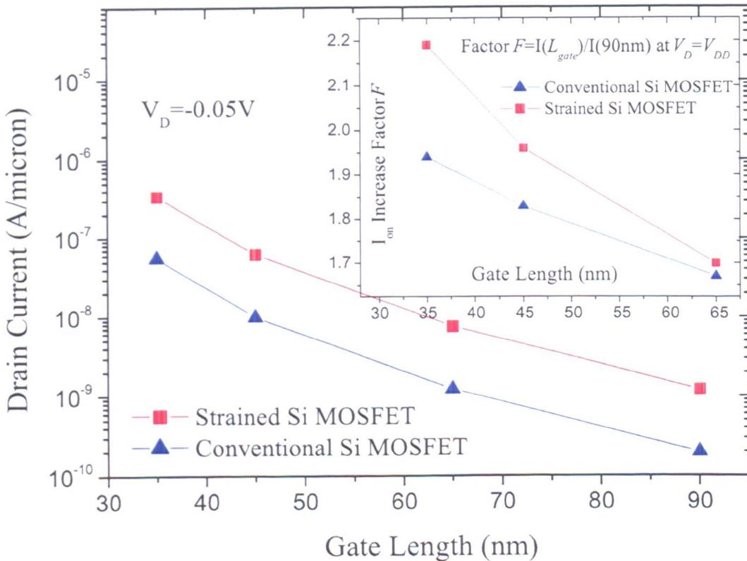
Figure 5.11: The low drain currents of Si control and strained Si MOSFETs as a function of gate length (scaling from 90 nm); the inset shows the high drain on current increase of scaled Si and strained Si MOSFETs as a function of gate length compared to the 90 nm devices
