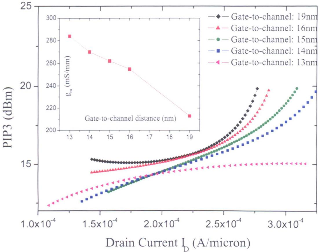
Figure 4.19: The device PIP3 and transconductance  $g_m$  (the inset) characteristics with different gate-to-channel distances
