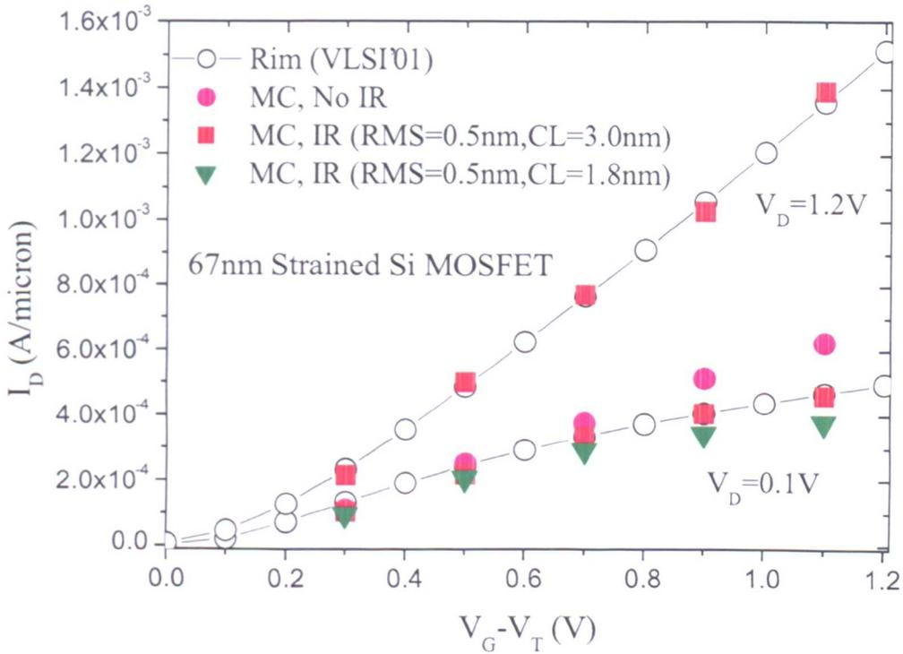
Figure 6.6: Monte Carlo simulator  $I_D$ - $V_G$  characteristics of the 67 nm strained Si MOSFET with and without IR scattering, compared with data from Rim *et al.* [31]
