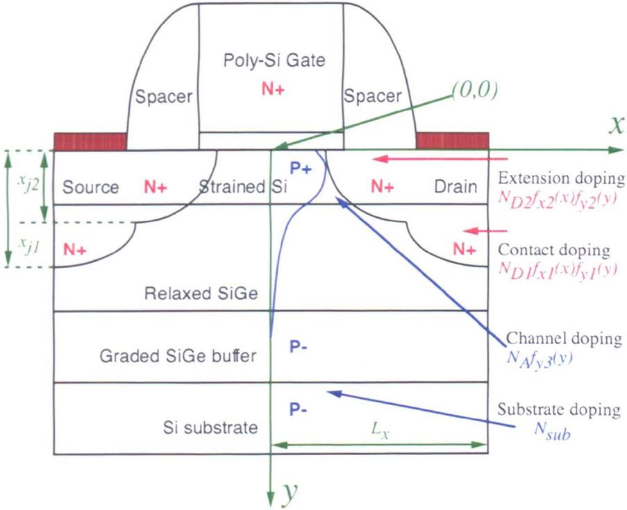
Figure 5.3: Illustration of the doping profiles within the strained Si MOSFET
