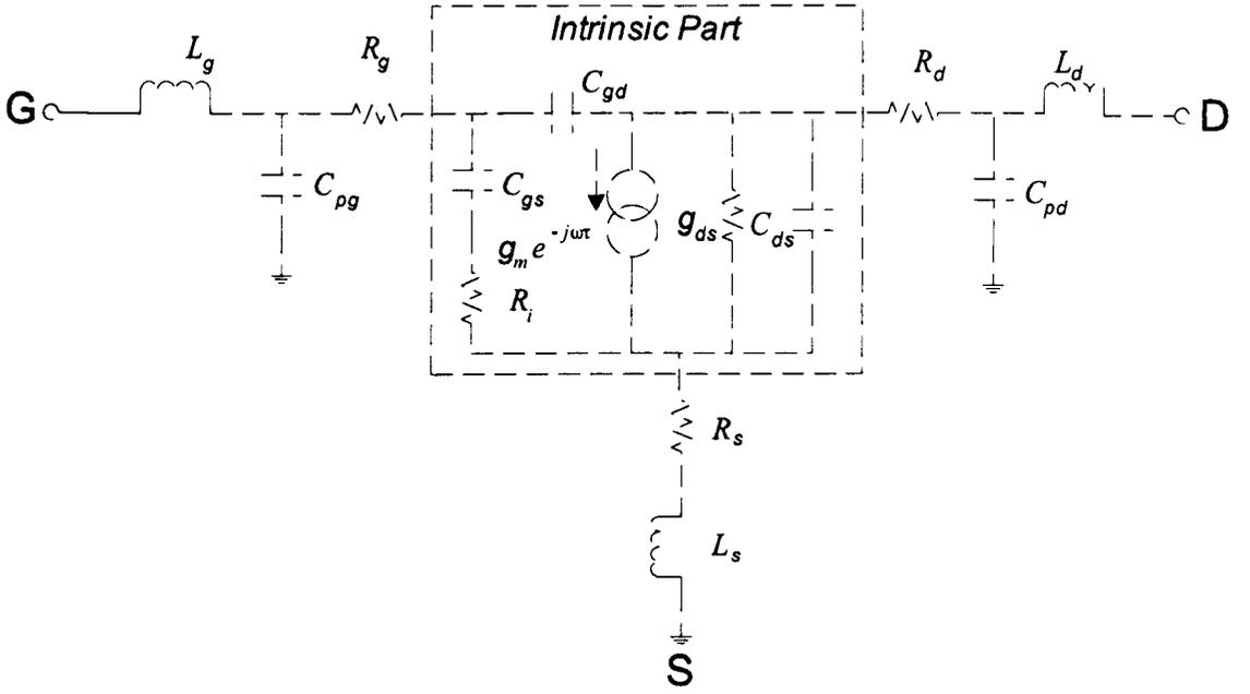
Figure 4.2: Small-signal equivalent circuit of a field effect transistor [149]
