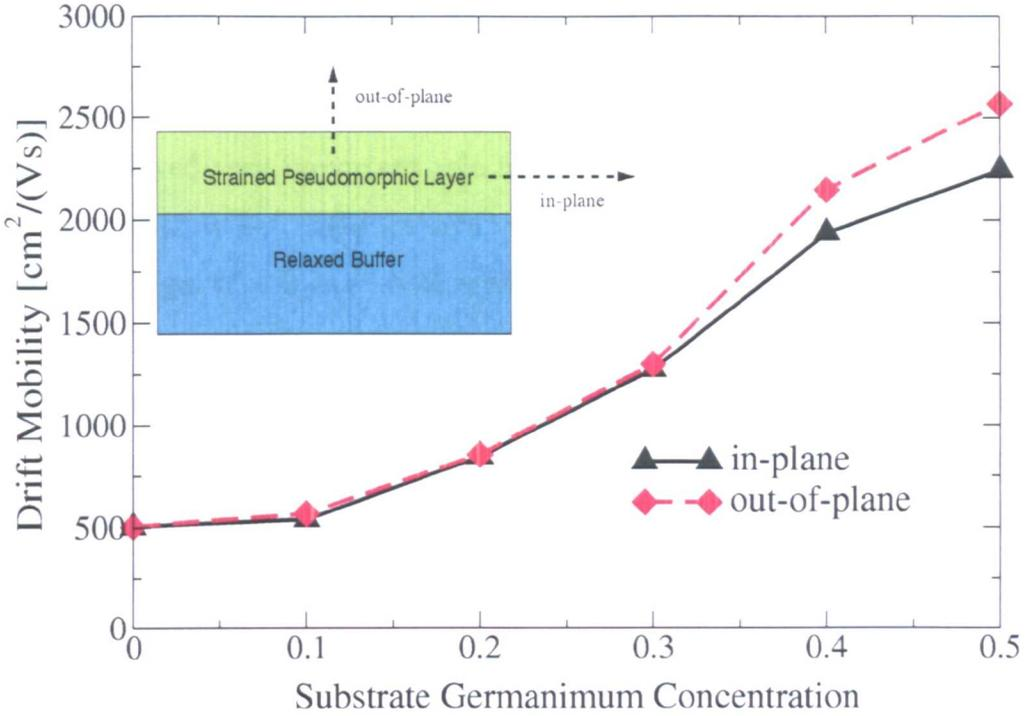
Figure 2.4: Monte-Carlo calculation of low-lateral-field ( $0.25\text{kV/cm}$ ) in- and out-of-plane hole mobilities in strained Si as a function of Ge content within the SiGe buffer. Inset shows the in and out-of-plane directions.
