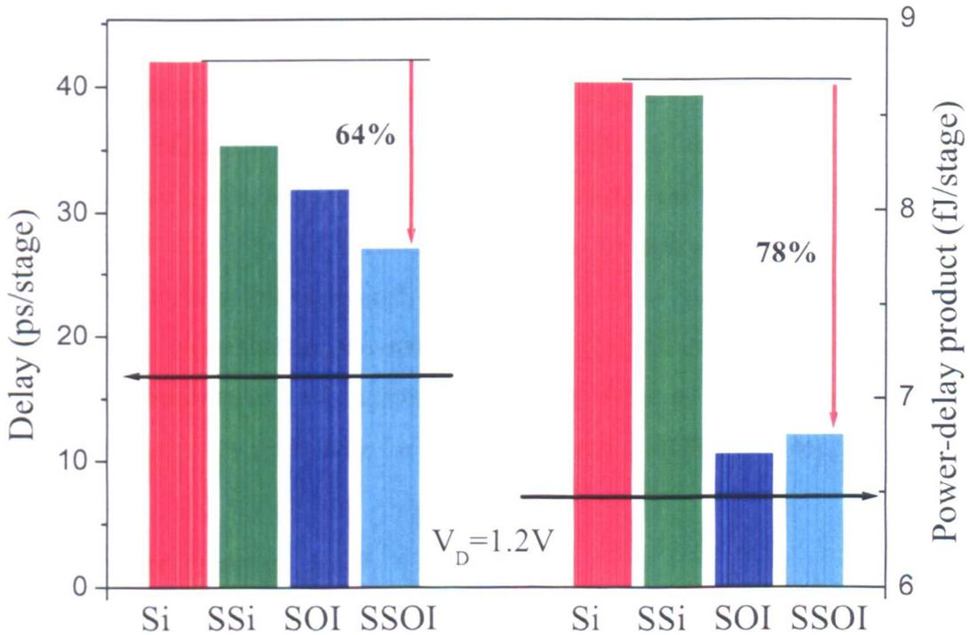
Figure 5.19: Comparisons of the circuit delays and power-delay products of 67 nm conventional Si, strained Si, conventional SOI and strained Si SOI CMOS unloaded 3-stage ring oscillators ( $W_n/W_p=1\mu\text{m}/2\mu\text{m}$ )
