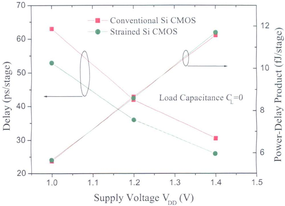
Figure 5.15: Circuit delays and power-delay products versus the supply voltage for the 67 nm Si and strained Si CMOS unloaded 3-stage ring oscillators
