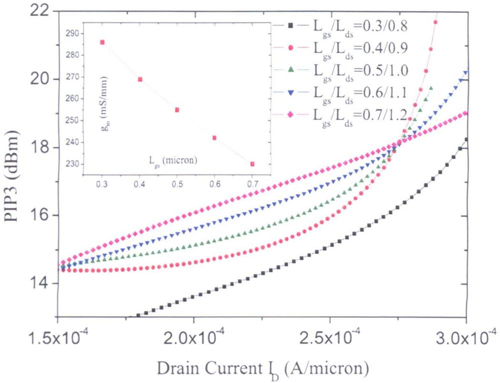
Figure 4.20: The device PIP3 and transconductance  $g_m$  (the inset) characteristics with different gate-to-source distances  $L_{gs}$
