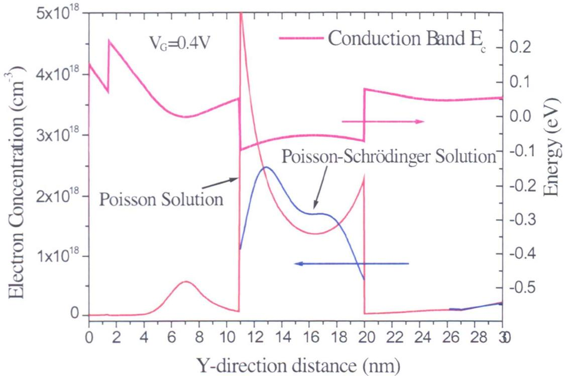
Figure 4.6: 1D band diagram and electron distributions from the 1D Greg-Snyder solver based on the solutions of Poisson's equation and Poisson-Schrödinger
