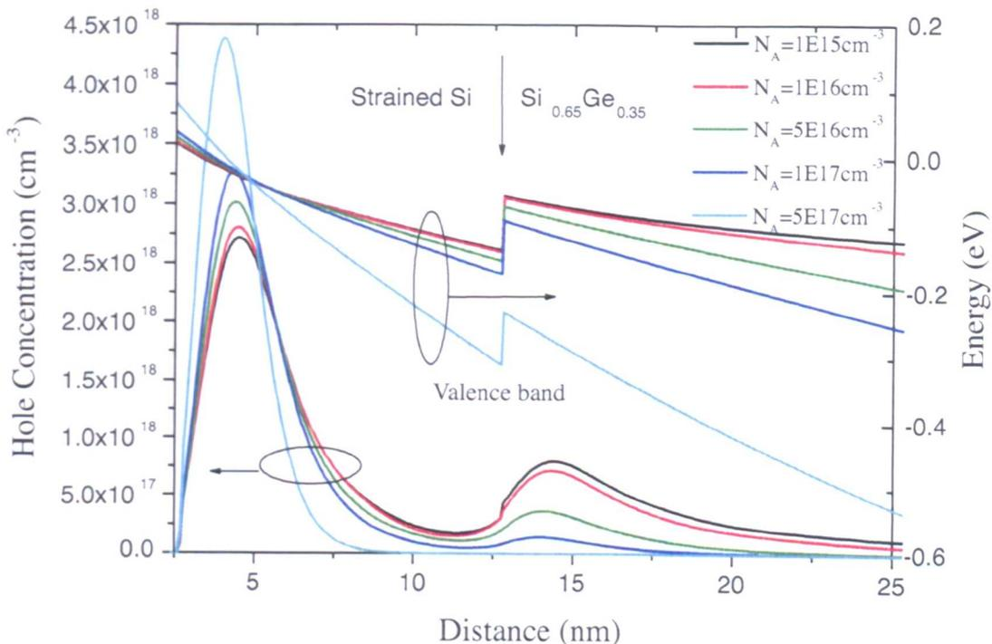
Figure 5.8: Hole distributions and valence band profile in the channel for a range of uniform substrate dopings obtained using 1-D Poisson-Schrödinger solutions (sheet densities in the channel  $n_s = 1 \times 10^{12} \text{ cm}^{-2}$ )
