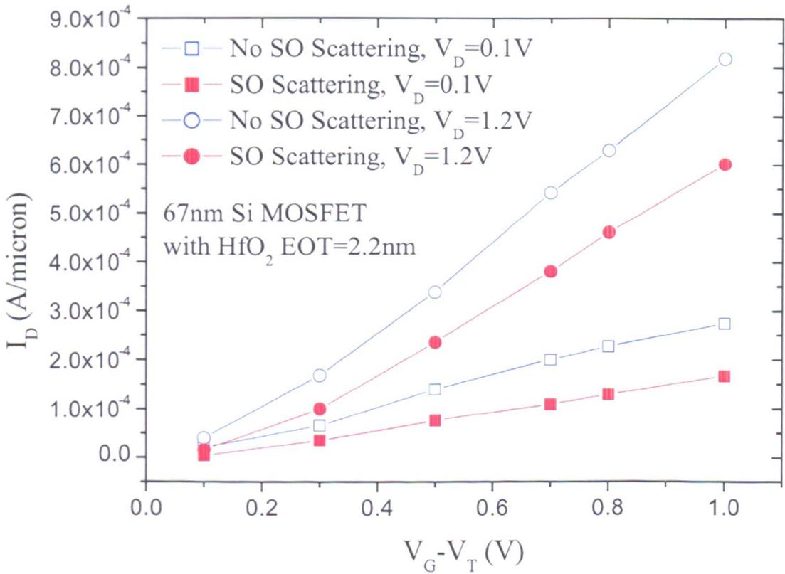
Figure 6.12: Monte Carlo simulated  $I_D-V_G$  characteristics with and without SO phonon scattering of the 67 nm n-type conventional Si MOSFET with HfO<sub>2</sub> gate dielectrics.
