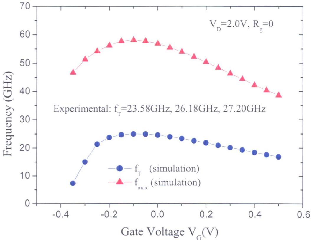
Figure 4.9: Extracted  $f_T$  and  $f_{max}$  characteristics of the  $0.25 \mu\text{m}$  MODFET
