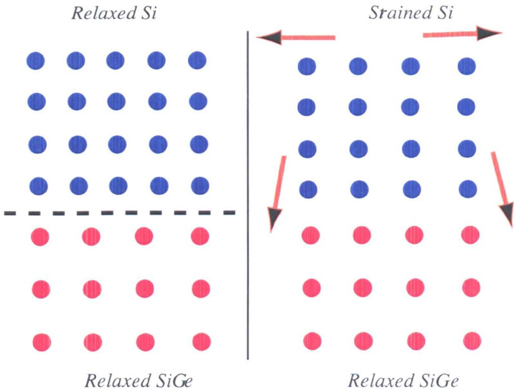
Figure 2.2: Schematics of the Si and SiGe lattice structure. The Si is pseudomorphically grown on the SiGe layer
