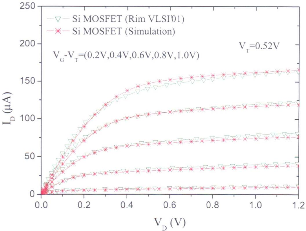
Figure 5.5: Calibrated  $I_D$ - $V_D$  characteristics of the 80 nm gate length Si n-MOSFET
