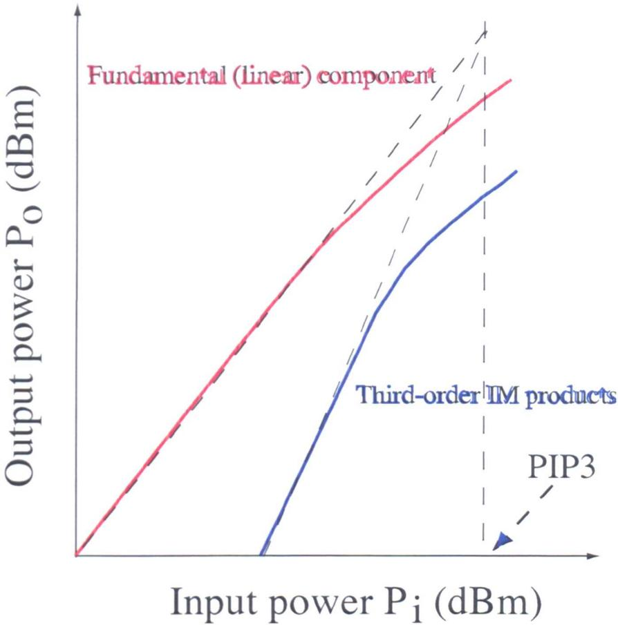
Figure 4.3: Illustration of the definition for PIP3
