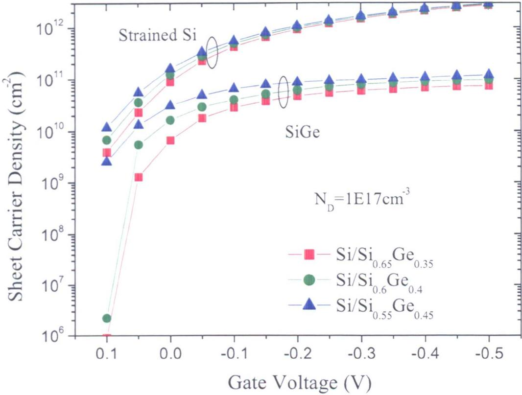
Figure 5.9: Sheet carrier densities in the channel and the SiGe buffer layer with different Ge concentrations as a function of gate voltage obtained using a 1-D Poisson-Schrödinger solver (assuming a uniform substrate doping  $N_D=1 \times 10^{17} \text{ cm}^{-3}$ )
