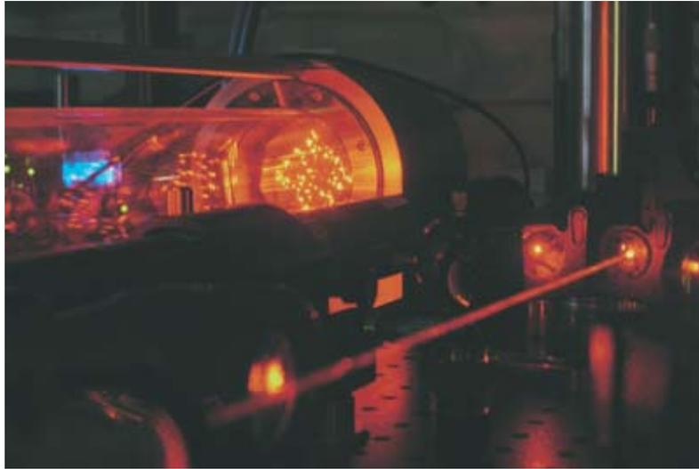
Figure 3.10: The Herriott multipass cell is aligned using a Helium Neon tracer beam. A spot pattern is visible on each of the cell mirrors.
