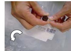
5. Holding the tap nozzle as shown, open all 12 bags by turning taps anti-clockwise (2 turns)
