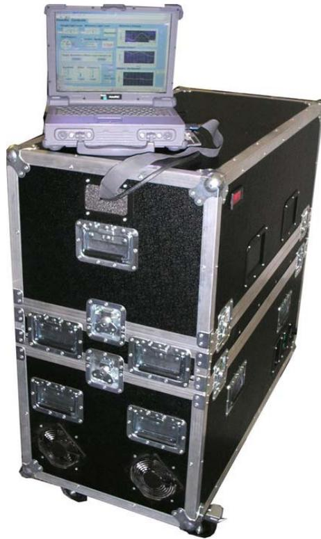
Figure 3.1: Photograph of the ultra-sensitive, real-time portable ethane spectroscopy system. The self-contained instrument has dimensions 1 m x 0.5 m x 1 m (L x W x H)
