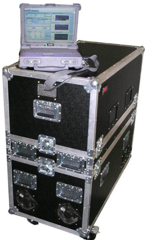
**Figure 1.** The ultra-sensitive, real-time ethane spectroscopy system developed at the University of Glasgow. The instrument with dimensions 1 m × 0.5 m × 1 m ( $L \times W \times H$ ) is completely self-contained.
