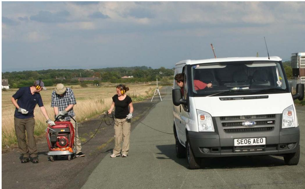
Figure 5.1: The portable instrument was housed in a van and the generator was transported on a trolley. Ethane concentration measurements were made via a sample inlet tube mounted at the top of the vehicle. Measurements of wind speed and direction were made using an anemometer (shown in the distance).
