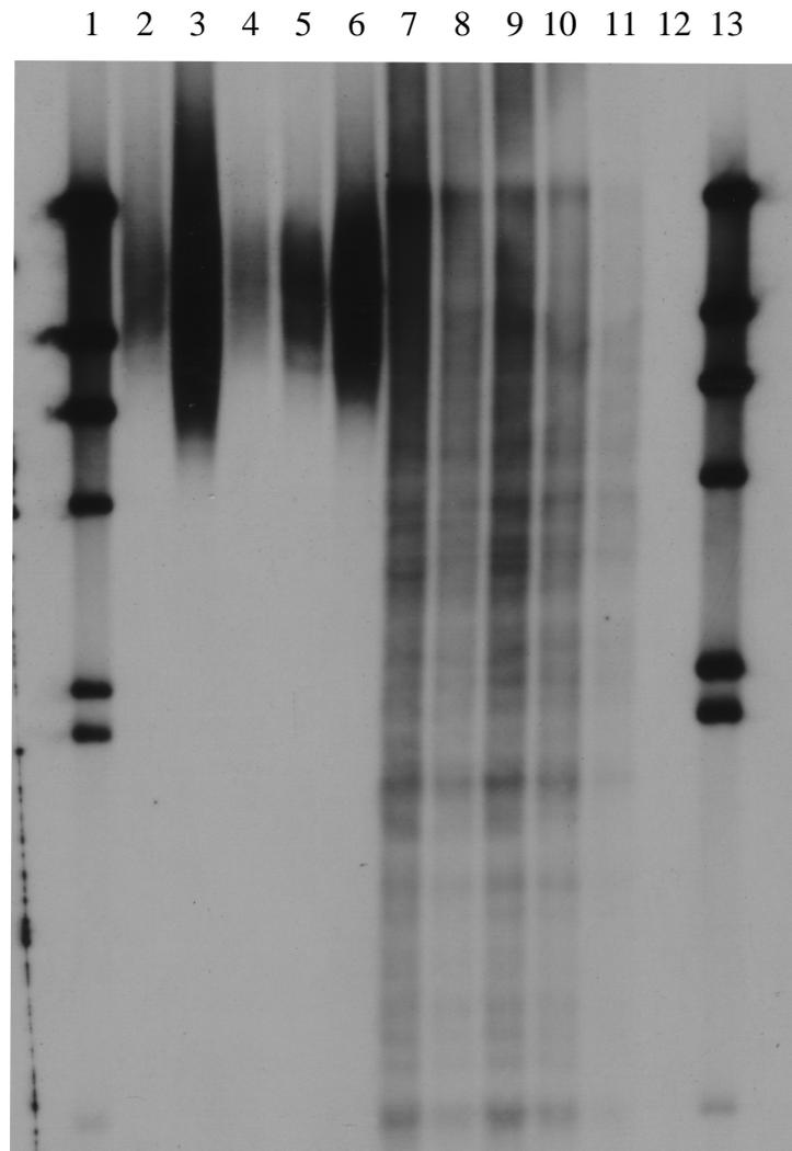
**Figure 6.3:** Representative blue-footed booby TRF gel produced by constant-field gel electrophoresis, with DNA extracted using a DNeasy Blood and Tissue Kit. Lanes 7-11 contain blue-footed booby samples, with substantial banding present in the TRF smear. For comparison, lanes 2-6 contain TRF smears from European shag DNA; these smears are clear with no obvious banding. Lanes 1 and 13 contain markers, lane 12 is blank.
