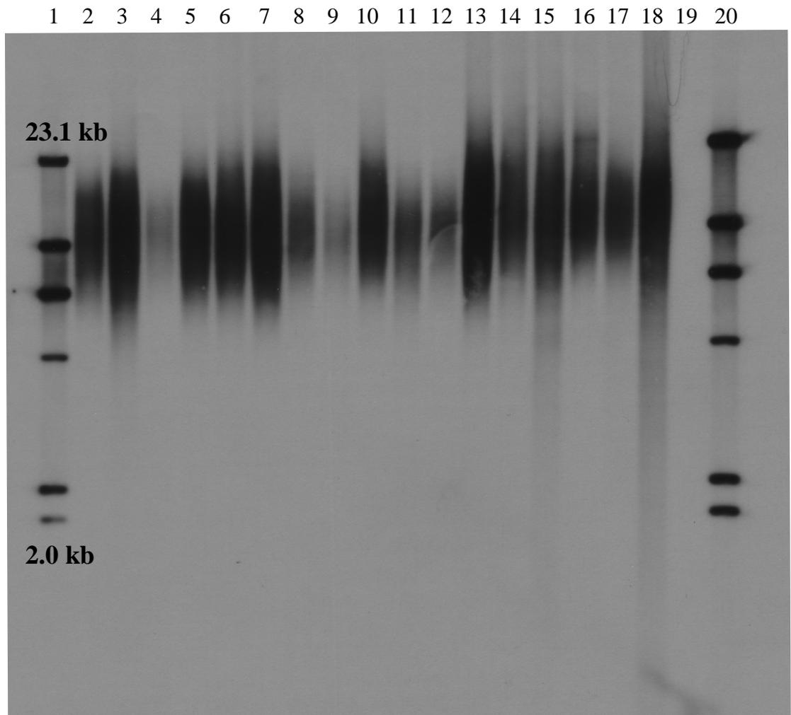
**Fig. 1.6:** Example of an autoradiograph produced by TRF analysis (with constant field gel electrophoresis). Lanes 1 and 20 contain a molecular size marker, lanes 2 – 19 each represent a different sample (lane 19 is blank). Increased intensity of the smear at a given molecular weight means there are more telomere fragments of this size in the cell population.
