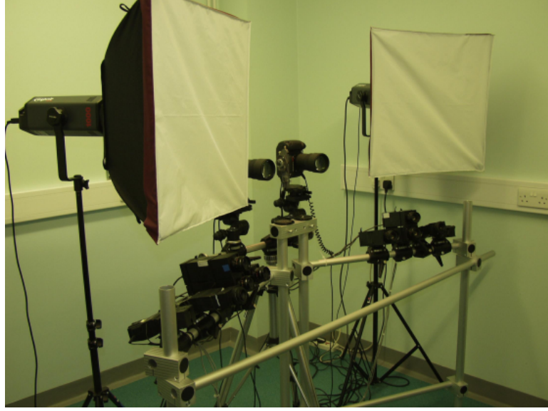
Figure 3.3: Single pod stereo-pair system with two cameras mounted on a rig, along with two portable flash units.
