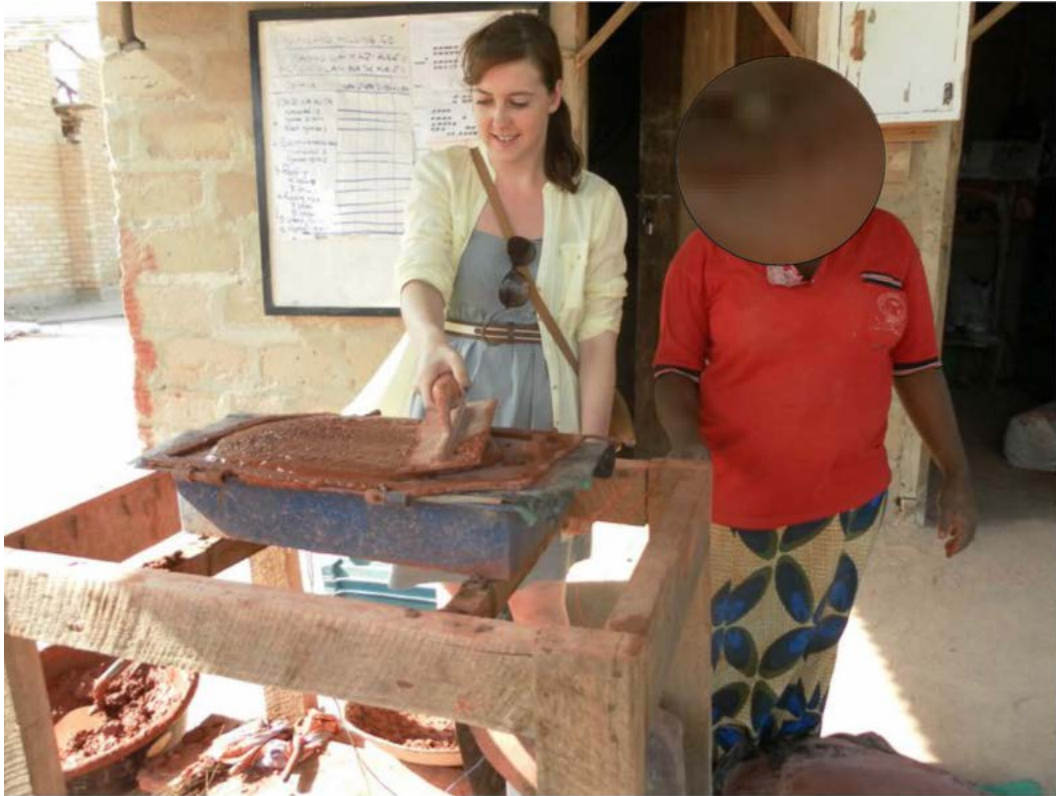
Figure 4.7: Making roof tiles in Chamazi (fieldwork photograph)
