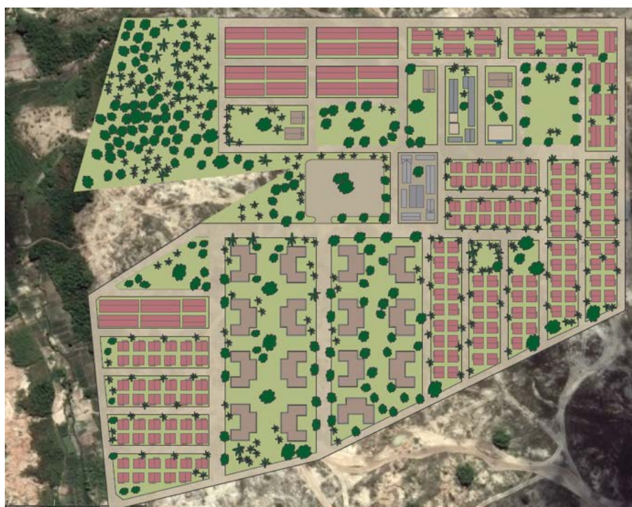
Figure 8.2: Plans for the finished Chamazi resettlement site including housing units, open space, services, commercial space, light industries, market and bus stand (Source: Ricke, 2012).
