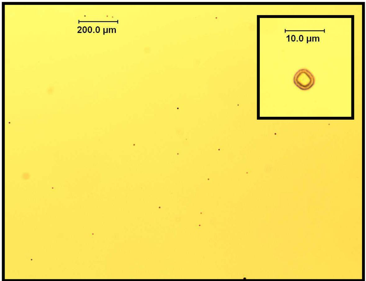
**Figure 6.10:** Optical microscope image of surface of QCSE wafer showing pits. Inset shows single pit at higher magnification.
