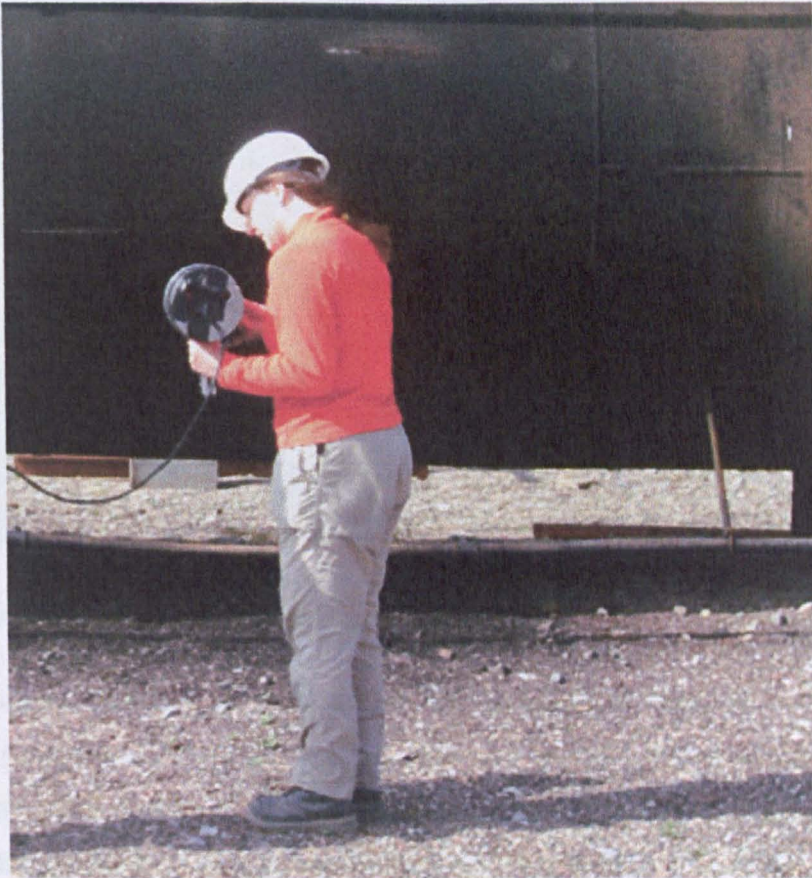
Figure 6.9: Carbon coated storage tank used to test the sensitivity of the instrument under low backscattered-light conditions
