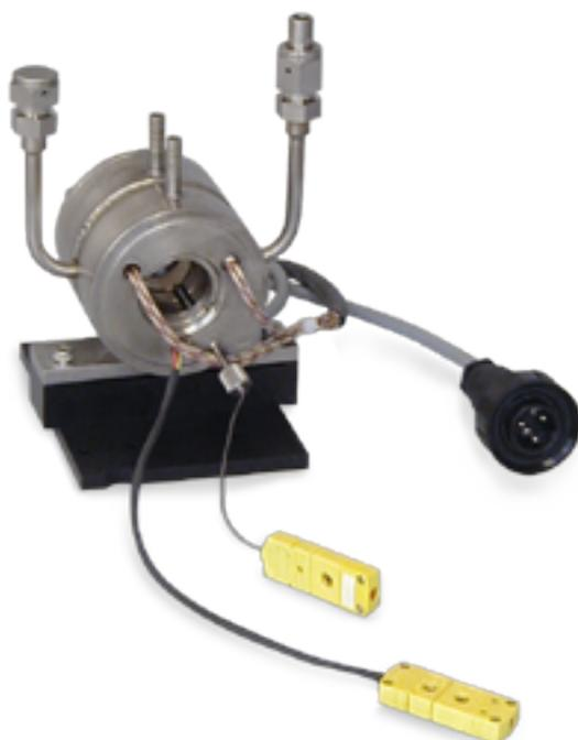
Figure 2.4: Picture of the Harrick High Temperature transmission IR cell
