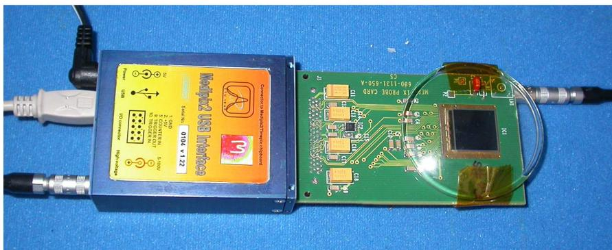
Figure 5.4: Medipix2 chipboard connected to IEAP's USB interface.
