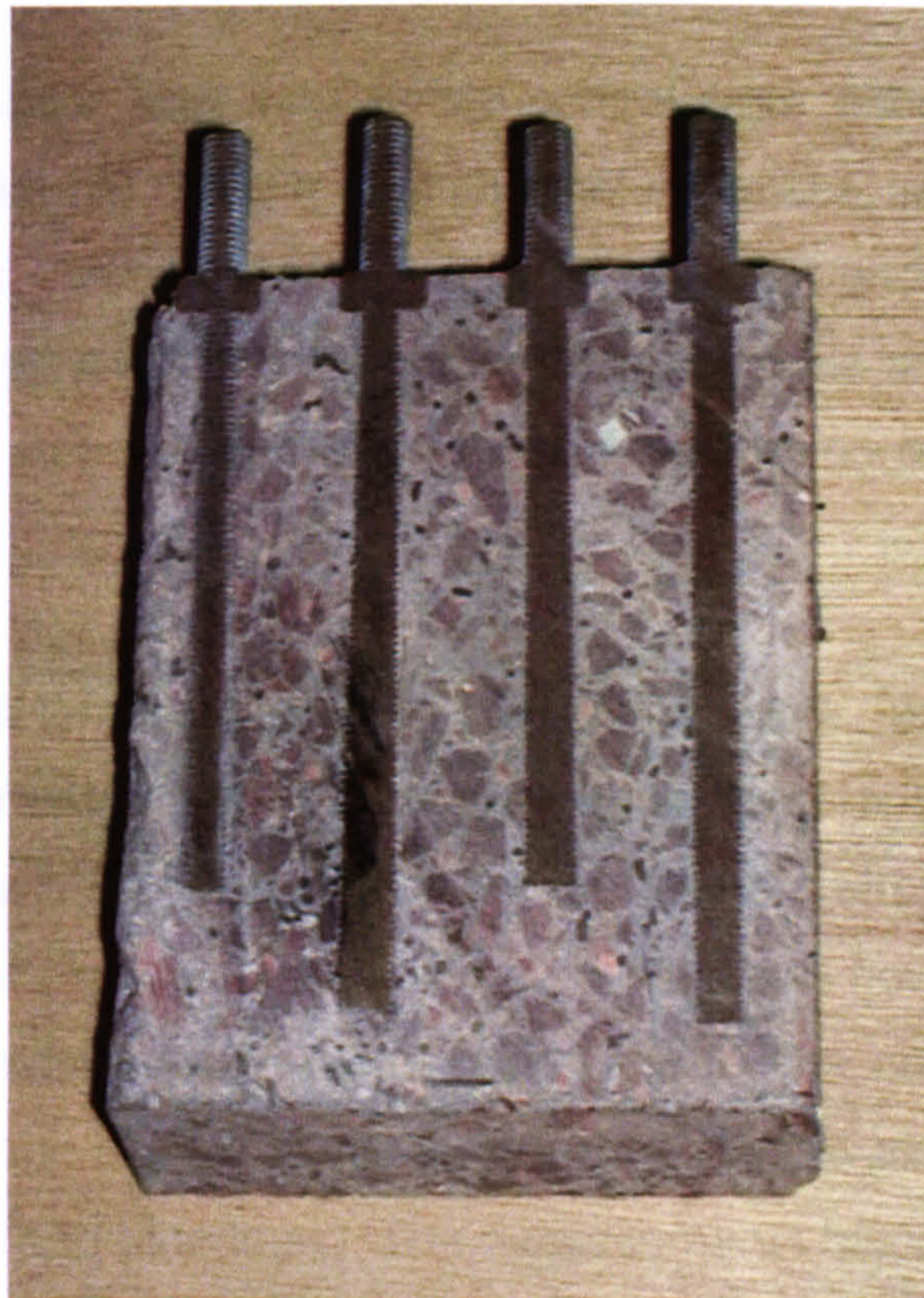
Figure 3.16 Cut through a plane where the threaded rods had been cast into a specimen
