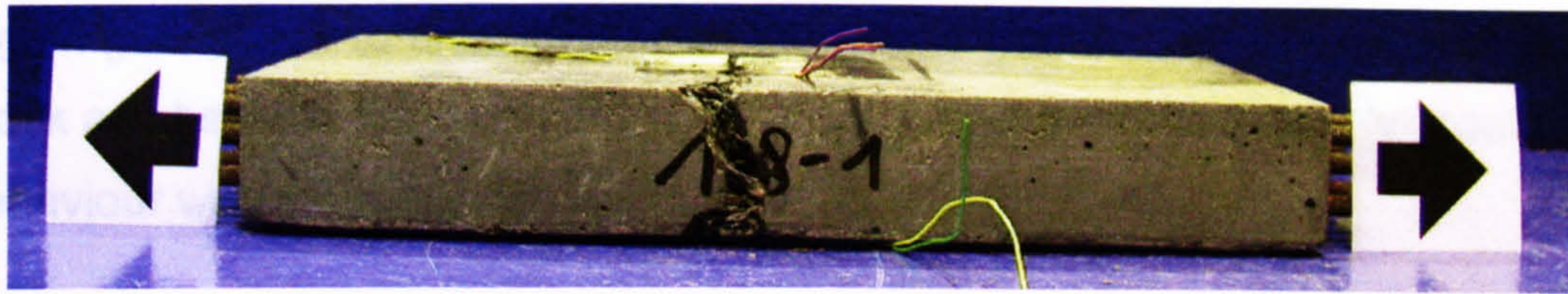
Figure 6.28 Failure mode of SFRHPC ( V_f = 2\% , aspect ratio l/d = 65 , fibre length l = 35 mm) specimen of the compression-tension series in uniaxial tension
