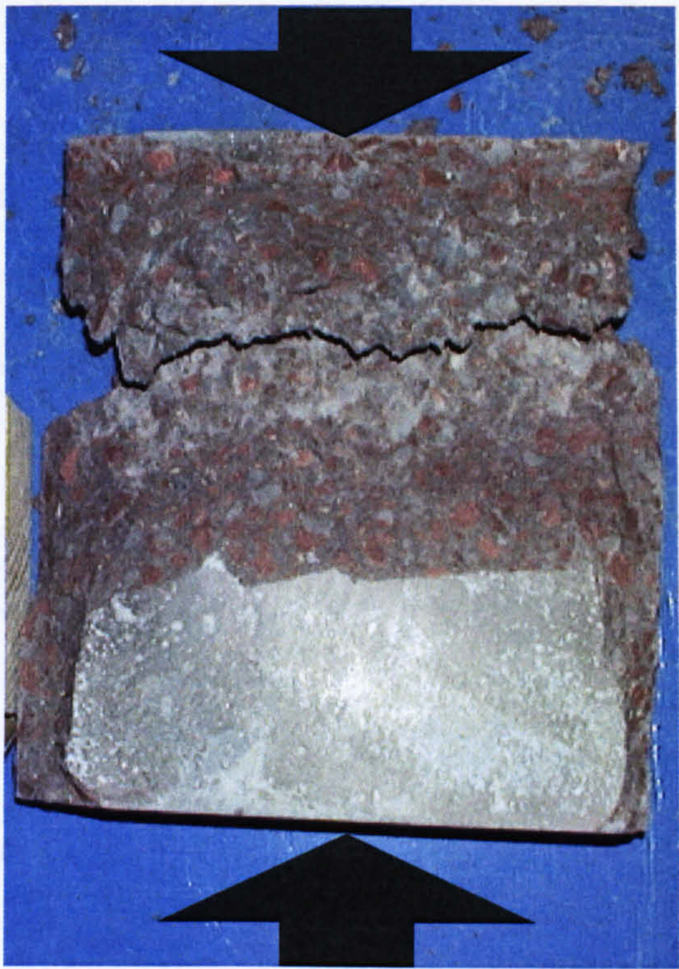
Figure 6.1 Failure mode of plain HPC specimen of the compression-compression series in uniaxial compression
