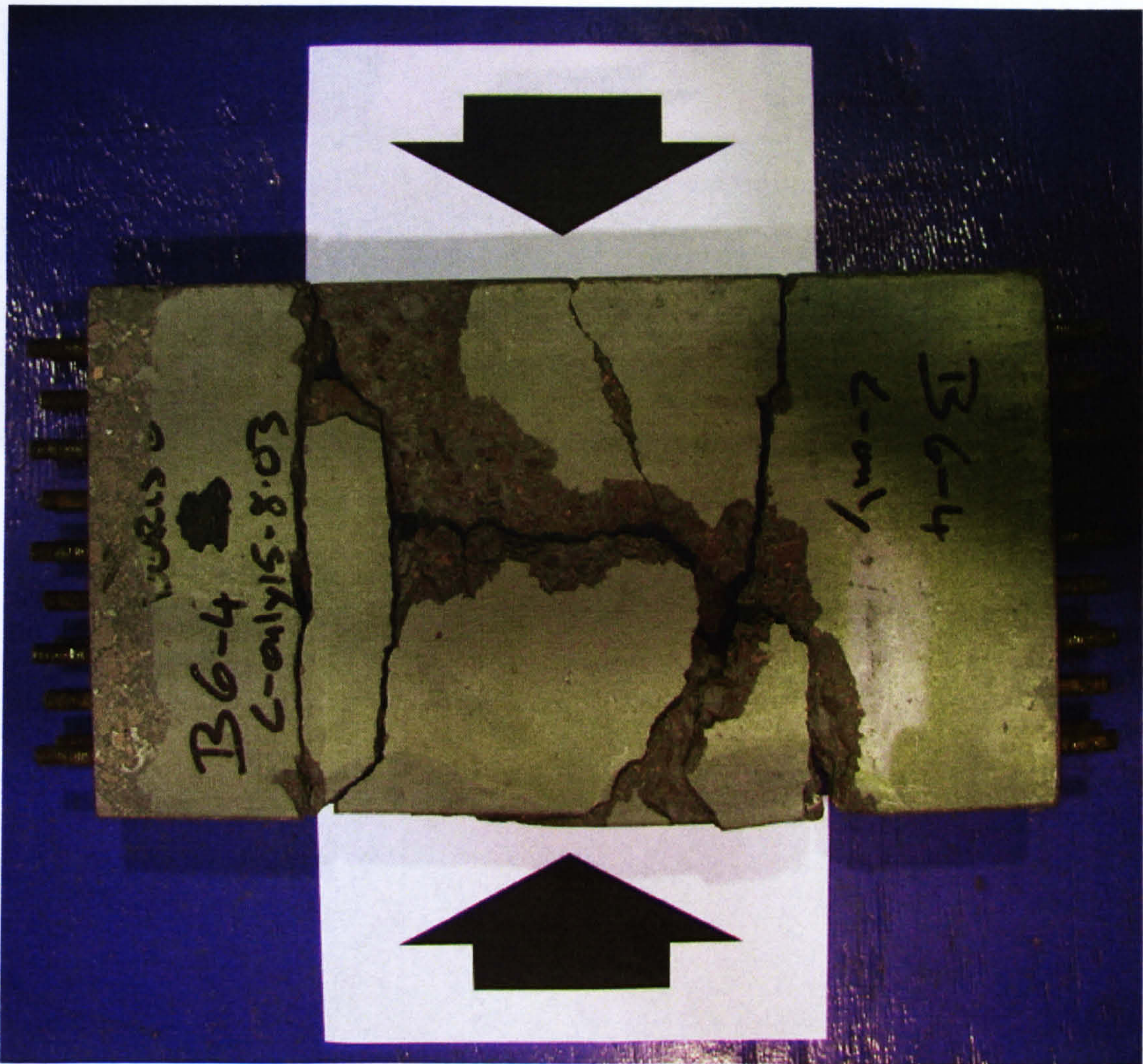
Figure 6.2 Failure mode of plain HPC specimen of the compression-tension series in uniaxial compression
