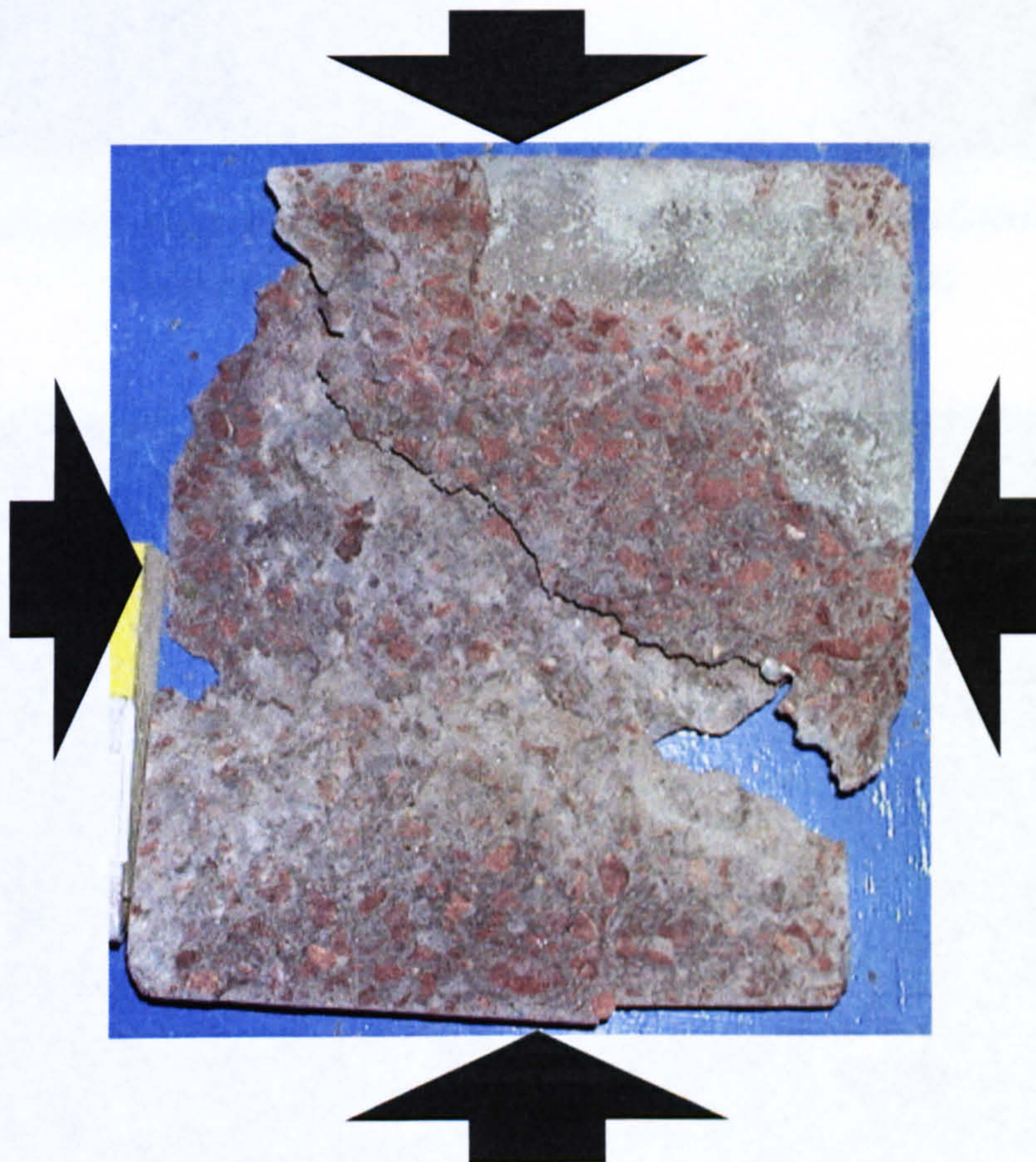
Figure 6.5 Failure mode of plain HPC specimen of the compression-compression series in biaxial compression ( \sigma_2/\sigma_3 = 1 )
