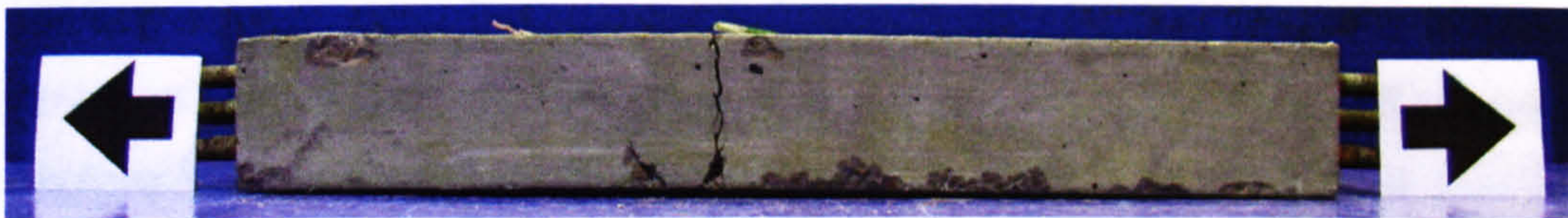
Figure 6.26 Failure mode of SFRHPC ( V_f = 1\% , aspect ratio l/d = 65 , fibre length l = 35 mm) specimen of the compression-tension series in uniaxial tension
