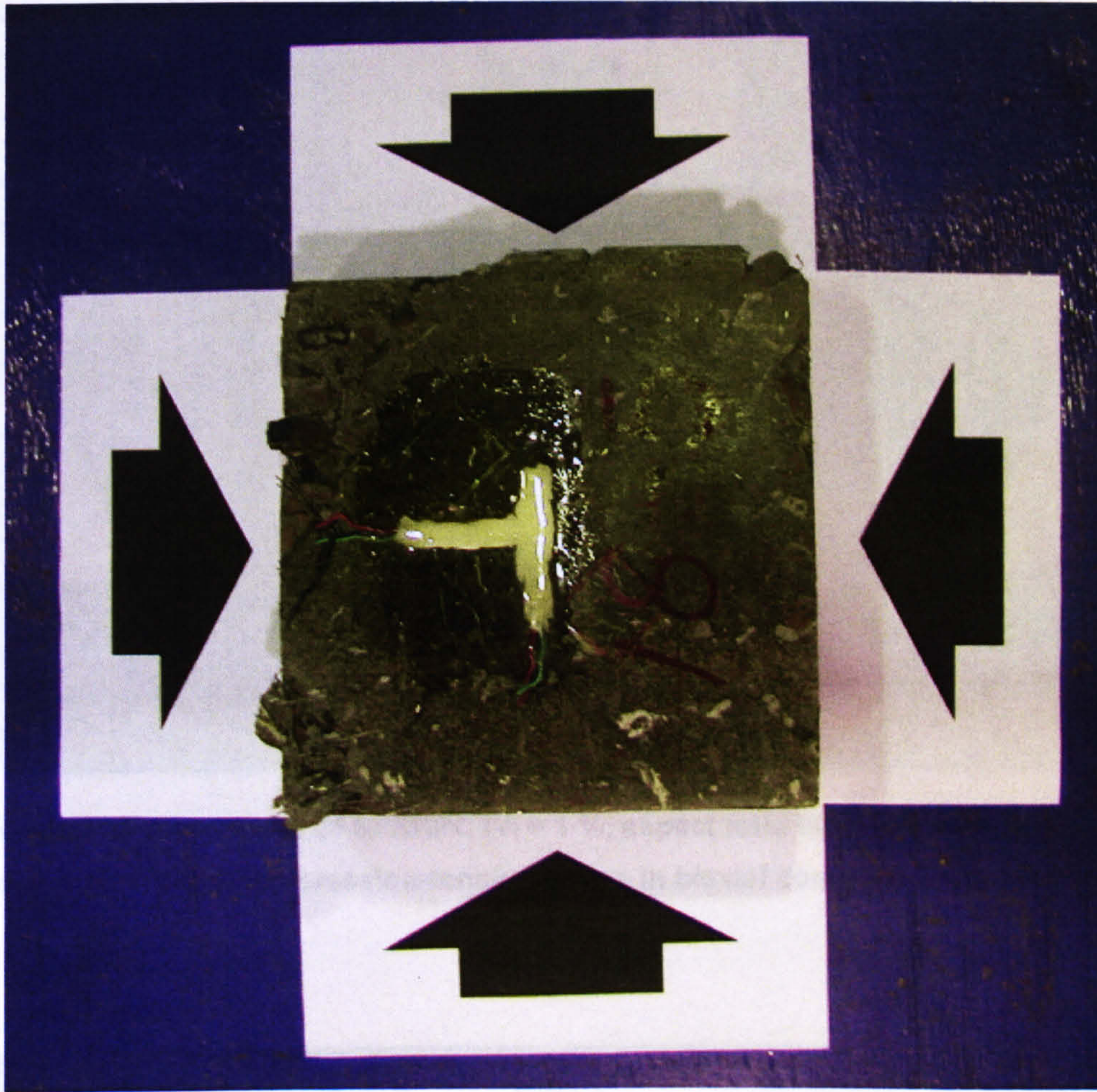
Figure 6.19 Failure mode of SFRHPC ( V_f = 2\% , aspect ratio l/d = 65 , fibre length l = 35 mm) specimen of the compression-compression series in biaxial compression ( \sigma_2/\sigma_3 = 1 ) tested with the solid steel block platen system
