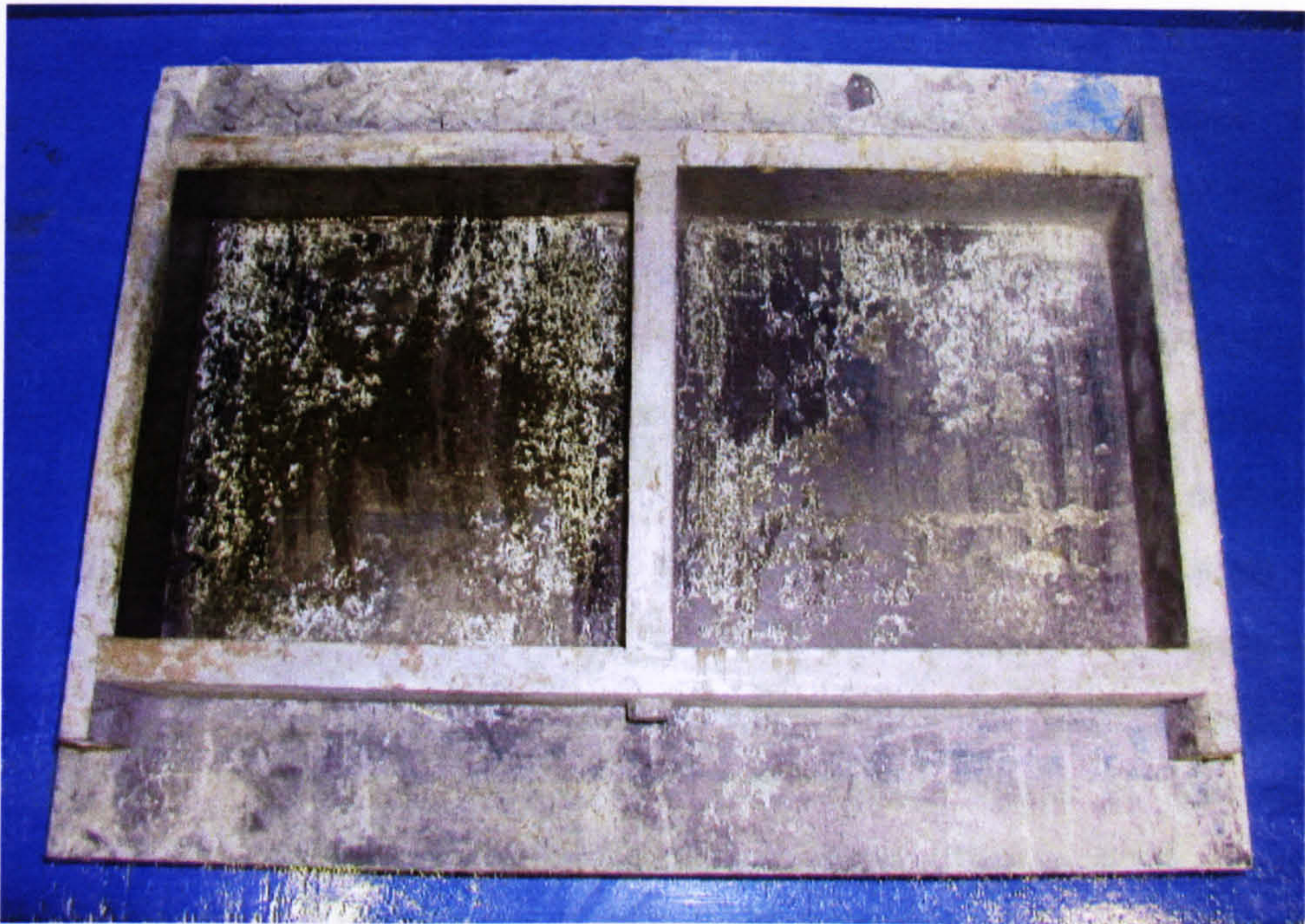
Figure 3.26 Steel moulds for two compression-compression specimens
