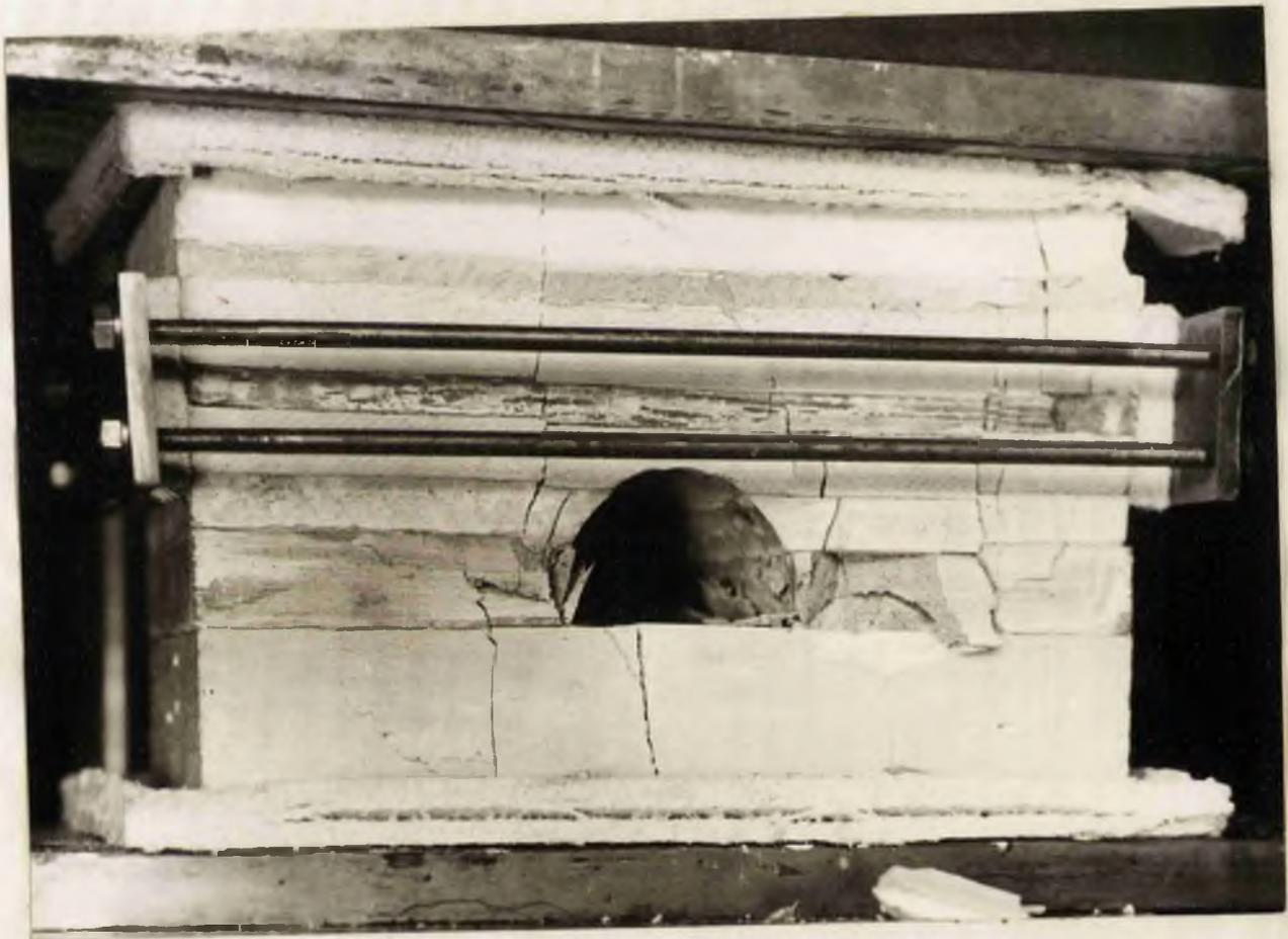
Applied load 425 lb./in.<sup>2</sup>. Note particularly the marked deterioration of the roadsides and the position of the major fractures,  $\frac{1}{2}$  inch from the sides of the excavation, forming the familiar arched-shaped zone over the roadway. The pavement heave has also become more pronounced.
