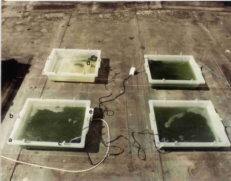
Plate 5: Outdoor Miniponds: (a) polypropylene tray (b) perspex lid (c) bolt (d) mixer (e) mixer control (f) temperature probe
