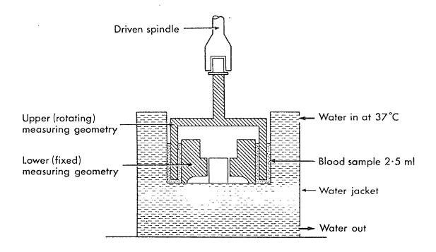
Figure 2 Diagram of the Measuring Geometry of the Deer Rheometer
