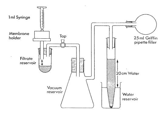
Figure 7 Diagrammatic Representation of the Apparatus for Measuring the Erythrocyte Deformability Index
