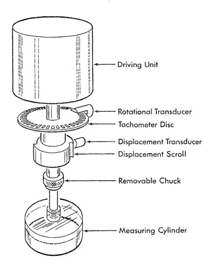
Figure 3 Diagram of the Displacement and Angular
