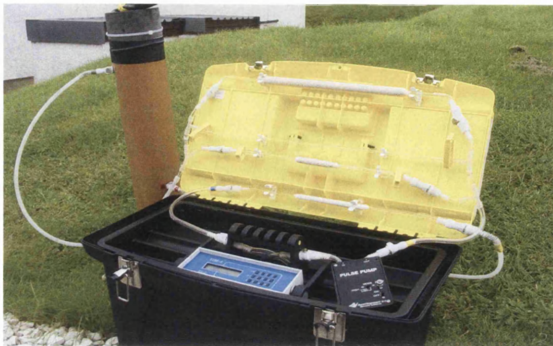
Figure 2.2 - The molecular sieve sampling system in field operation. The chamber is for demonstration purposes only.
