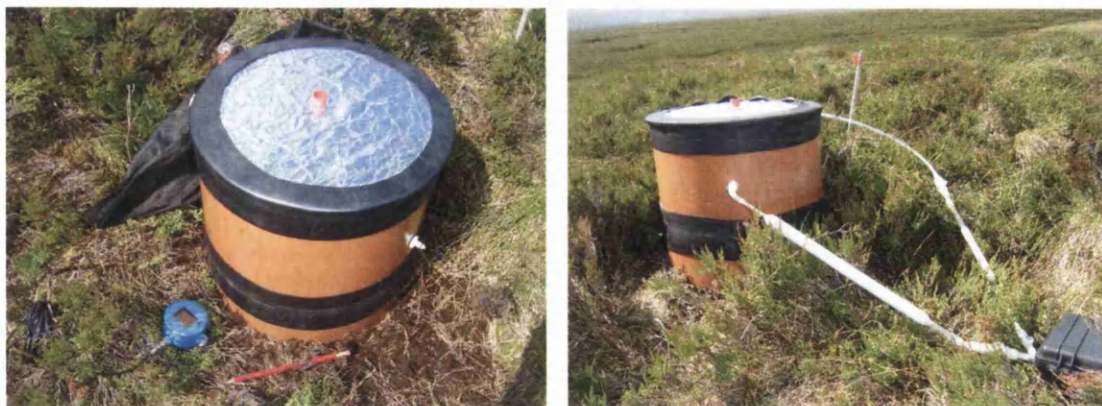
Figure 5.2 – Photographs illustrating the respiration chamber design (LHS) and the scrubbing system used to remove atmospheric CO 2 from all chambers before capture of respired CO 2 (RHS).
