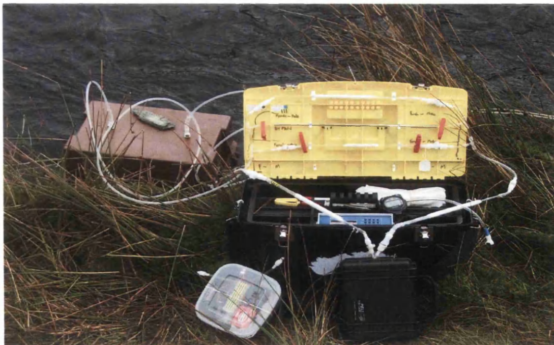
Figure 2.10 - Photograph of \text{MS}^3 attached to a floating chamber (Billett et al. , 2006), used to capture \text{CO}_2 evasion from a peatland stream in the Upper Conwy, Wales, February 2006. Photograph supplied courtesy of Dr. Mike Billett, CEH Edinburgh, UK.
