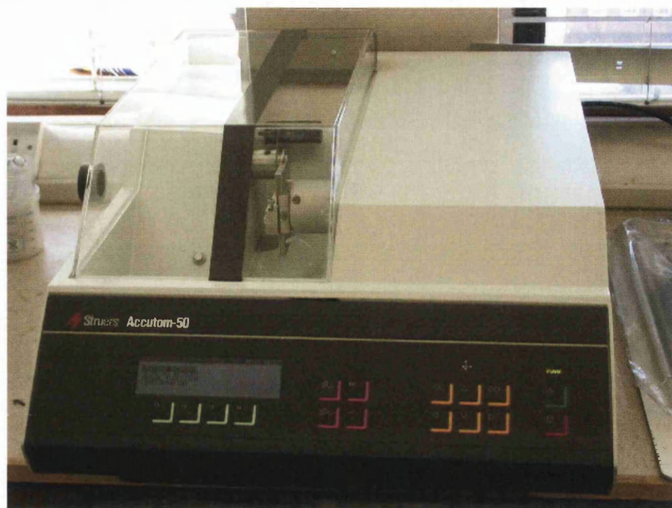
Figure 7 - Accutom-50 machine used to cut the tooth blocks into 200 \mu\text{m} sections
