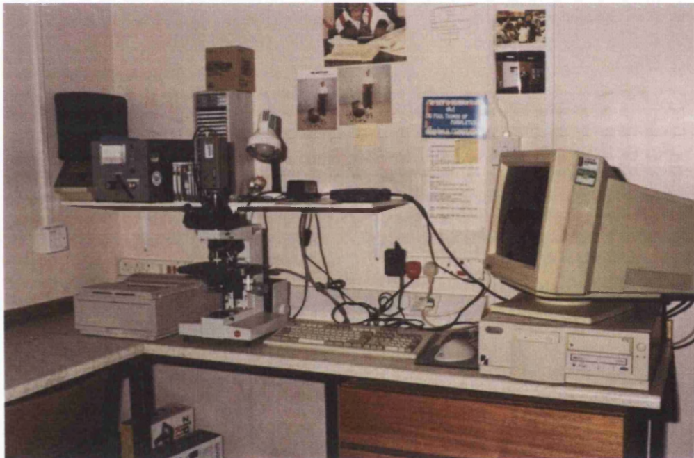
Figure 9 - Photograph of image analysis hardware used to measure the mineral content of the microradiographs in TMR
