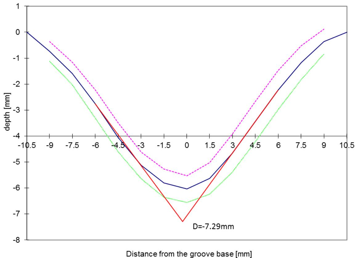
Figure 5.14. Diagram of Govan 14 sample 8 Groove Profile, demonstrating how variable D is calculated (adapted from Kitzler Åhfeldt (2002b, 8a)).
