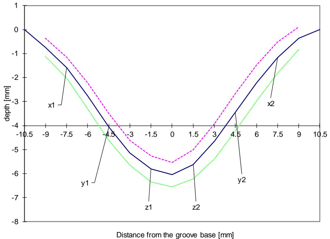
**Figure 5.12.** Diagram of Govan 14 sample 8 Groove Profile with labelled measurements required to calculate variables AvgX, AvgY, and AvgZ, adapted from Laila Kitzler Åhfeldt (2002, 8a).
