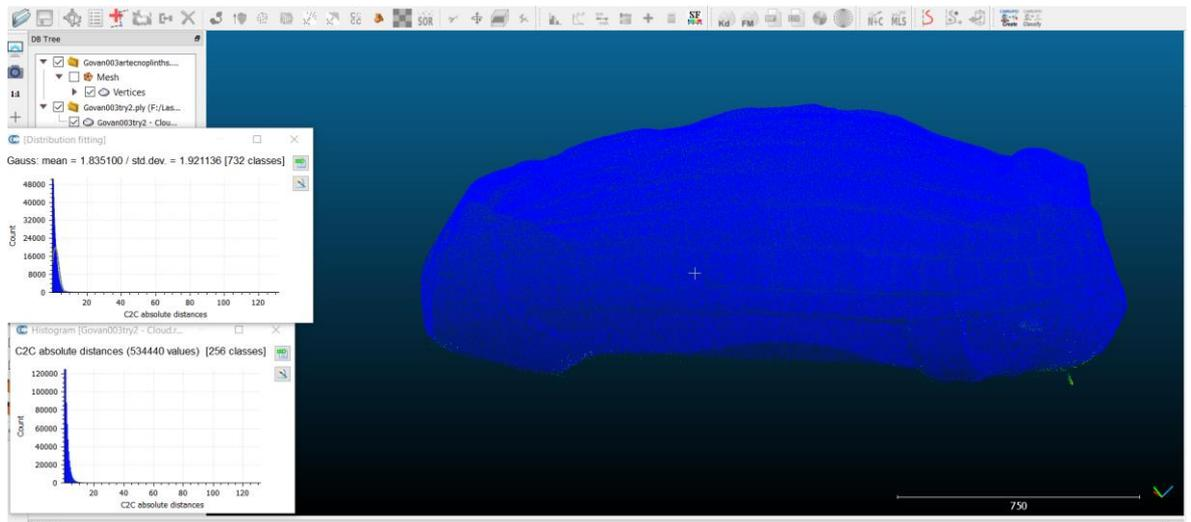
**Figure 5.2.** Point cloud of Govan 3 produced by laser scanning compared to that produced by WLS. A virtually identical result to the previous comparison, there is a 2-3 mm distance between corresponding points when the two point clouds are compared.
