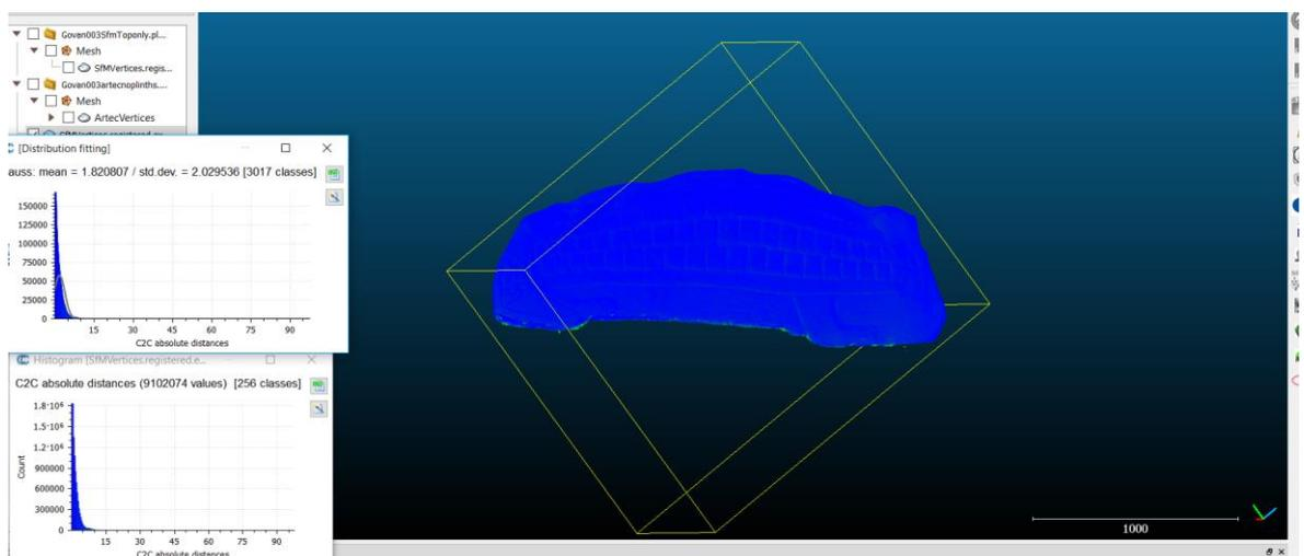
**Figure 5.1.** Photogrammetric and WLS 3D models of Govan 3 compared through *CloudCompare*. The main deviations occur near the edge of the 3D model (2-3 mm difference between points), largely because photogrammetry was able to capture more of the stone than WLS.
