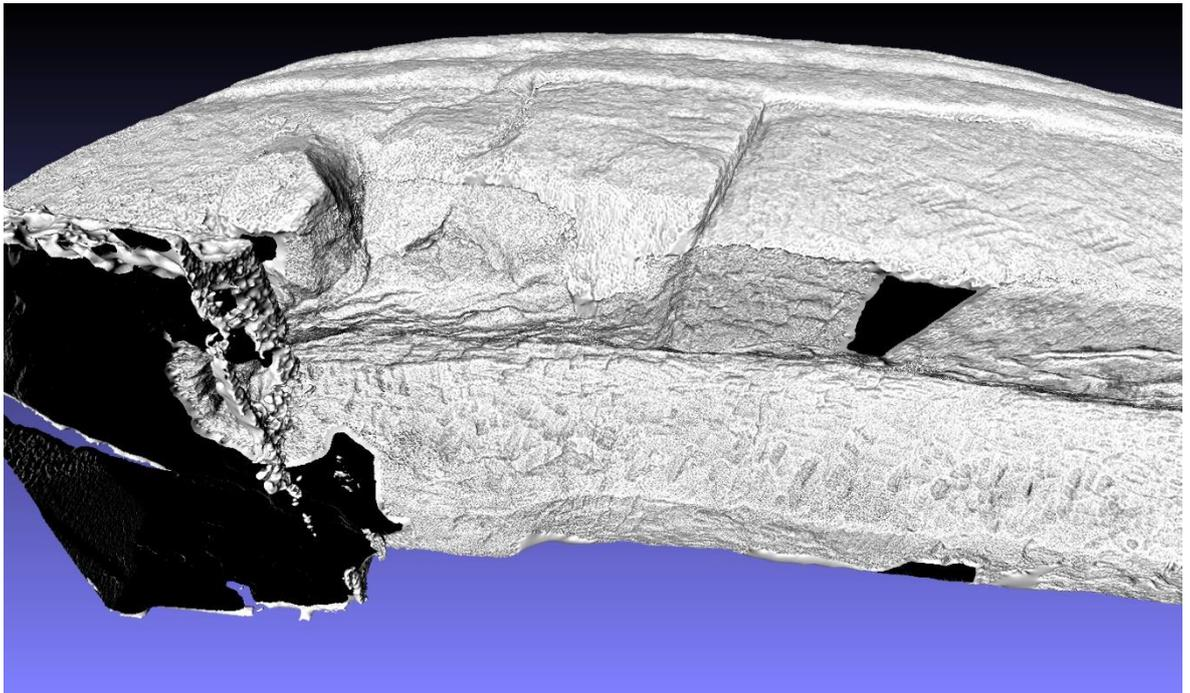
Figure 5.4. The underside of the model of Govan 3, where areas of low data capture (the plinth in the left portion of the image) and holes which have been filled (smooth areas along the edge of the stone) can be identified.
