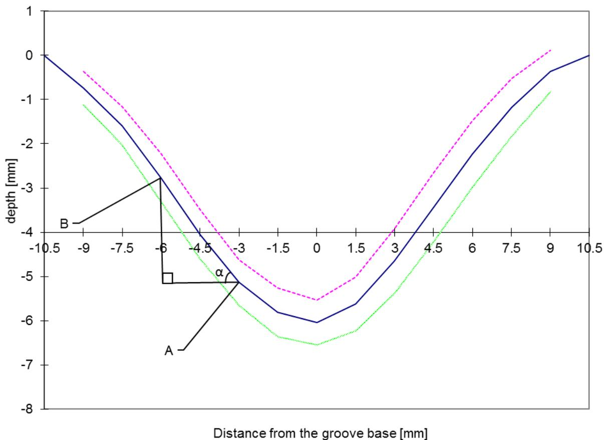
Figure 5.13. Diagram of Govan 14 sample 8 Groove Profile, demonstrating how Groove Angle variable  $\alpha$  is calculated.
