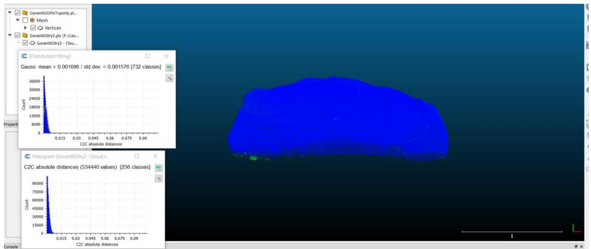
**Figure 5.3.** Laser scan point cloud of Govan 3 compared to the SfM photogrammetric point cloud. Again, a 2-3 mm average distance was found between corresponding points, with most of the inaccuracy relating to the bottom edge of the monument.
