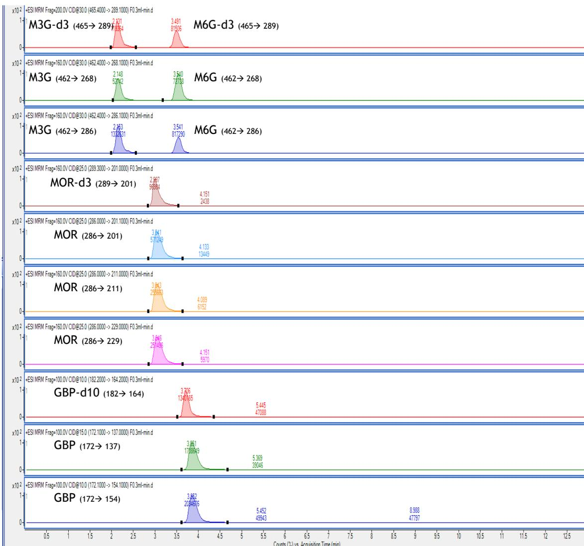
Figure 4-22 The Chromatogram of 4 drugs and 4 Internal Standards
