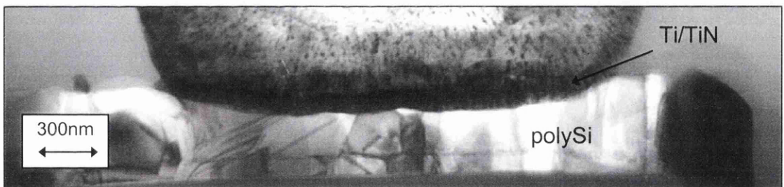
Figure 3.12: Image showing the thickness variation of the Ti/ TiN diffusion barrier
