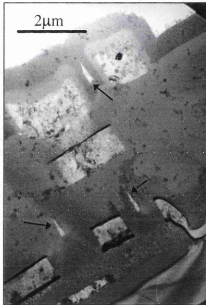
Figure 3.19: Voids in the \text{SiO}_2 (marked with arrows) created during fabrication are probably harmless, but could provide sites for unwanted impurities
