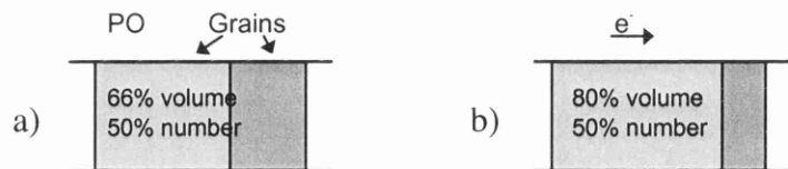
Figure 5.21: Diagram showing that the number fraction of grains, not the volume fraction, affects the electronic properties. Both films have the same number of grain boundaries, and only the number fraction of a PO reflects this
