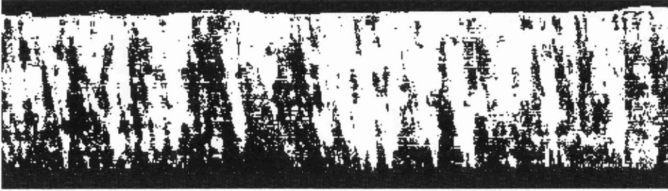
Figure 6.24: The binary image of figure 6.23 used to allow simple calculations to determine the degree of texture through the film
