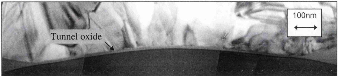
Figure 3.16: Image showing the thickness uniformity of a 15nm layer of \text{SiO}_2 , 'tunnel oxide'
