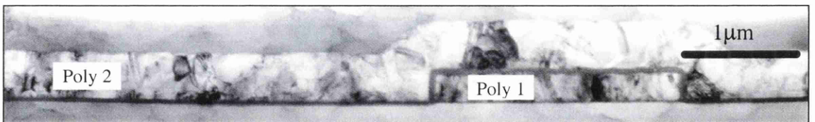
Figure 5.1: Image of the two polySi films studied for POs using the Kikuchi method
