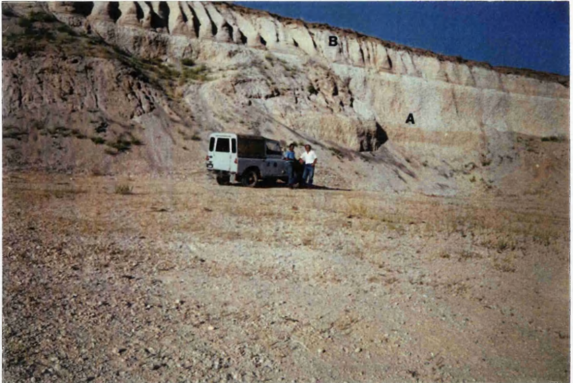
Photo 3.13. Pumice deposits on the Ercis-Patnos road side (38025-33250), view towards NE. The deposits are poorly graded and show local changes in both thickness and depositional features. The lower part (A) is composed of a coarse pumice, and the upper part (B) comprises fine pumice clasts.
