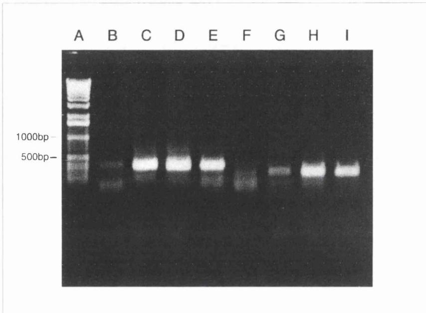
**Figure 3.2.2.4 Optimisation of Annealing Temperature**
