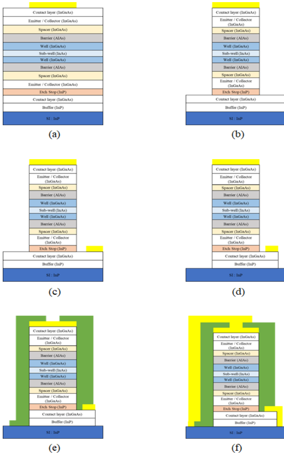
Figure 2.2: RTD device fabrication steps: (a) top contact metal deposition, (b) wet etch to the bottom emitter/collector layer, (c) bottom contact metal deposition, (d) wet etch to substrate, (e) PI-2545 deposition and via opening using dry etch, (f) bond pad metal deposition
