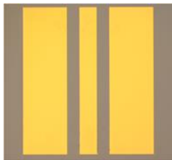
Figure 3.5: Micrograph of CPW test structure. The centre strip width is 60 \mu\text{m} , the gap width is 40 \mu\text{m} , while the ground plane width is 200 \mu\text{m} . The CPW test structure length is 500 \mu\text{m} .
