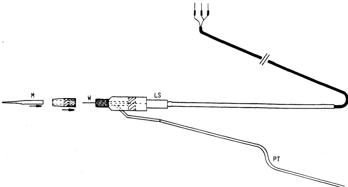
Fig. 5: Suction electrode for extracellular measurement of nerve AP conduction. A silver wire (W) was connected electrically via a Limb socket (LS), embedded in perspex, to the recording circuitry (Fig. 7). A glass microelectrode (M) was placed over the silver wire and connected via polythene tubing (PT), filled with liquid paraffin, to the remainder of the apparatus (Fig. 6).
