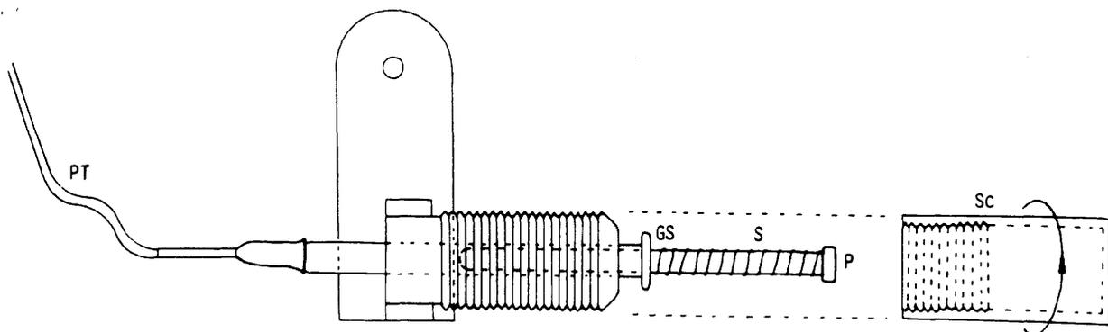
**Fig. 6:** Suction electrode for extracellular measurement of nerve AP conduction. Changes in pressure at the microelectrode tip (Fig. 5) were induced by movement of the plunger (P) of a glass syringe (GS), in either direction, by means of a perspex screw (Sc) and a steel spring (S) placed around the plunger. The syringe, filled with liquid paraffin, was connected to the remainder of the suction electrode (Fig. 5) by polythene tubing (PT).
