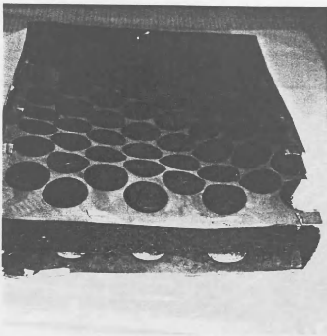
Last remaining air filter unit, as found, except for partial cleaning of plate. Dimensions are 500x375x50mm
