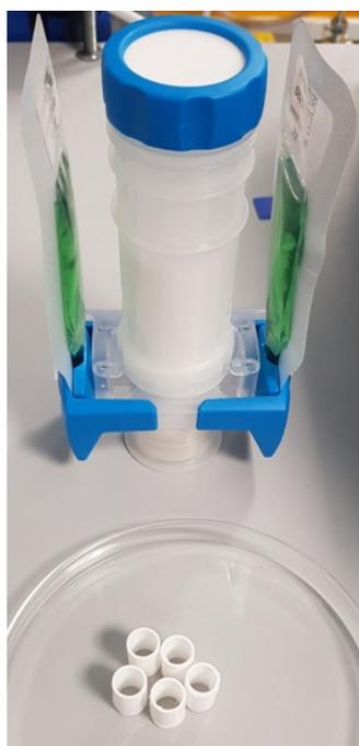
*Figure 53 – Optipac® bone cement mixing device and plastic moulds. Monomer (green) is added to the white polymer powder within the canister under vacuum then manually mixed.*
