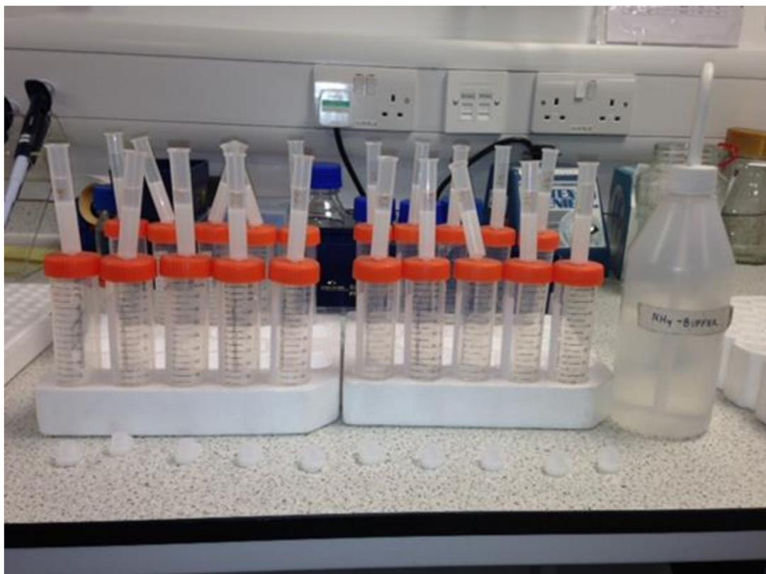
**Figure 2-3. Desalination using PD-10 column.**
