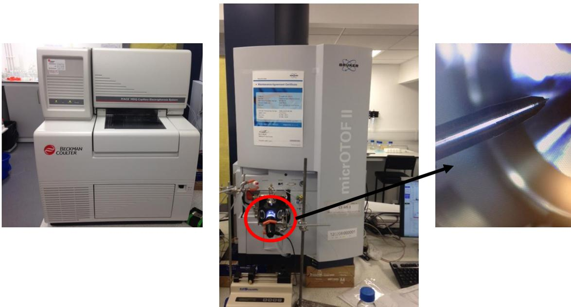
**Figure 2-4. Capillary electrophoresis – mass spectrometry.**
