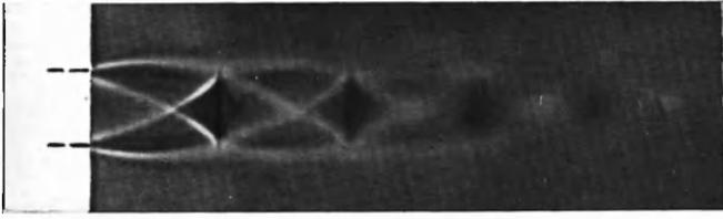
Fig. 2. — Shadow Photograph of Jet from a nozzle under expanding from 50lb/in<sup>2</sup> gauge to atmosphere.
