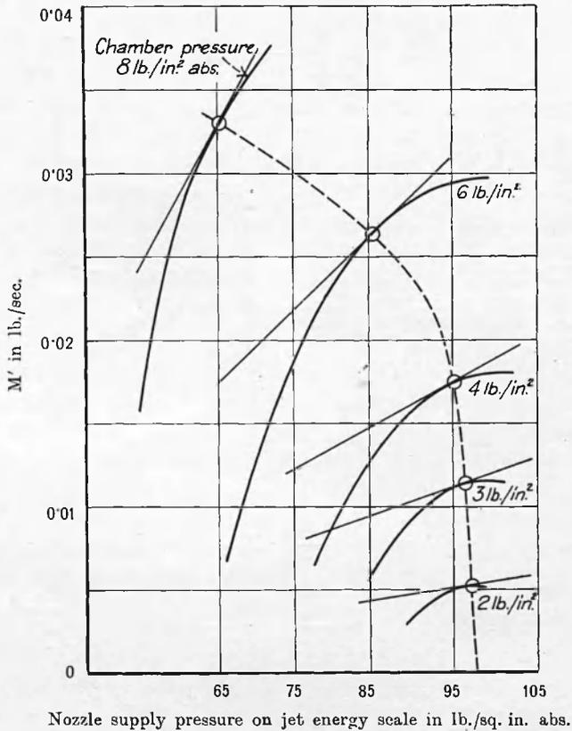
FIG. 3.—Curve of Maximum Efficiency, Diffuser "B."
