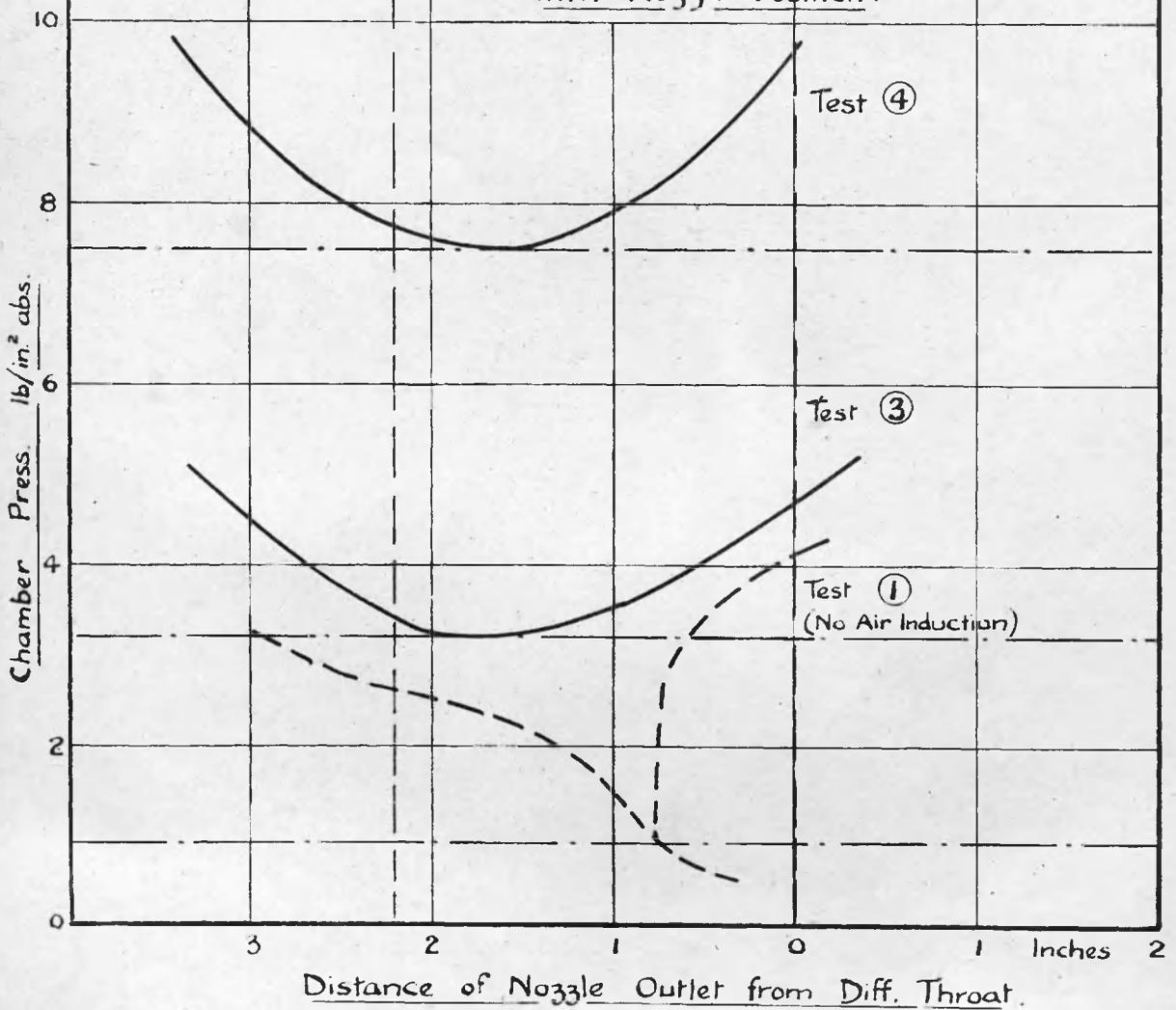
chamber, which allows the ejector to adjust itself to its own vacuum almost immediately.
