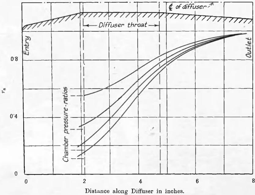
FIG. 5.—Pressure Ratio Curves, Diffuser "B."
