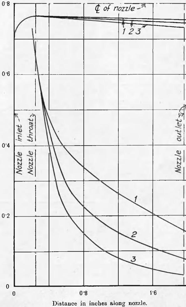
FIG. 4.—Pressure Ratio Curves, Nozzles 1, 2, and 3.
