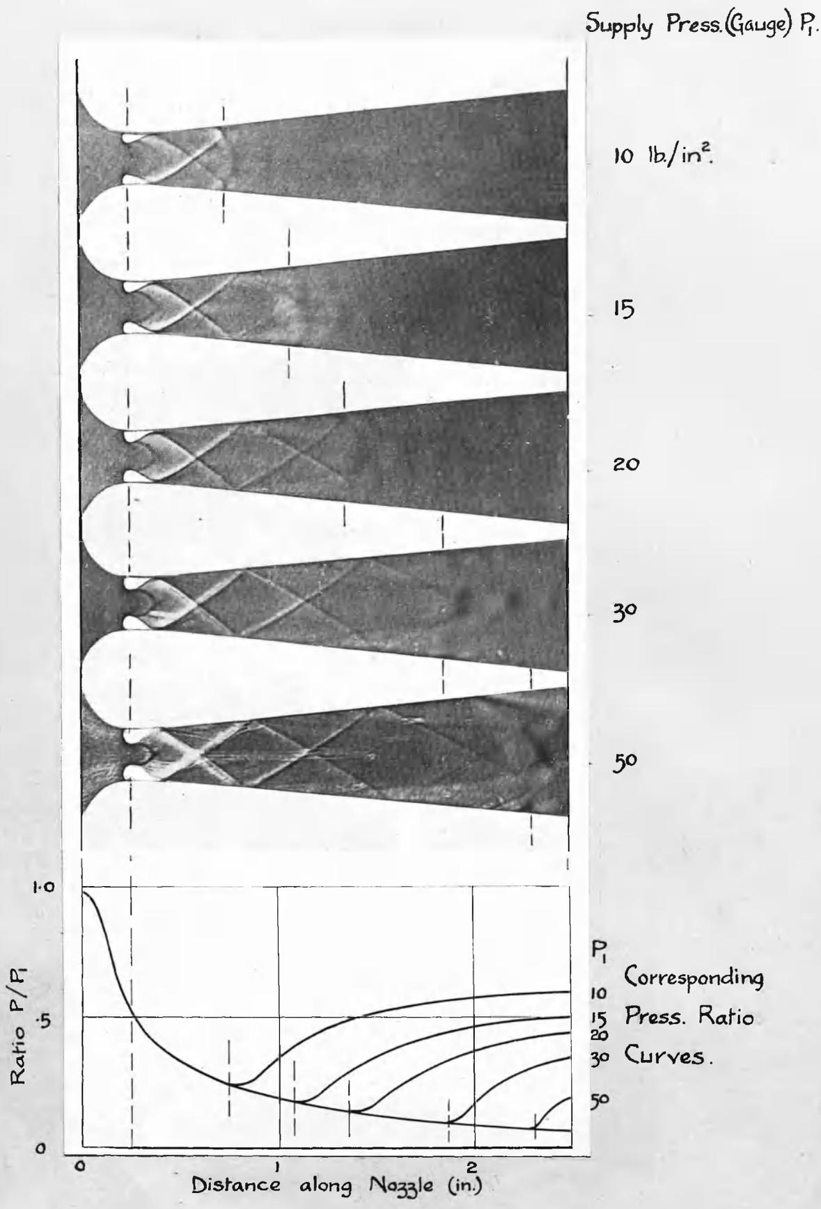
Fig. 4. - Shadow Photographs of waves produced in a glass-sided divergent nozzle by projections, 0.02 in. high, fixed at the throat.
