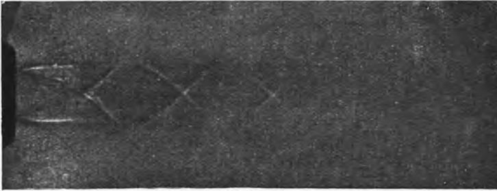
(a) Expansion to atmosphere (sides of diffuser removed). Nozzle press. 95 lb. per sq. in. abs.
