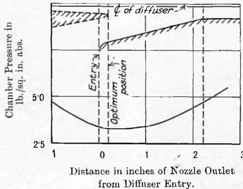
FIG. 6.—Effect of Distance between Nozzle and Diffuser.
