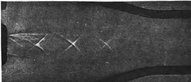
(b) Nozzle press. 65 lb. per sq. in. abs.; suction 0.046 lb. per sec.; chamber press. 10.0 lb. per sq. in. abs.
