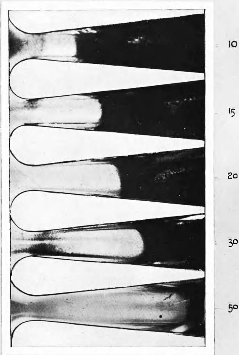
Fig. 1 - Air Jet Photographs, showing the effect of the jet on the oil-coated glass sides of a divergent nozzle.
