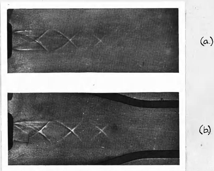
(a) Expansion to atmosphere (with brass strips of diffuser removed). Nozzle pressure  $95 \text{ lb./in.}^2 \text{ abs.}$
