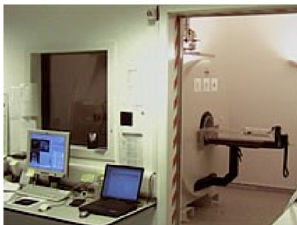
Figure 4.4: Bruker Biospec 7 Tesla MRI scanner with a 30 cm horizontal bore and the equipment used for preclinical experiment in GEMRIC.
