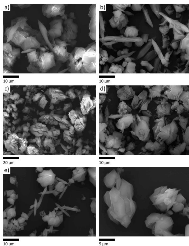
Figure 2.24. SEM images of 1-TFA prepared with different molar equivalents of TFA: a) 1 eq, b) 2 eq, c) 3 eq, d) 4 eq, e) 5 eq.
