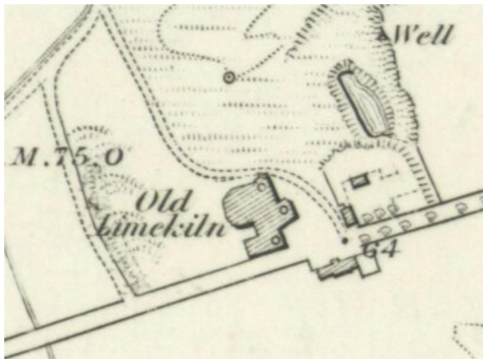
Figure 22 Roofed building symbol with three obvious draw holes. No trace remains of what appears to have been a substantial bank of draw kilns. Forfarshire Sheet 28, published 1865.
