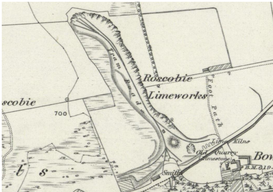
Figure 48 Roscobie Limeworks in Fife (Six-inch first edition, Fife sheet 30, published 1856). Note the use of 'Tram Roads' leading from the quarry face to a bank of three clamp kilns.
