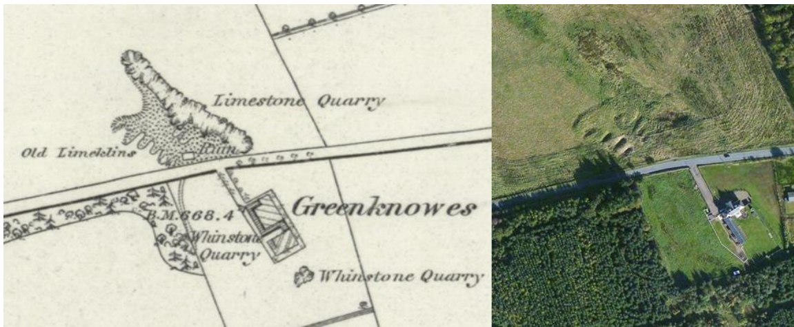
Figure 20 Disused lime kilns at Greenknowes in Fife (NT109932, Perth and Kinross, Sheet 30). Left: six clamp kiln symbols on the map (two are obscured by the quarry shading). Right: the same view from Bing aerial photography showing clear clamp kiln shaped depressions on the ground. Note that the more degraded kiln on the left is faithfully represented, whereas the relative size of the other clamps appears quite different between the photograph and the map.
