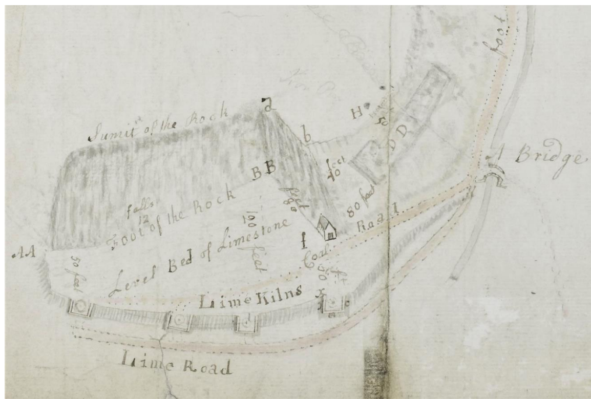
Figure 39 Plan of the limestone quarry of Craighead, in Dailly, Ayrshire, 1797 (NRS RHP1628). Limestone was carried a short distance from the quarry face to be loaded in the head of the four draw kilns. Coal was led up to the working platform along a short road. The burned lime was then drawn out level with the lime road and carted off for sale.
