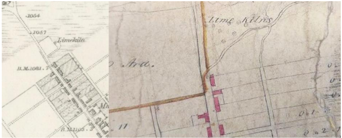
Figure 25 Comparison between estate map and OS First Edition. Right: Group of eight lime kilns at the north end of the village of Tomintoul in Moray, from a plan of Strathavon, surveyed by George McWilliam, 1839 (NRS, RHP1807). The same plan shows a further four kilns immediately to the south of the village. Left: The corresponding OS sheet, Banffshire Sheet XL, surveyed 1869 and published 1872, shows only a single kiln symbol at each end of the village.
