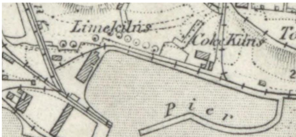
Figure 19 Map symbols for Charlestown Harbour in Fife (NT064835, Fife and Kinross-shire, Sheet 39, published 1856). Charlestown lime works was at one time the largest producer of lime in Scotland. Note the sequence of symbols set against the line depicting the edge of the kiln bank, with each symbol representing one of the nine pots on the site. The variations in symbol here do not correspond to any known difference in kiln pot design, hence the opinion that the circle-dot symbol (and its variants) represents some kiln of generic lime kiln.
