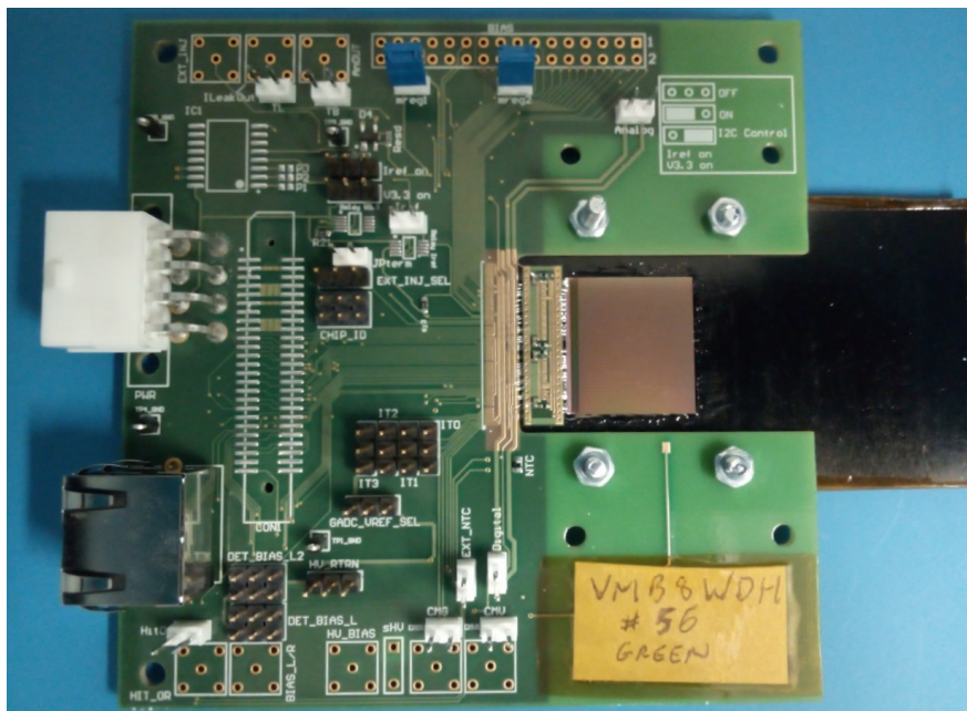
Figure 5.3: Single Chip Card (SCC) with ASIC-Sensor assembly mounted on a Carbon Fiber Reinforced Polymer (CFRP) base board.
