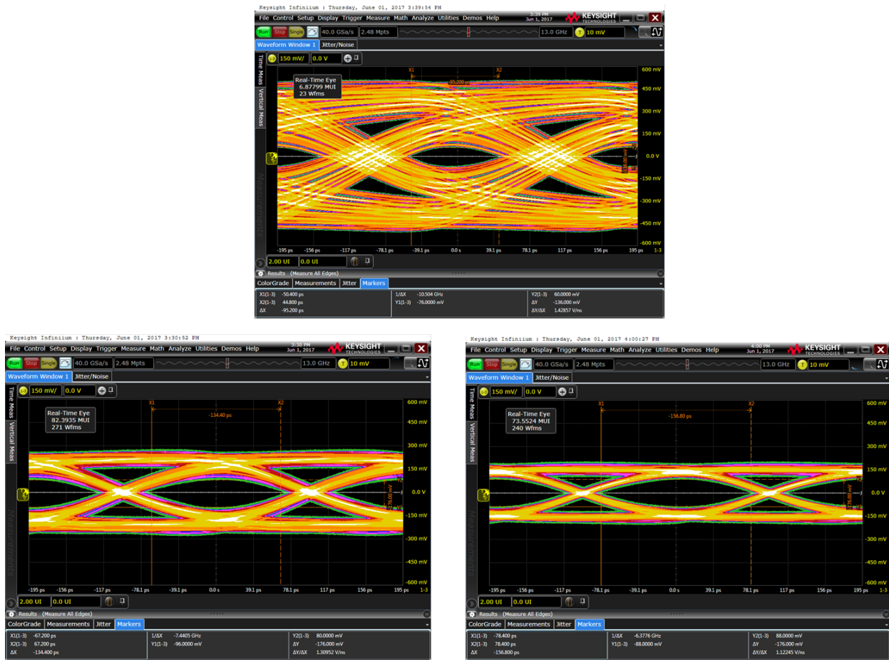
Figure 4.15: Top - Eye diagram with no CTLE applied. Bottom left - Eye diagram with CTLE circuit without L-R-L network and Bottom right - CTLE circuit with L-R-L network.
