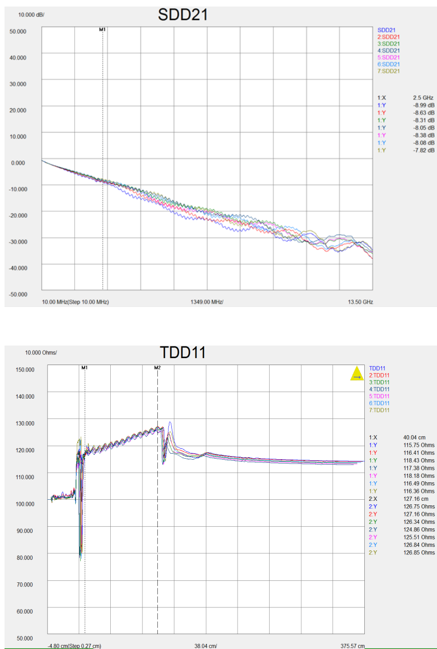
Figure 4.3: Top - Transmission results (S-parameters) for TapeVar1.1 measuring a mean loss of 8.32 dB at 2.5 GHz. The results are without fixture removal. Bottom - Impedance measured to be 120 \Omega on (pseudo) TDR on the network analyser.
