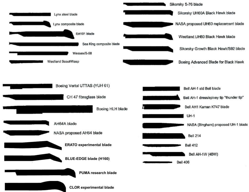
Figure 1.12: A wide range helicopter rotor blade planforms showing the variety of used designs based on [178].
