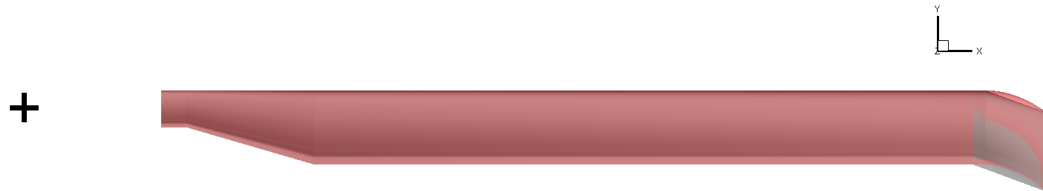
Figure 9.1: Difference between the baseline (in grey) and parameterised (in red) AH-64A blades
